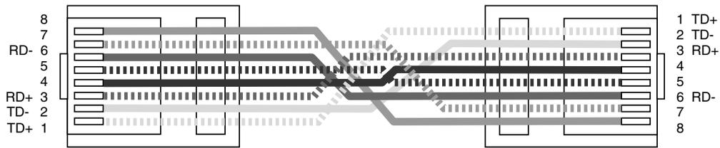
Figure 2-6: 10/100Base-T Straight-through cable
