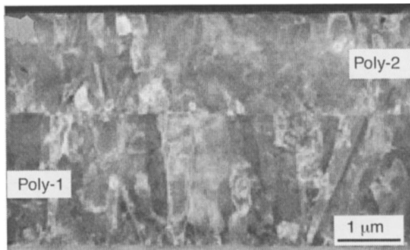
Fig. 3.18. TEM micrograph of cross section of polysilicon films.
