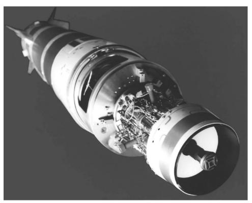
**Figure 3.1** Raytheon's Lightweight Exoatmospheric Projectile (LEAP) is a highly modular, lightweight, space-tested interceptor element for the Standard Missile-3. Courtesy Raytheon (*see colour section*).
