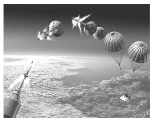
Figure 7.3 Launch abort system. Courtesy NASA.
