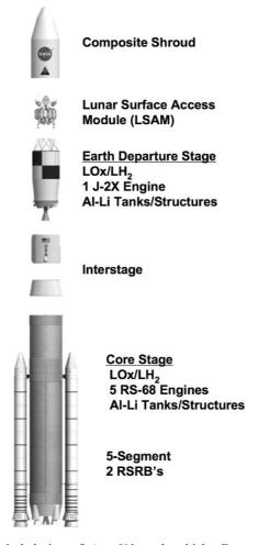
Figure 7.2 Exploded view of Ares V launch vehicle. Courtesy NASA.
