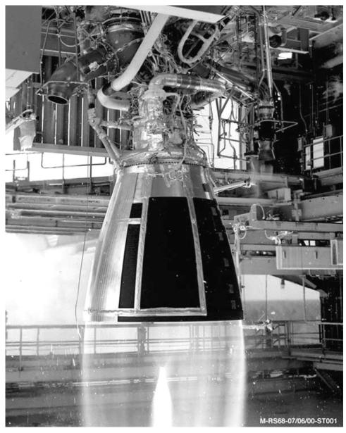
Figure 7.4 RS-68 rocket engine. Courtesy NASA.
