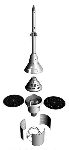
Figure 7.6 Exploded view of Orion. Courtesy NASA.
