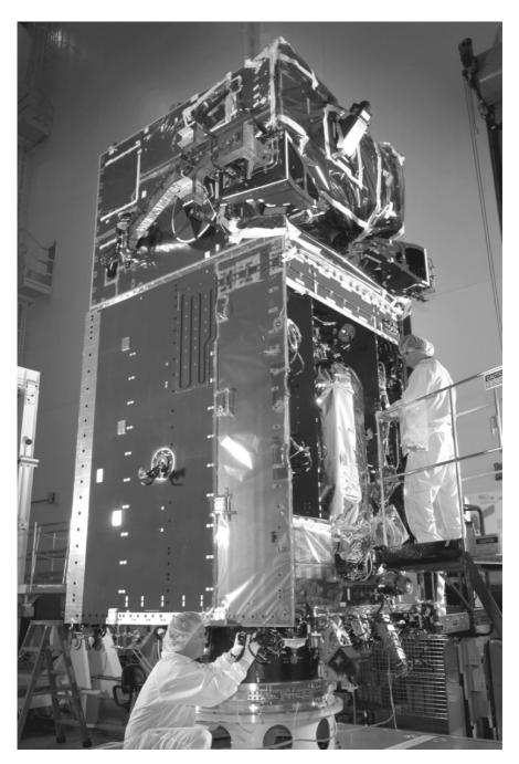
**Figure 4.10** Lockheed Martin technicians prepare the first Space-Based Infrared System (SBIRS) geosynchronous orbit (GEO-1) spacecraft for a major test at the company's facilities in Sunnyvale, California. Courtesy Lockheed Martin.
