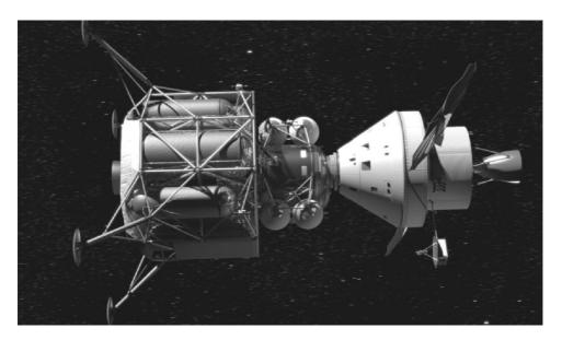
Figure 7.5 Altair attached to the Orion capsule. Courtesy NASA (see colour section).
