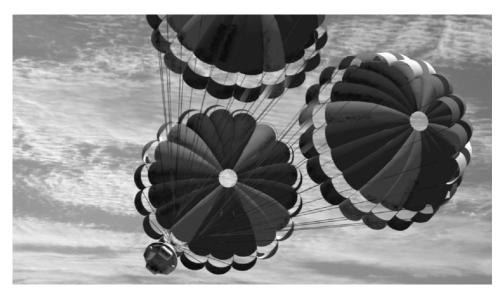
Figure 7.8 Orion's primary parachutes. Courtesy NASA.
