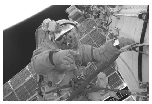
Figure 7.12 Orlan space suit. Courtesy NASA (see colour section).
