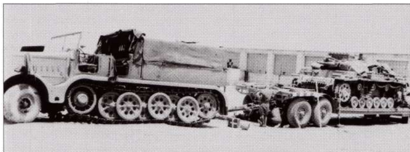
A damaged late-production PzKpfw III Ausf F armed with the 50mm KwK 38 L/42 being loaded onto a heavy tank transport trailer towed by a heavy 18-ton tractor FAMO F2 SdKfz 9. Regimental workshops ( Panzer Werkstatt Kompanien ) did an excellent job in recovering and repairing damaged tanks. (Filippo Cappellano)
