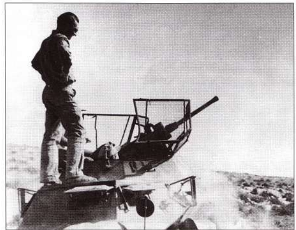
A leichte Panzerspähwagen (2cm) SdKfz 222 in an apparently staged photo to show its 20mm Kwk 30/38 used in an anti-aircraft role. Poorly armoured and excessively lightweight, the SdKfz 222 did not prove a suitable vehicle for desert warfare. (Carlo Pecchi Collection)
