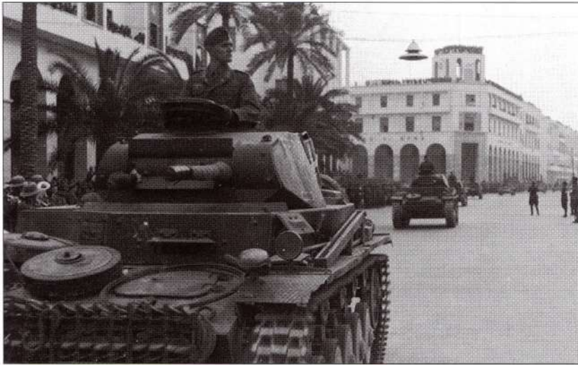
A column of PzKpfw II Ausf. Cs of Panzer Regiment 5, very likely belonging to one of II.Abteilung's leichte Panzerzug . The 1941 establishment of a Panzer regiment still included a large number of these light tanks. (Carlo Pecchi Collection)
