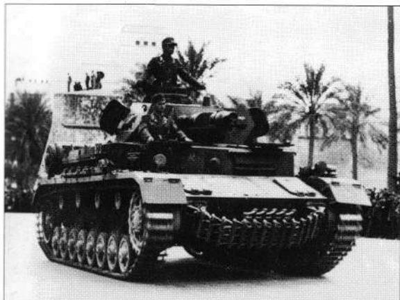
A PzKpfw IV Ausf. D of 8. Kompanie/Panzer Regiment 5 parading through the streets of Tripoli. Though it was the heaviest tank in the DAK inventory until November 1942, its 75mm KwK 37 L/24 was of little use against enemy armour except at very short ranges. (Carlo Pecchi Collection)
