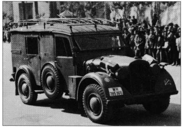
An Auto Union/Horch Kfz 17 communications car belonging to the Nachrichten Zug of Panzer Aufklärungs Abteilung 3 (see tactical sign on the left mudguard) parades through the streets of Tripoli. This vehicle was used by Nachrichten Züge in a wide variety of different arrangements, either for radio or wire communications. (Carlo Pecchi Collection)
