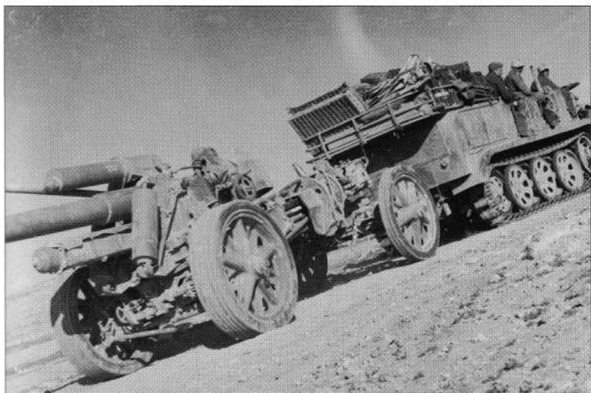
A 150mm schwere Feldhaubitze 18 howitzer towed by an 8-ton Krauss-Maffei KM m 11 SdKfz 7 tractor (note the three external wheels). It belonged to III.Abteilung of either Artillerie Regiment 155 or 33. (Carlo Pecchi Collection)
