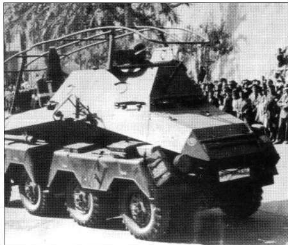
An eight-wheeled Panzerfunkwagen SdKfz 263, a heavy communications armoured car mounting a 30-watt Funkgerät 8 with a large frame antenna. It probably belonged to 3.Kompanie/Nachrichten Abteilung 39 (mot). (Filippo Cappellano)
