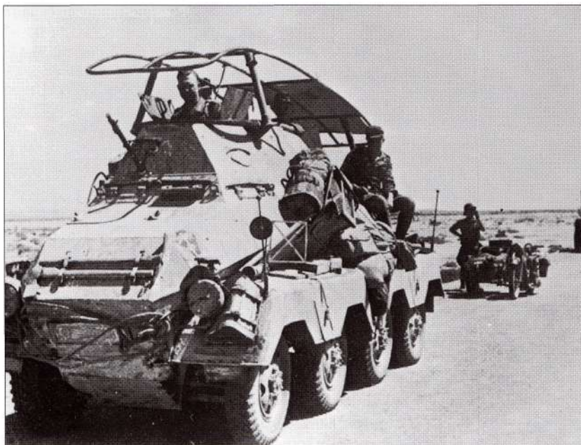
A column belonging to a Panzer division's Nachrichten Abteilung , very likely portrayed in spring or summer 1941. The first vehicle is an eight-wheeled Panzerfunkwagen SdKfz 263 followed by a BMW combination and by two kleiner Panzerfunkwagen SdKfz 260/261. The DAK's 'palm with swastika' insignia stands out on the dark-grey background. (Carlo Pecchi Collection)
