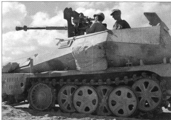
An SdKfz 250/1 armed with a French 25mm Hotchkiss light anti-tank gun. In early May 1942 Panzer Aufklärungs Abteilung 33 received ten of these, which were used to form two Züge (each one with five vehicles) in its schwere Kompanie . (Carlo Pecchi Collection)
