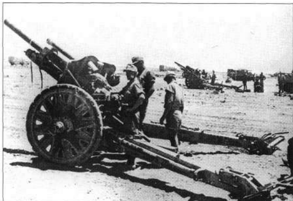
A leichte Batterie equipped with 105mm leichte Feldhaubitze 18 howitzers is ready to open fire (note the 3-ton Hanomag H Kl 6 SdKfz 11 half-tracks in the background). This howitzer was inferior to its British equivalent, the 25-pdr. (Carlo Pecchi Collection)
