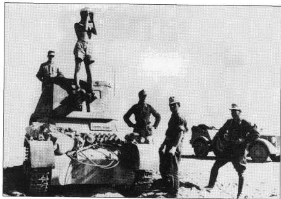
In a featureless terrain like the Western Desert, even standing on top of a tank was helpful for observation. A 47mm Pak (t) L/43 (sfl) auf PzKpfw I Ausf. B (or simply Panzerjäger I) in the desert. These equipped Panzerjäger Abteilung 605 (sfl), and were still in use in October 1942. (Carlo Pecchi Collection)
