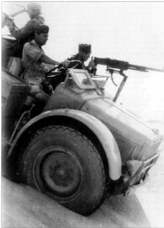
Vehicles derived from the TL37 artillery tractor, like this armed version, had good off-road mobility and were heavily armed. (Filippo Cappellano – AUSSME)
