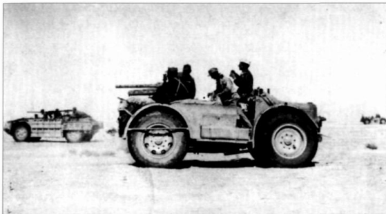
An AS37, modified with a 75mm gun, and an AS42 Sahariana to the rear. The AS37 and AS42 proved very effective vehicles, with good firepower and mobility, and they gave the Italian forces the ability to respond quickly. (Filippo Cappellano – AUSSME)
