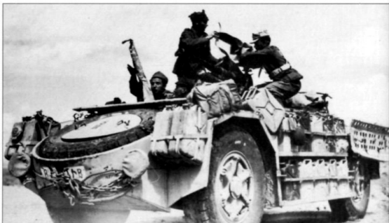
The most powerful version of the AS42 Sahariana was armed with a 47/32 gun and two 8mm machine guns. The 47/32 gun had AT and fire-support capabilities. (Filippo Cappellano – AUSSME)
