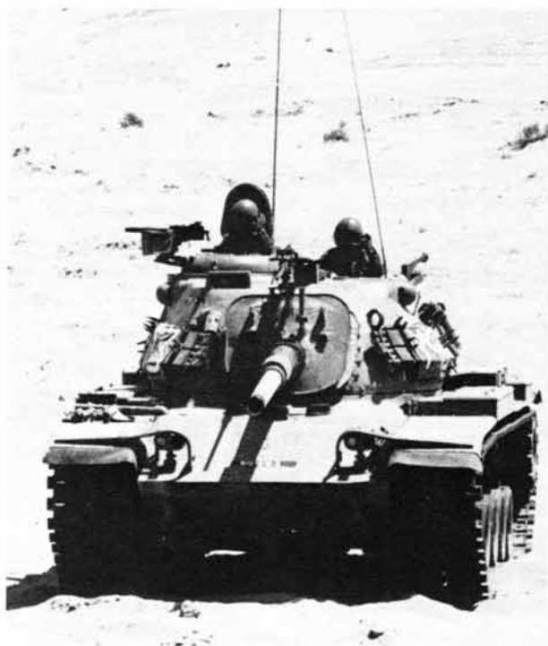
M60A1 tank in Sinai, 1973. Generally satisfactory, it suffered from one vulnerability which had to be remedied urgently after the October War. The fast turret traverse system tended, if hit, to spray hydraulic fluid with a low flashpoint into the tank, causing explosive internal fires. (Author's collection)
