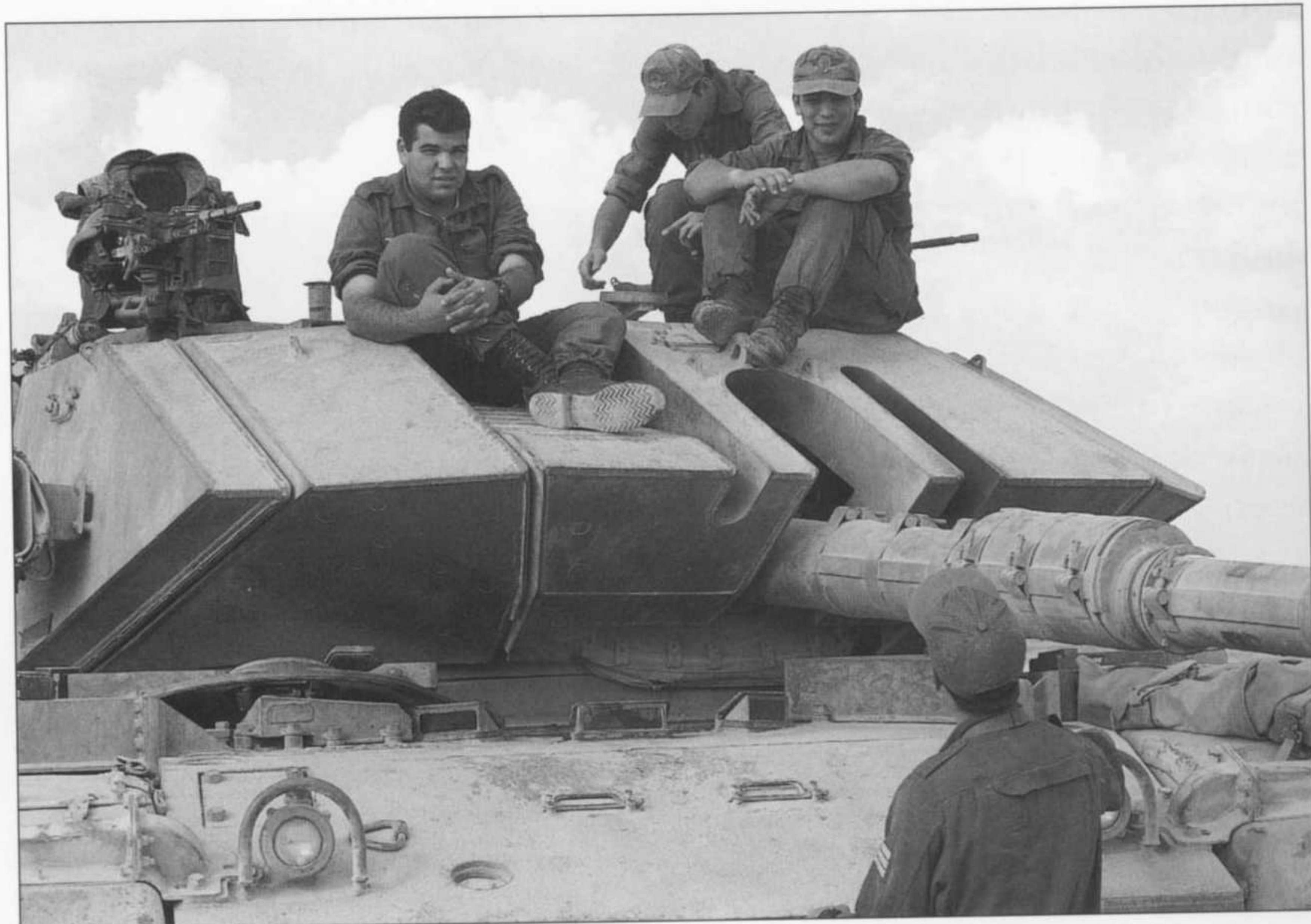
A Magach 7C photographed during 2000 in the Negev desert. The heavy, appliqué passive armour modules give the tank its characteristic arrowheaded front profile. The crew wear non-issue baseball caps with an unofficial unit logo of a tank and dragon.
