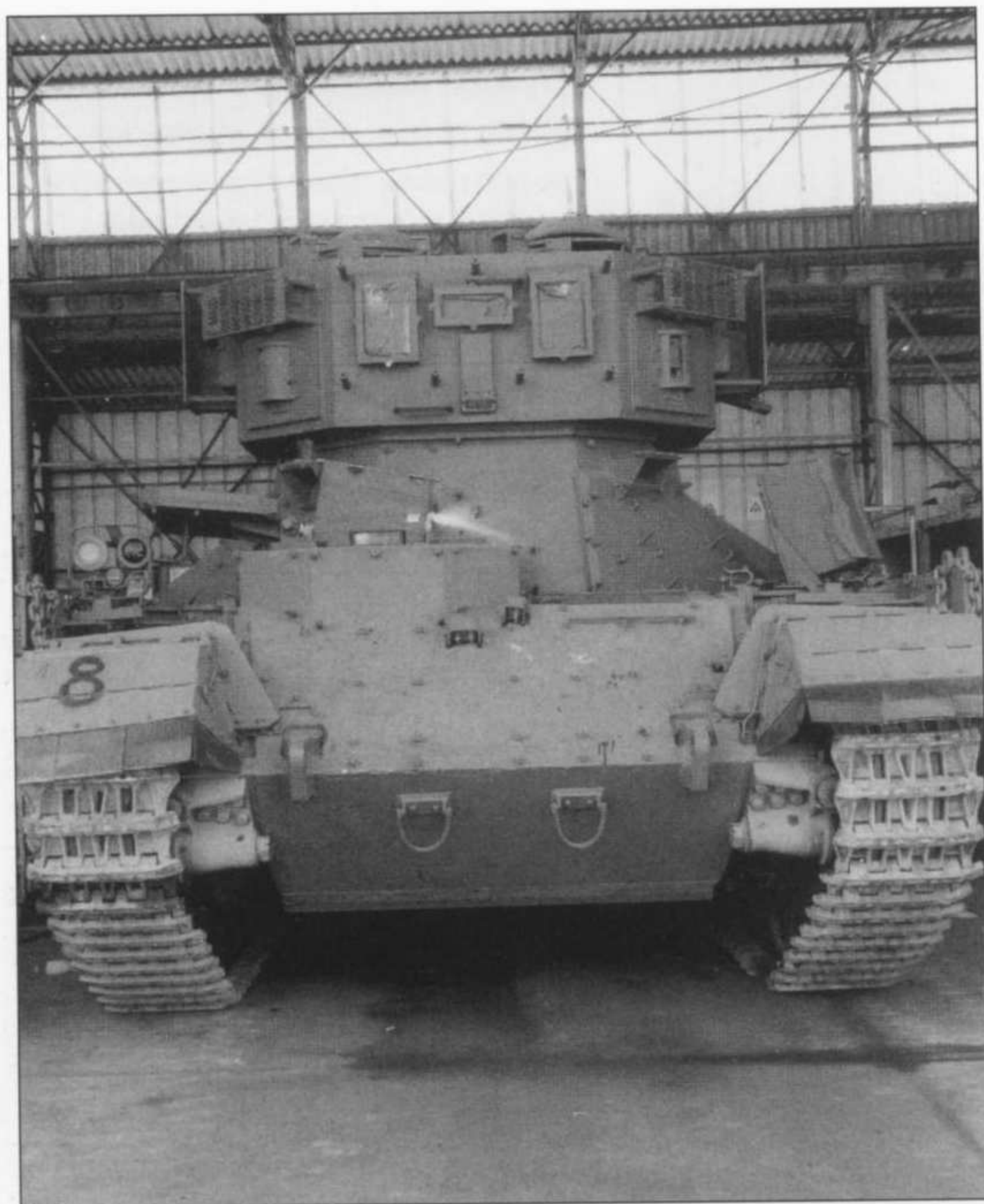
A Mifletset, or 'monster', photographed in December 2002 at Tel ha Shomer. The Mifletset is a conversion of the Nagmachon optimised for low-intensity conflicts in urban environments. Crude and ugly, but effective, this Mifletset awaits the fitting of its ERA tiles.
