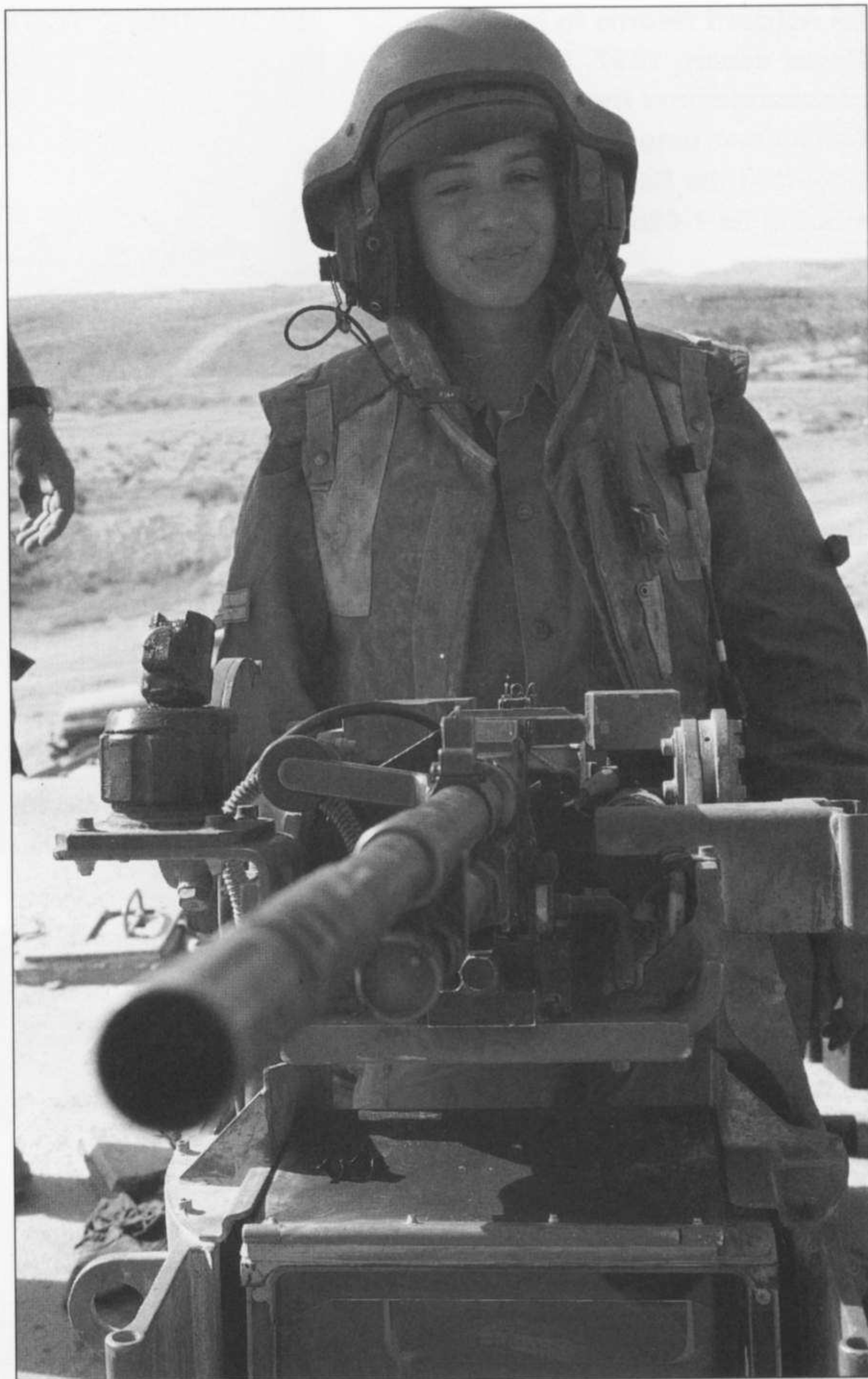
A female instructor waits by a Rafael OWS. Note the instructor's flak jacket and Type 602 helmet. The optical sight for the OWS is visible below the gun barrel. The knurled wheel to the left of the weapon is a searchlight mount.
