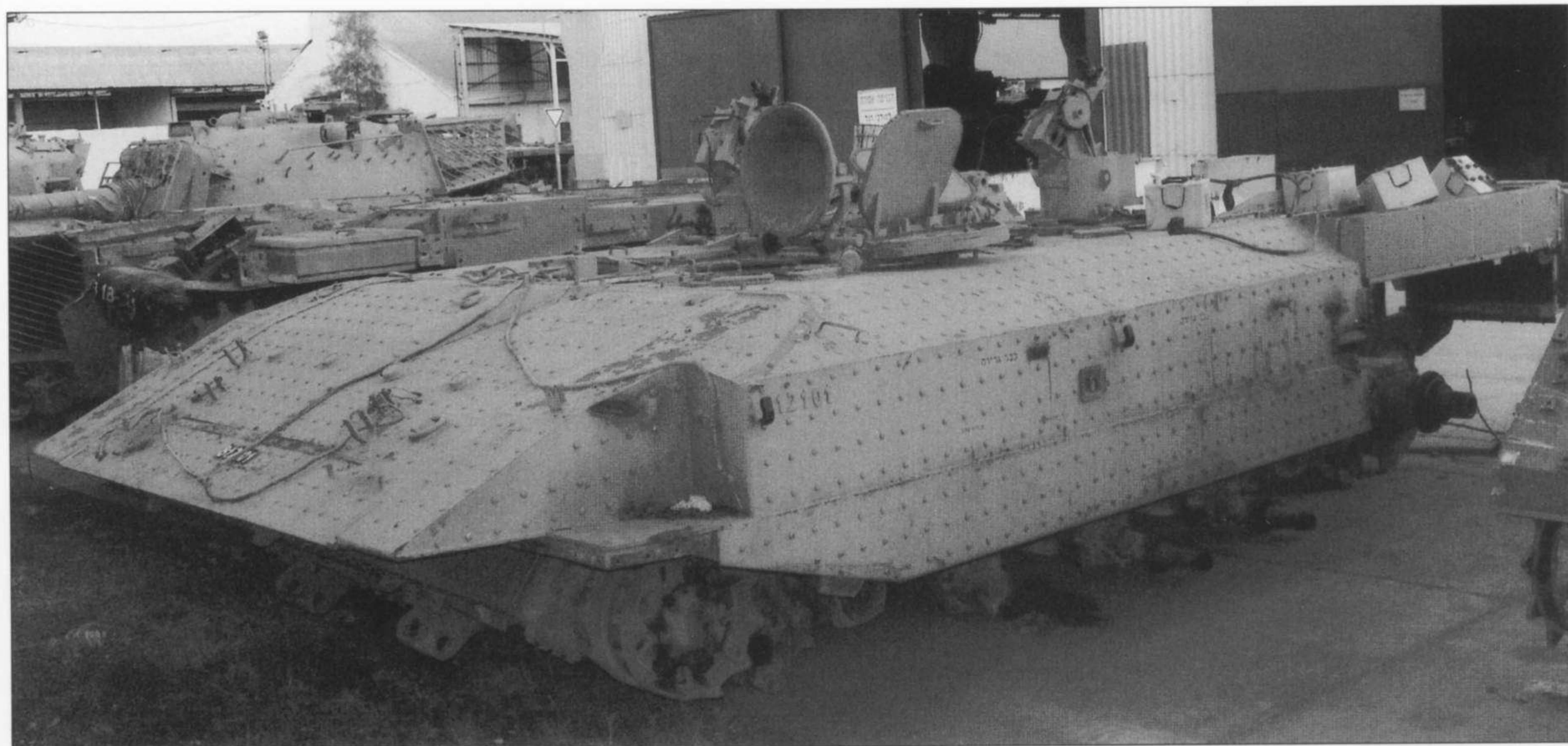
A tatty, pre-series-production Achzarit photographed in 2002 at Tel ha Shomer ordnance base. These early machines are distinguished by the heavily riveted armour found on their flanks and glacis, and by the fact that they carry two OWS.
