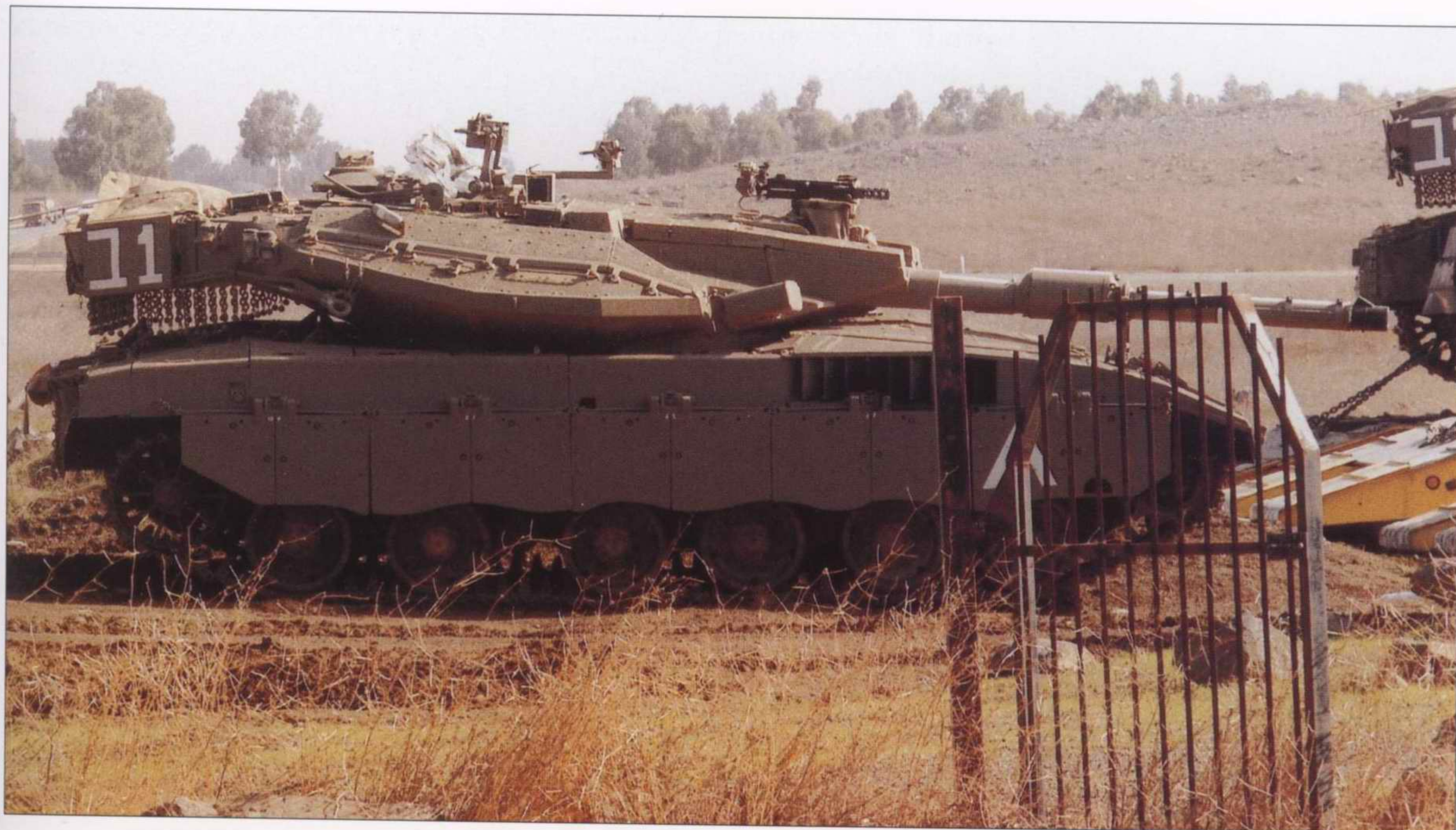
ABOVE A Merkava 3 Dor Dalet photographed near Nafach on the Golan Heights, December 2002. The fourth generation appliqué armour completely changes the turret profile. The machine gun, mounted over the cannon mantlet and used for sub-calibre training, is missing its barrel.
