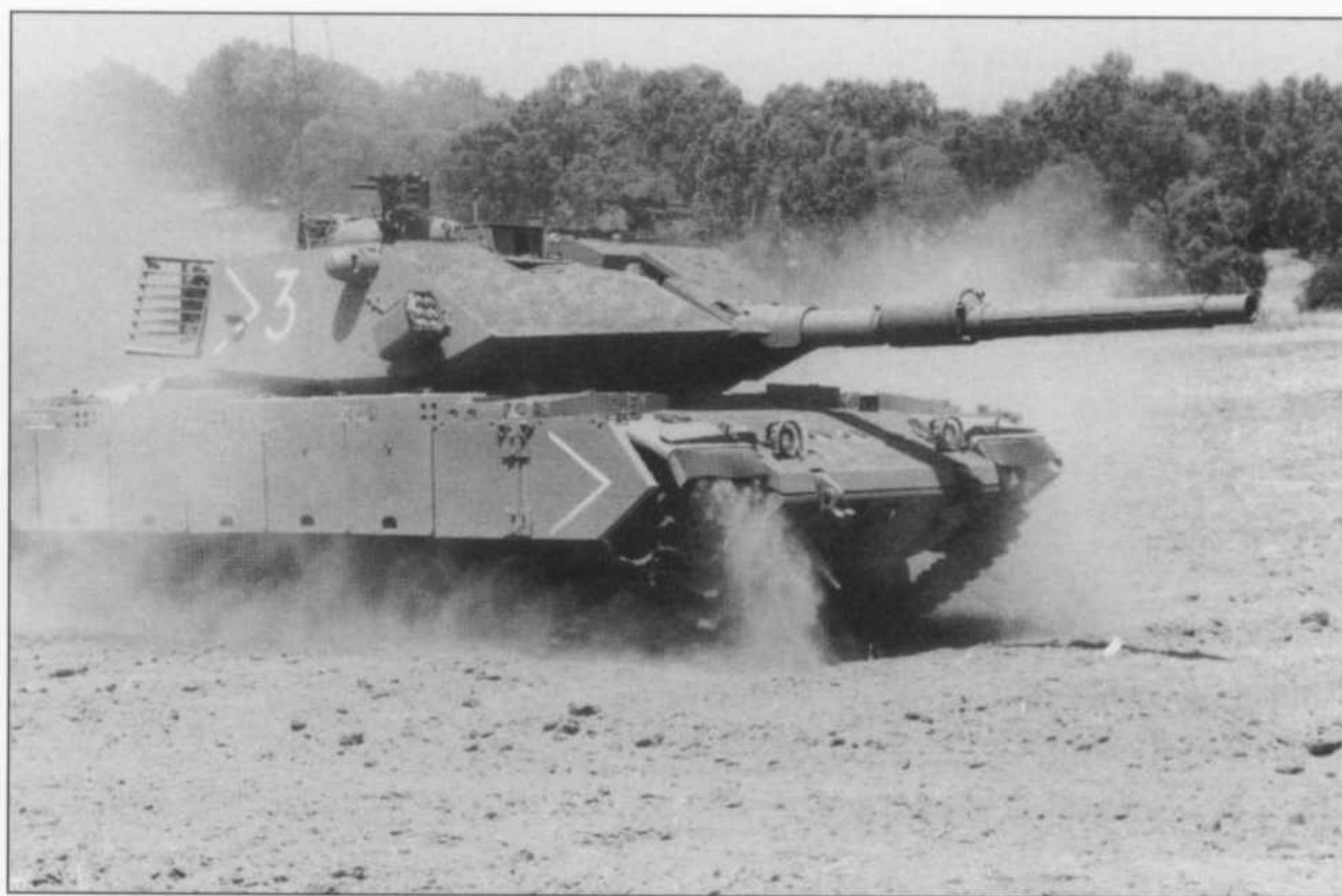
This is the Sabra, an export version of the Magach 7, photographed in 2000 whilst on trials. The Sabra is fitted with a 120mm cannon and has had some re-profiling performed on its arrowhead turret. Turkey is the lead customer for this tank. It is unlikely to enter IDF service. (IMI)
