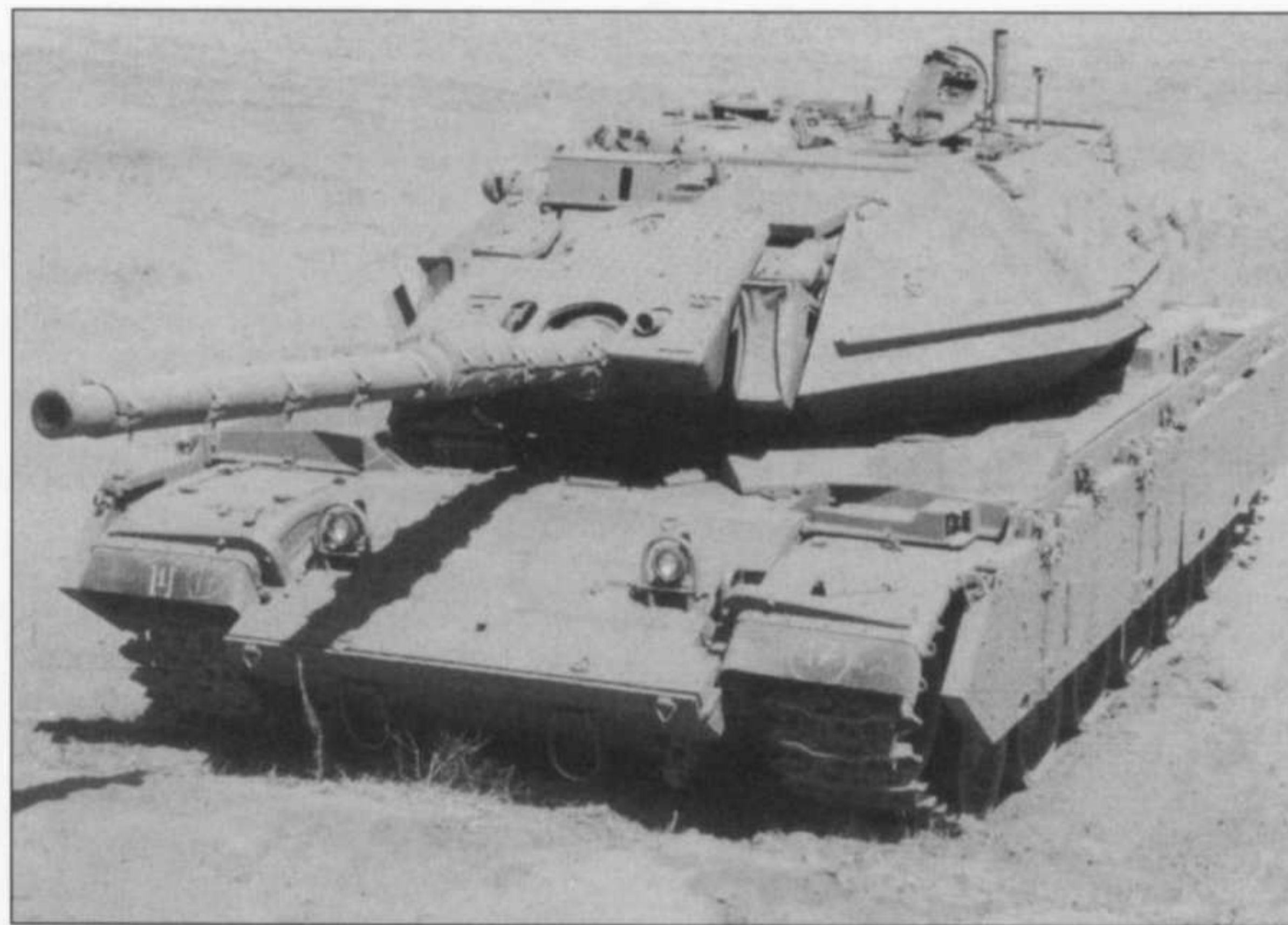
A Magach 6 BATASH showing off the curved turret lines formed by its add-on armour. The tank is sometimes seen in service without the heavy plate protecting the gun mantlet. (IMI/Slavin, courtesy Shaul Nagar)
