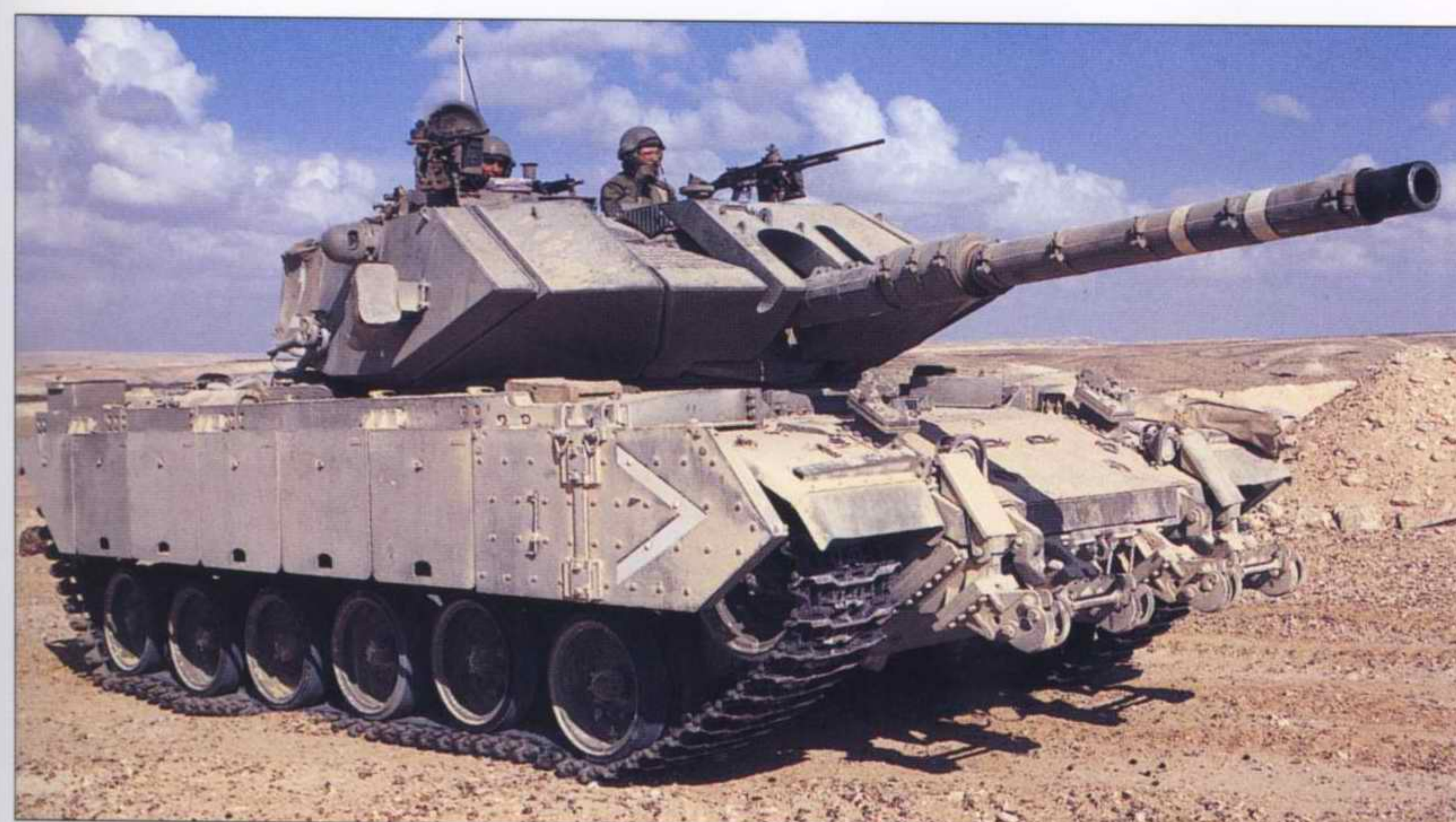
A Magach 7C photographed in the Negev desert, autumn 2000. Note the improved ballistic profiling when compared with the Magach 7A. This machine has been fitted with mounting brackets on its glacis for a bulldozer blade.
