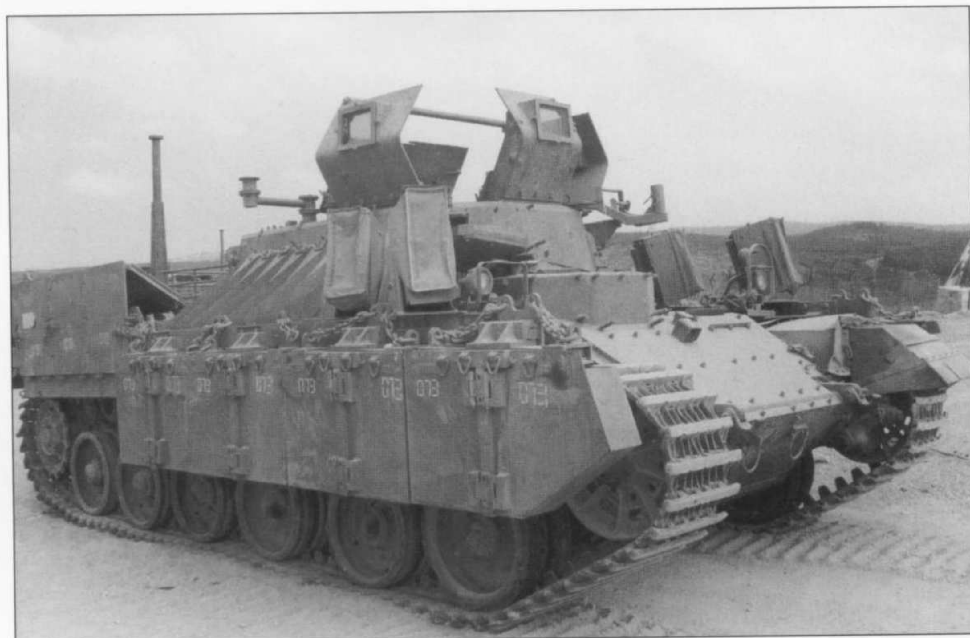
ABOVE TOP Nakpadon and Nagmachon Centurion-based carriers photographed in 2000. At the far left the chassis of a Nakpadon carrier with its appliqué armour modules removed can just be seen. The centre AFV is a Nakpadon, that on the right a Nagmachon.
