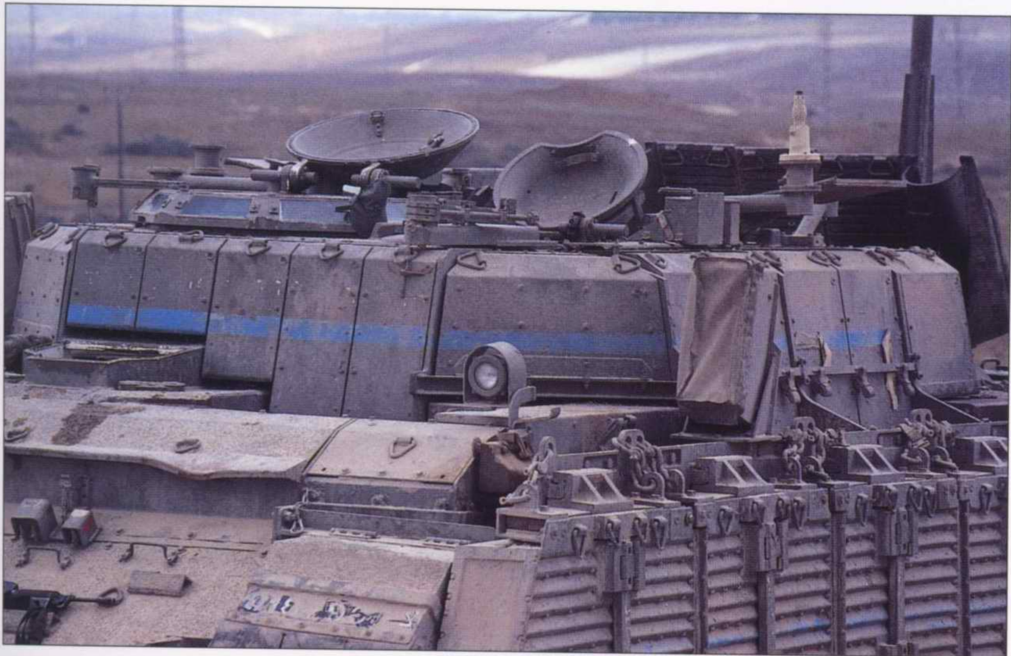
This photo taken in the summer of 2000 shows the thick appliqué armour modules carried by the Nakpadon. Note the vision blocks around the commander's cupola. The thin band painted on the fighting compartment is sky blue.
