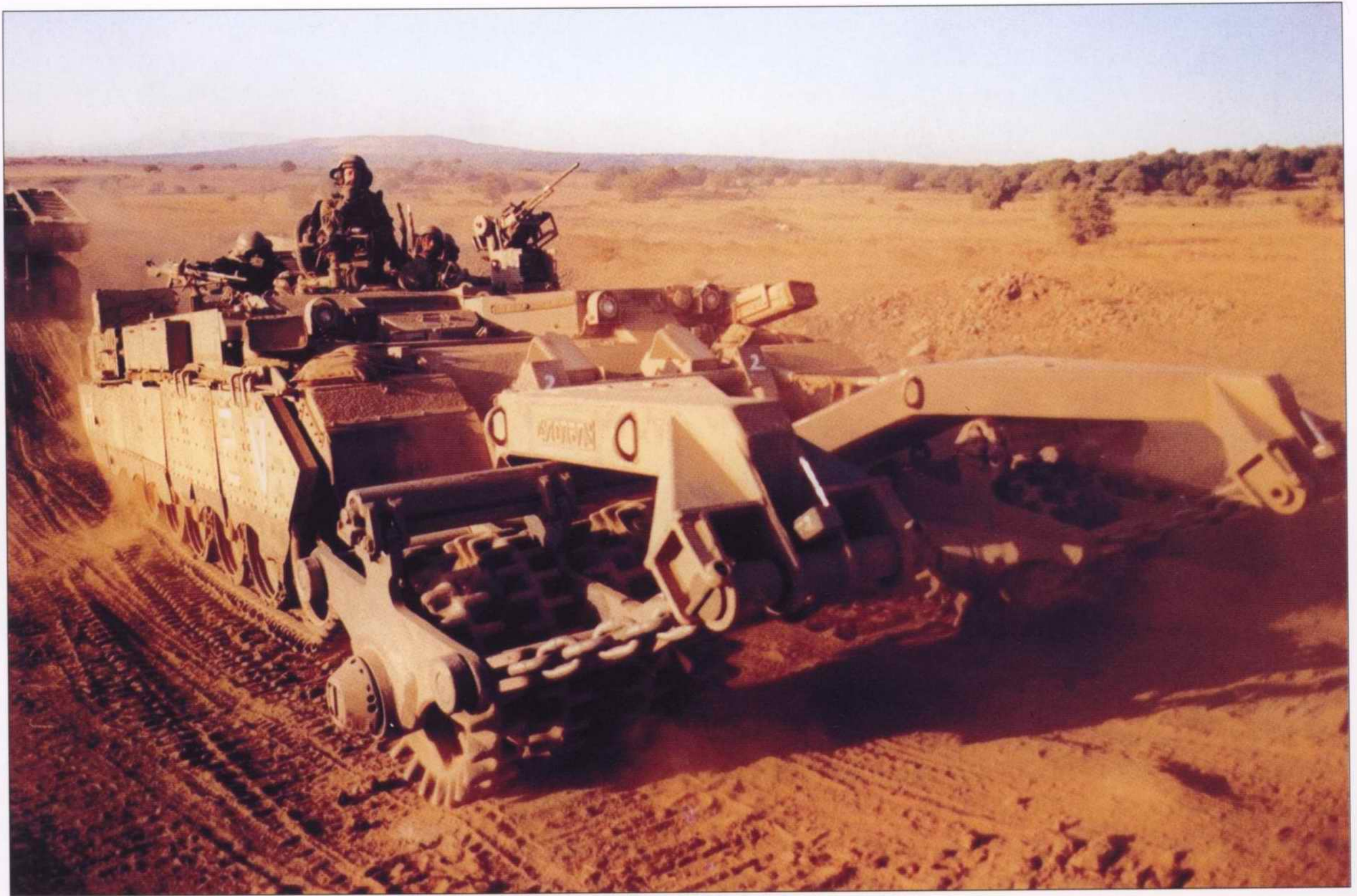
A Puma photographed in 2001, fitted with an RKM mine roller system. Despite the vehicle's bulk, it has a low silhouette. (Nadav Ganot, via the Israeli Government Press Office)
