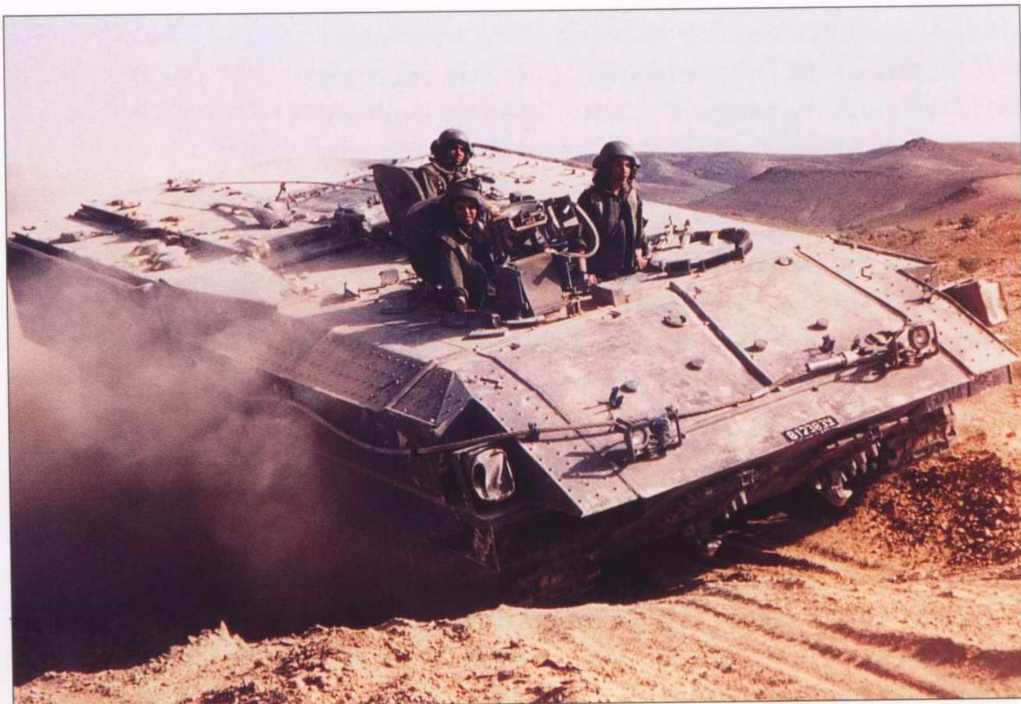
An Achzarit returns to base, Negev desert, 1997. The commander and the gunner are female instructors in training. Note that the Rafael OWS is missing its 7.62mm machine gun.
