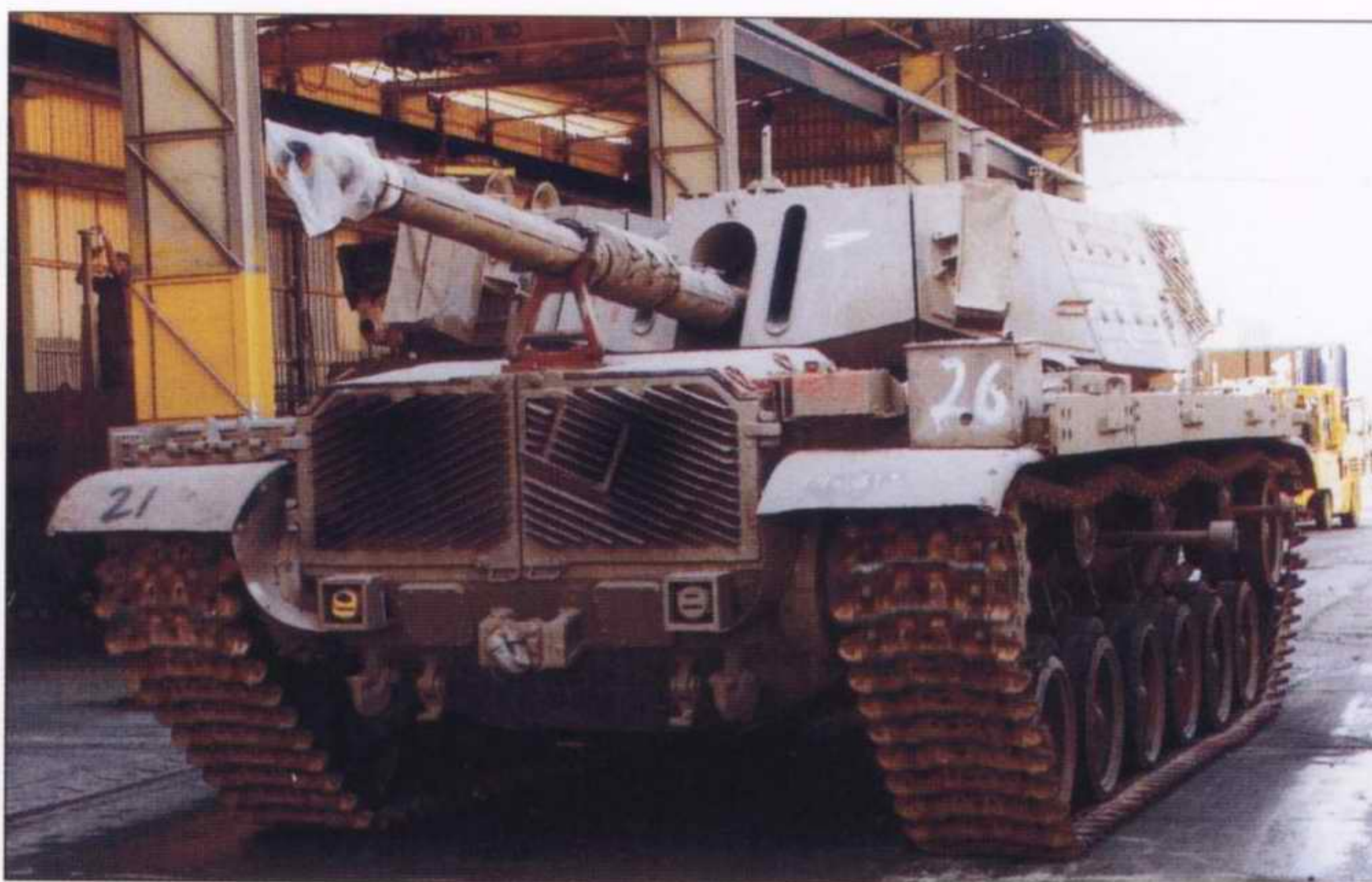
A Magach 7A trundles to the workshop for repair, December 2002. The tracks are in urgent need of re-tensioning. No matter how much the turret profile has been changed by appliqué armour kits, the engine grille betrays the tank's M60 origins.
