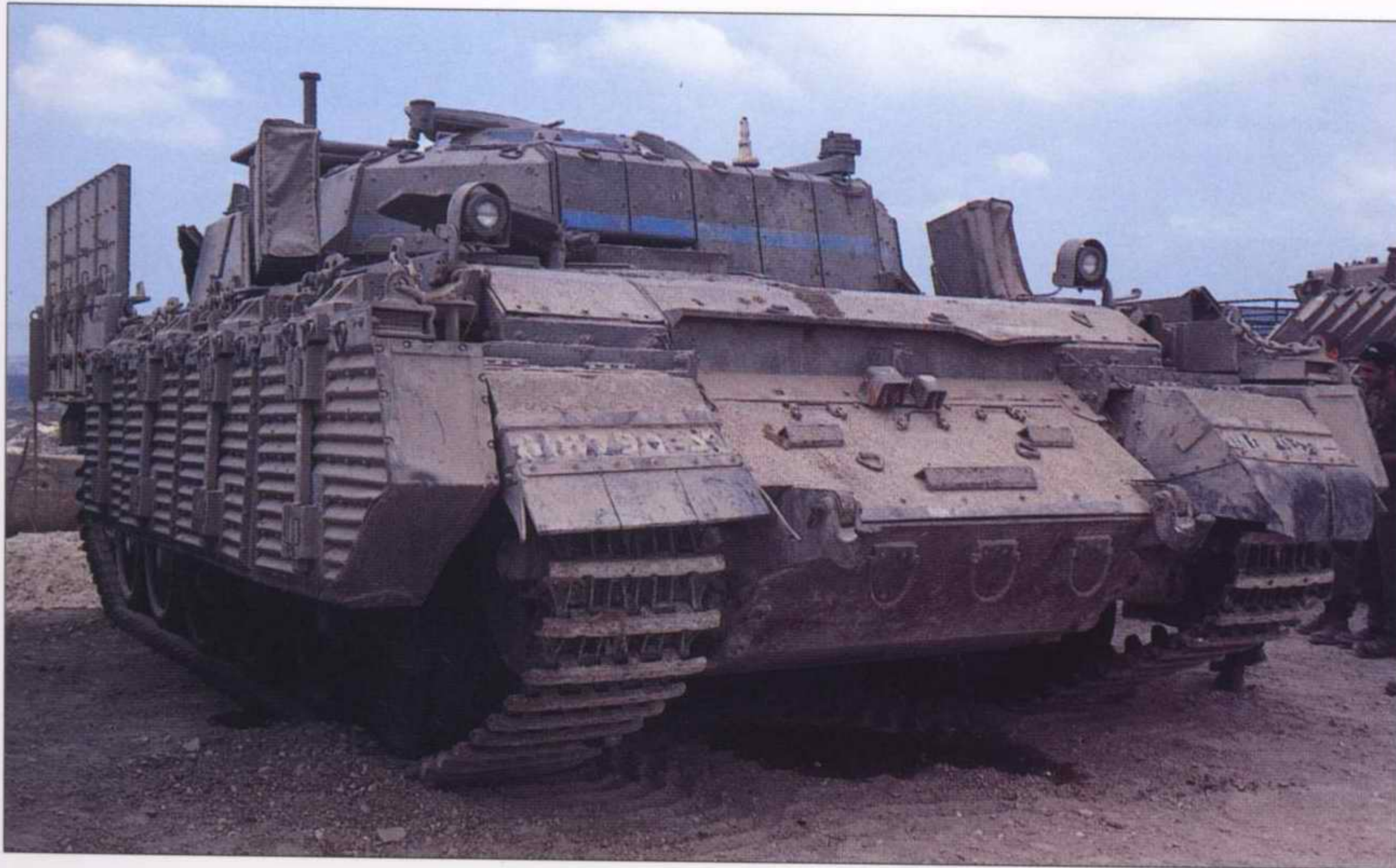
A Nakpadon photographed at Elyakim base, upper Galilee, 2000. It has a less cluttered appearance than the Nagmachon and its formidable side skirts have a corrugated appearance.
