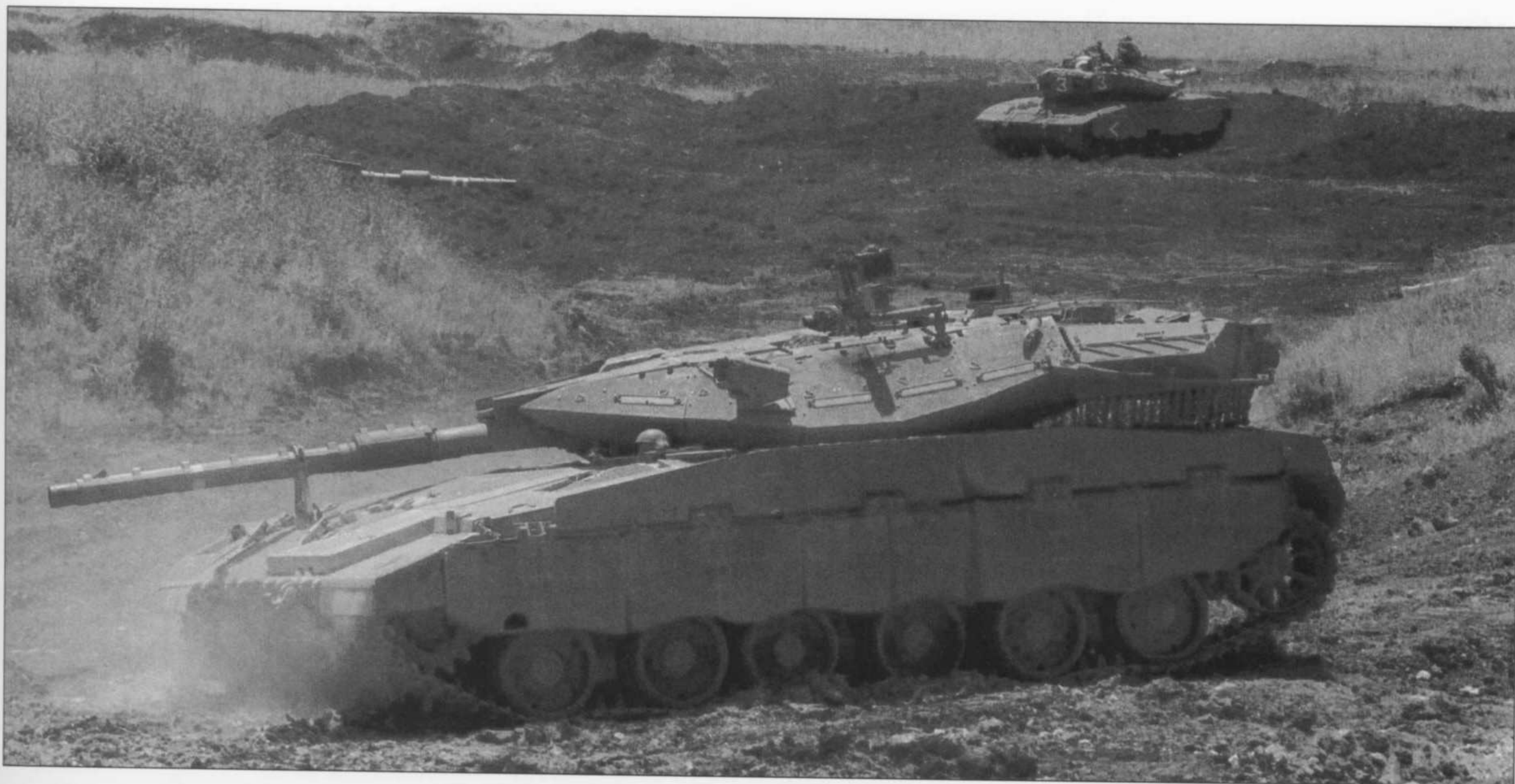
A Merkava 2 Dor Dalet, photographed in 2000 with Merkava 3s in the background. The add-on armour modules give a sleek silhouette. Note the heavy slab of armour protecting the driver's station. (Moshe Milner, courtesy of the Israeli Government Press Office)
