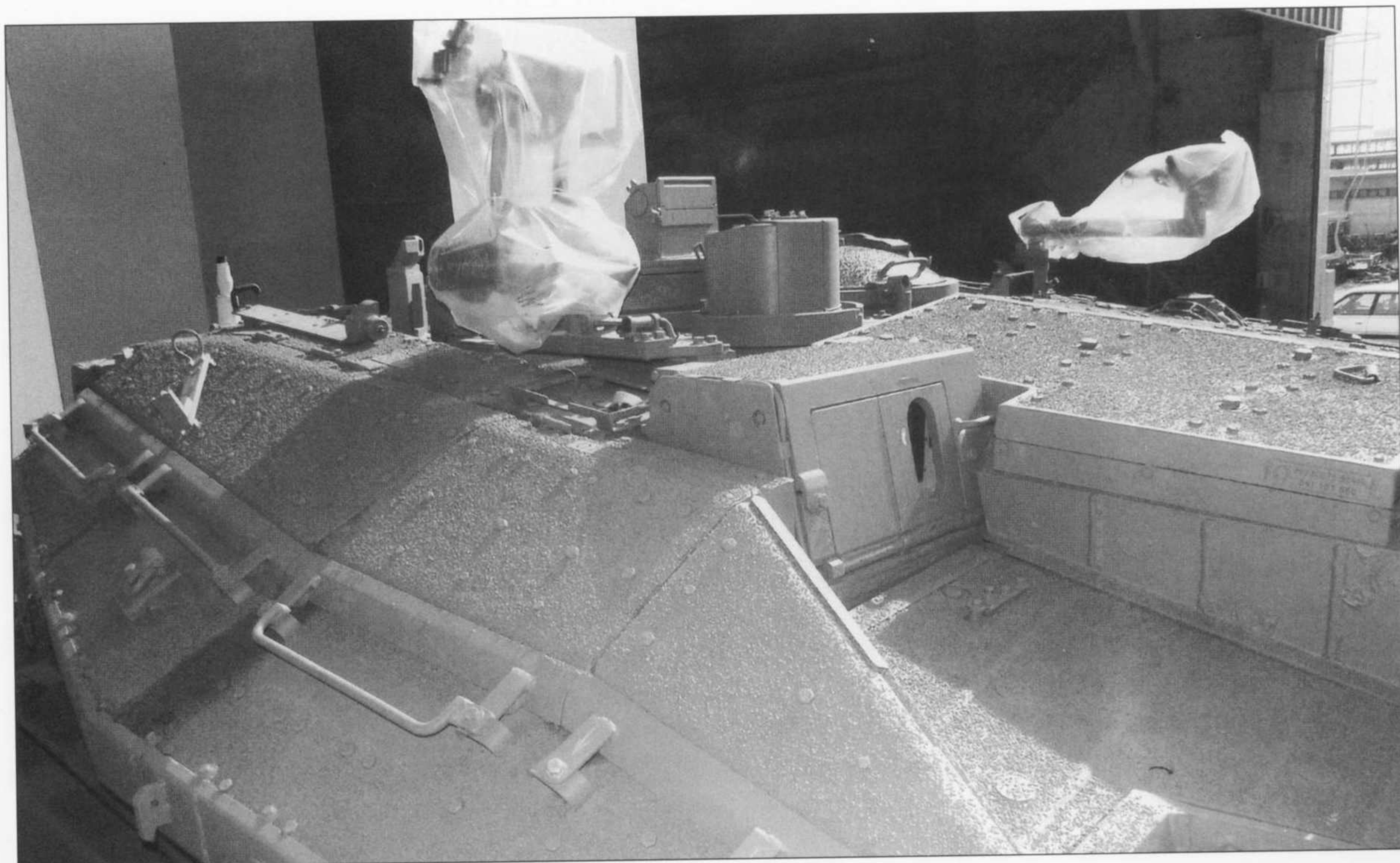
A close-up of the Merkava 3's turret fitted with appliqué fourth generation armour, photographed in 2002. The turret armour has a textured, non-slip surface and a stepped appearance. Note the independent commander's and gunner's sights.
