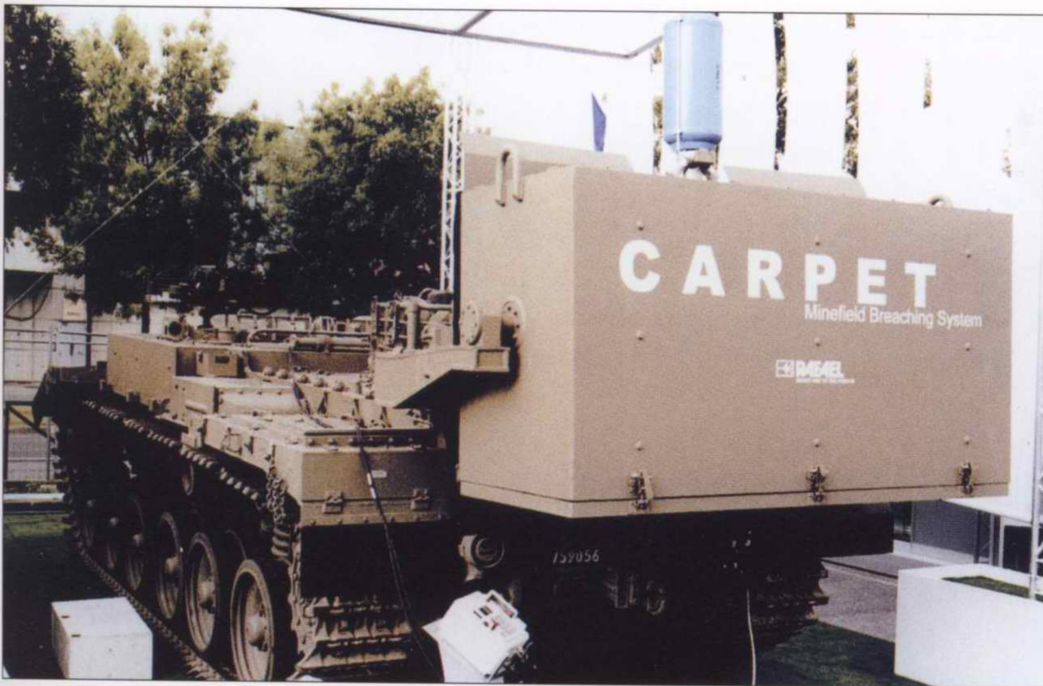
A Puma at the Eurosatory arms exhibition, June 2002, fitted with a Carpet minefield breaching system. An inert rocket is displayed at the top of the Carpet system module. (Stephan Marks)
