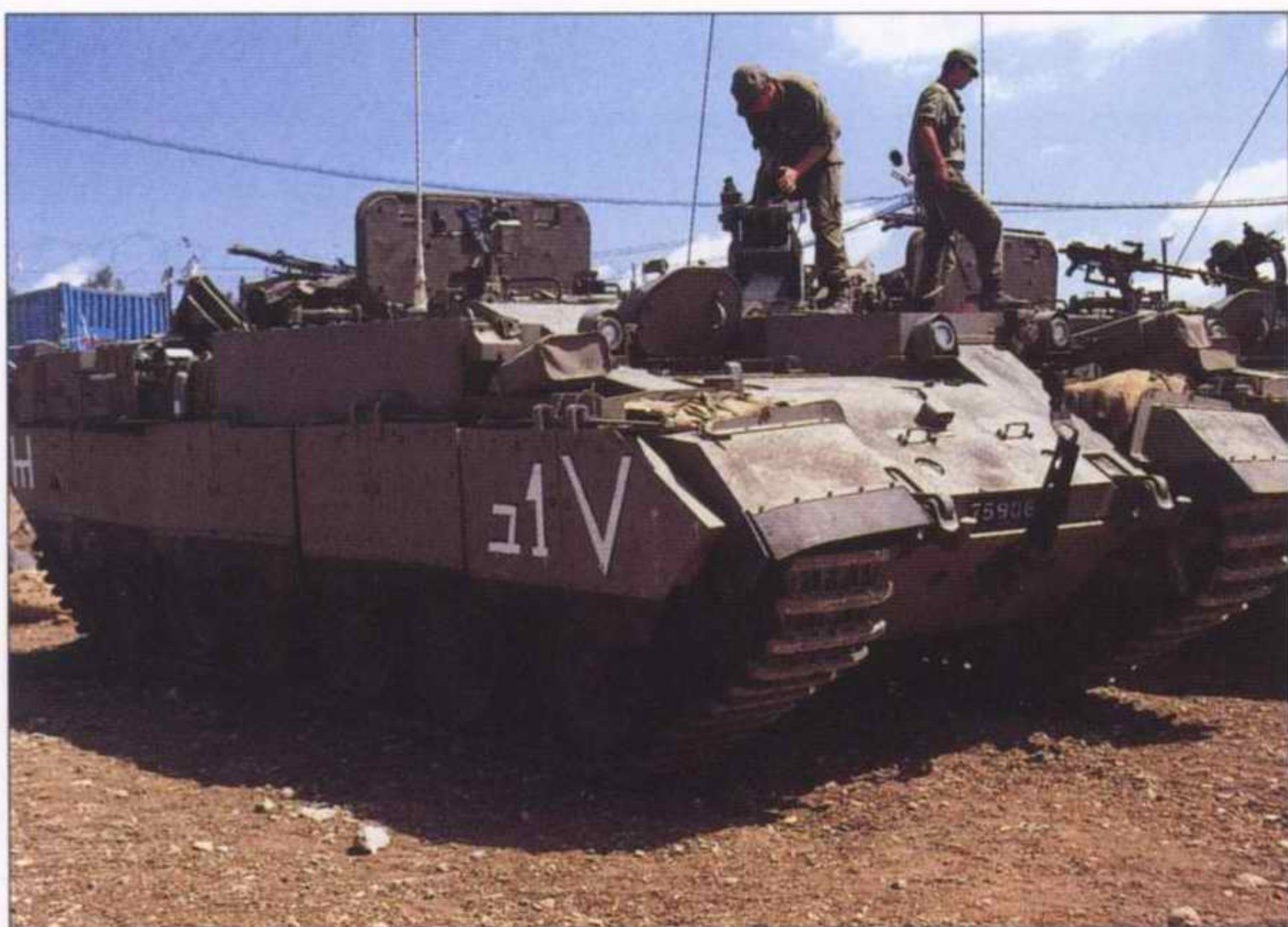
Pumas photographed in upper Galilee, 1996. The insignia on the nearer vehicle's far left, shows that it belongs to the combat engineers. Note the heavy appliqué armour found on the front sections of the side skirts.
