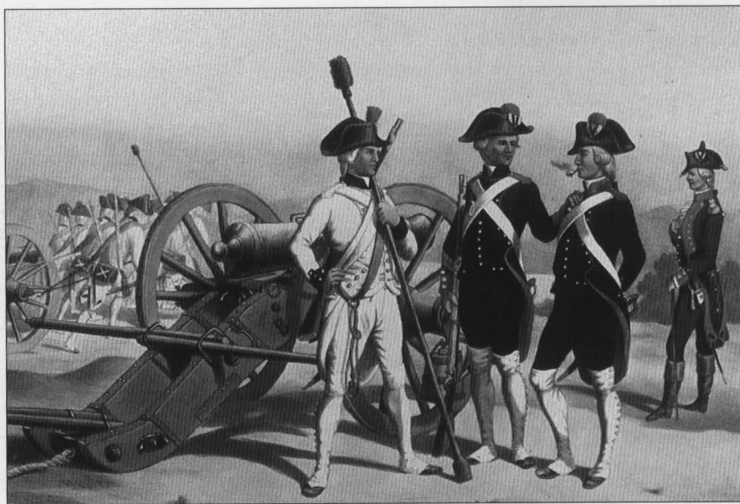
A Gribeauval 4-pdr field piece, c. 1786. Note the rods to manoeuvre the guns easily. The gunners wearing the white uniform are members of the reserve provincial artillery units (disbanded in 1789) and wear the bricole . Those in the background are shown pulling a field piece using their bricoles . Print after Moltzheim. (Anne S.K. Brown Military Collection, Brown University, USA, photo by René Chartrand)
