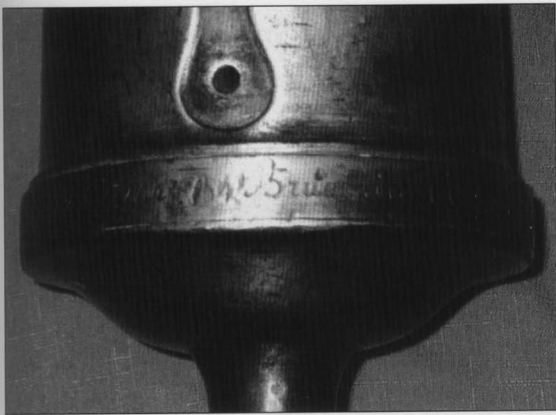
Breech detail of the light 3-pdr brass field gun barrel cast by Ramius at Le Creusot in 1794. The breech plate is engraved 'Ramius au Creusot Brumaire L'An 3'. (Val Forget, Navy Arms, USA)
