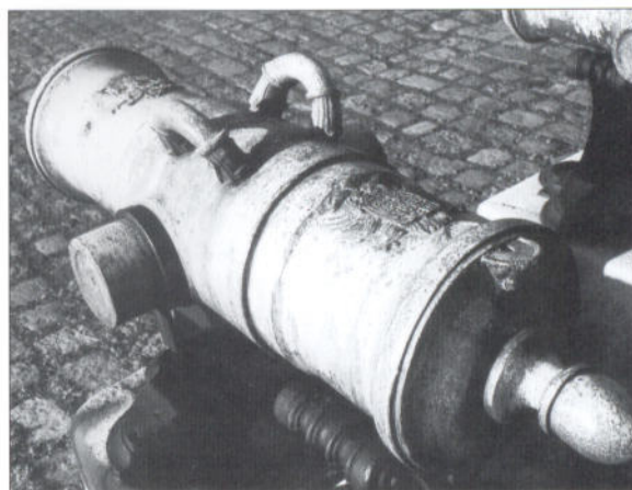
A 7-pdr howitzer barrel. The wider bore extended as far as the rear end of the thicker part.
