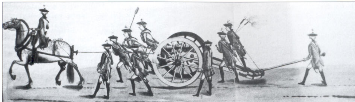
A 7-pdr howitzer being moved. This howitzer was allocated a three-horse team, so to move it in action the lead horse was unhooked from the limber and then connected by the drag rope to the front hook on the carriage. Manpower was also provided by the crew who would drag the gun by means of canvas straps slung over the shoulder nearest the gun and connected to it by ropes, which hooked through the drag hooks at the front and rear of the carriage.
