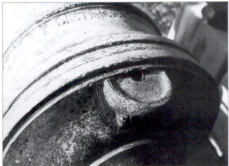
Details of the 1753 and 1780 touchhole designs. The vents were initially drilled at an angle through a rear touchhole support, so that the empty fuse tube was thrown clear of the crew on firing. In 1780 this design was changed to a vertical vent in the main part of the gun, which was easier to bore and, being shorter, was less prone to blockage.
