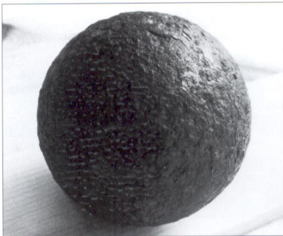
A 6-pdr shot from the Aspern battlefield. Note the surface damage caused by a mix of the effects of the original casting and the firing process. (M. Baulesch)
