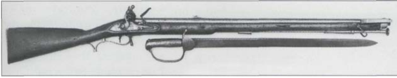
A Baker rifle manufactured by W. Ketland, of the usual dimensions and calibre, but made without a butt box. (Wallis & Wallis)
