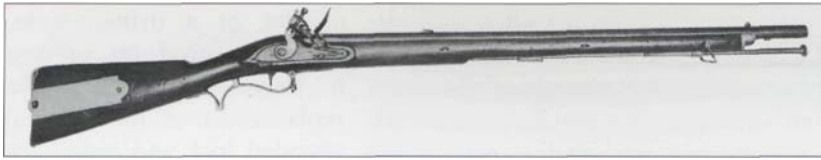
A Baker rifle with provision for a socket bayonet, with the bayonet locking-lug beneath the barrel; it has the first type of butt box and a folding back-sight. (Wallis & Wallis)
