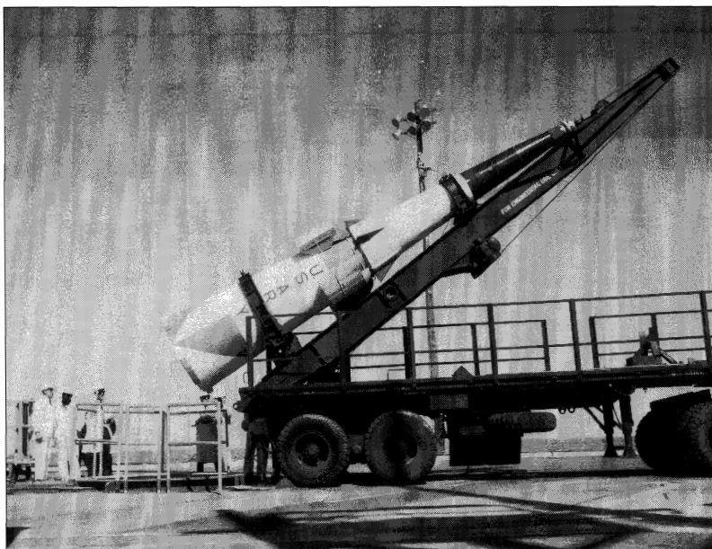
A Sprint missile being loaded into a launch cell. (National Air and Space Museum, Smithsonian Institution)
