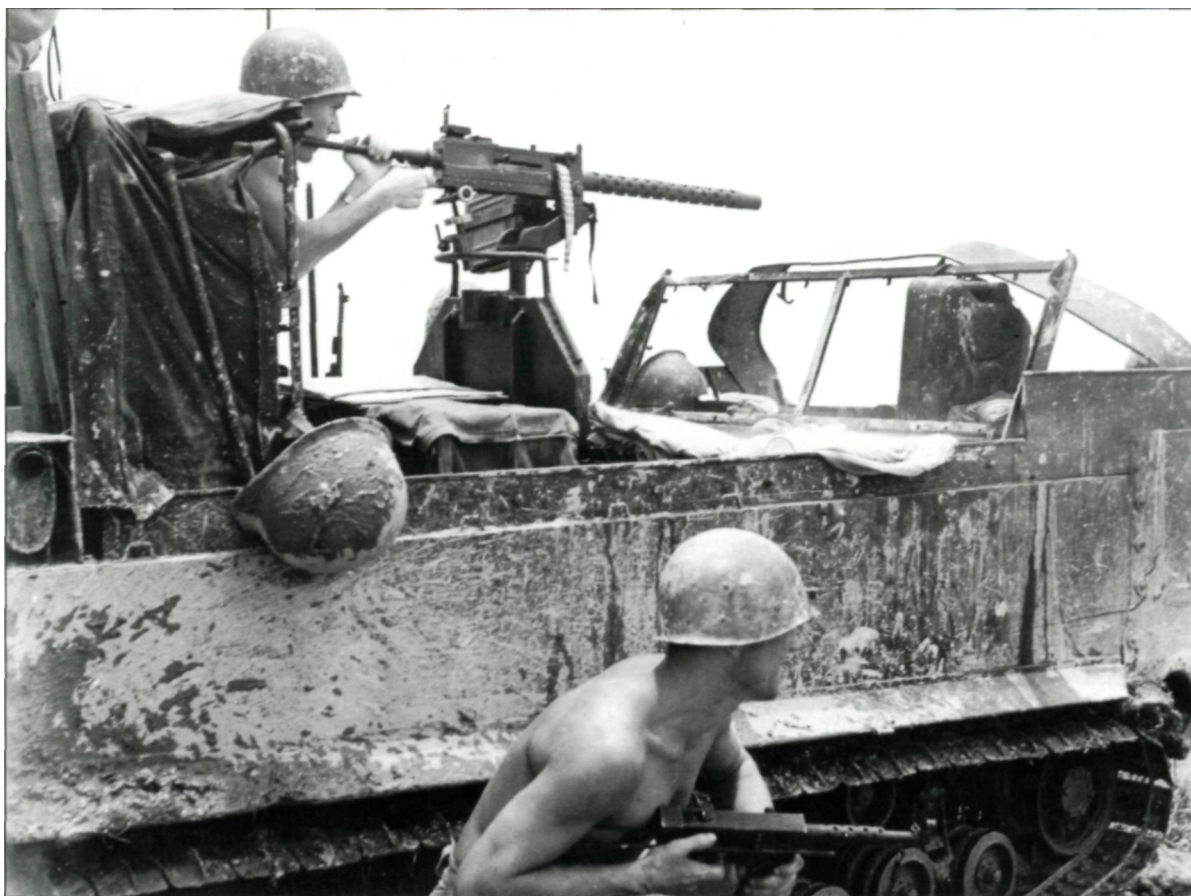
Tonkin, May 1952: during Operation Dromadaire near Hung Yen, a 1 er REC trooper of the 2 e Groupement Autonome mans the .30 cal. on his Crab. The M29C was never designed as a combat vehicle, but the Legion fitted them all with .30 cal. or LMGs, and those of support elements with 57mm recoilless rifles. (ECPA)
