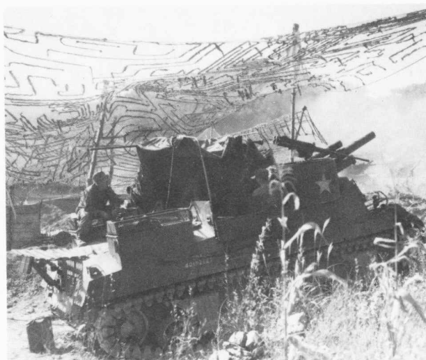
Many of the AFVs employed in Korea were of Second World War vintage, such as this M7B1 105mm Howitzer Motor Carriage of 'C' Battery, 300th Field Artillery Bn. firing in support of 1st Marine Div. during the battle for Hill 785, near Injeon 22 September 1951. A number of these vehicles were modified during the war by raising the howitzer mounting to increase the maximum elevation from +35 to +65 degrees; this conversion, designated M7B2, made easier the placing of indirect fire on the reverse slopes of steep Korean hills. (US Army SC381292)
