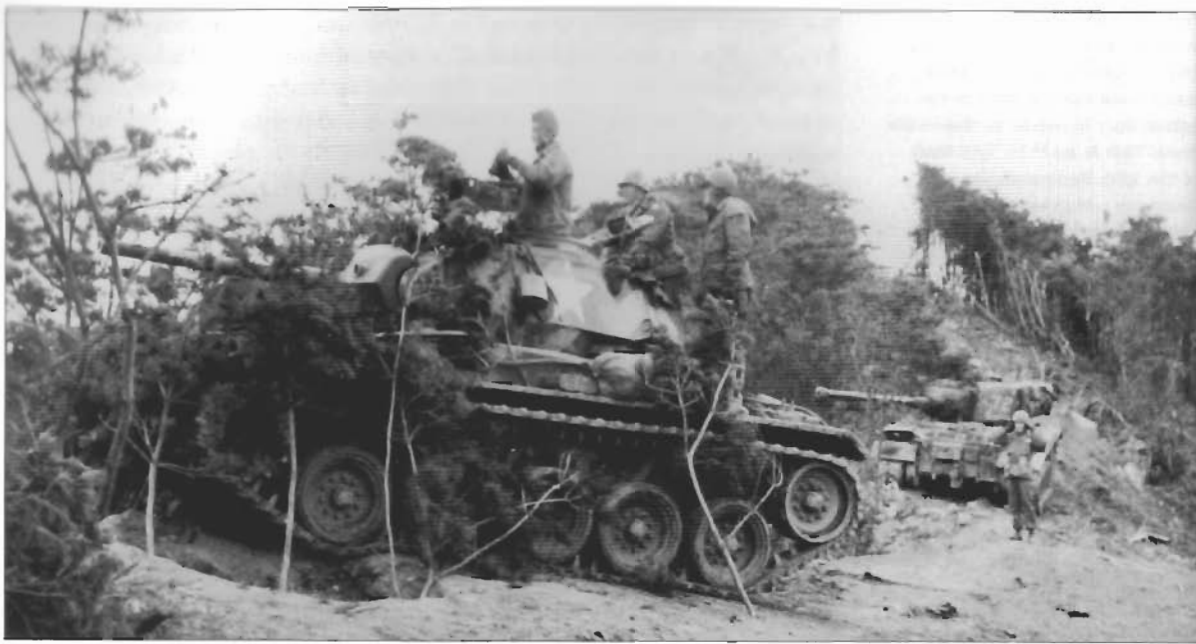
A well-camouflaged M24 Chaffee of the 64th Tank Battalion rests behind a ridge line while supporting the 3rd Infantry Division south of Seoul in February 1951. Behind it is one of the battalion's M46 heavy tanks. When used in its intended role as a reconnaissance vehicle, the M24 performed well. This M24 is unusual in that it has pattern-painted camouflage on the turret, which was uncommon in Korea. (US Army)
