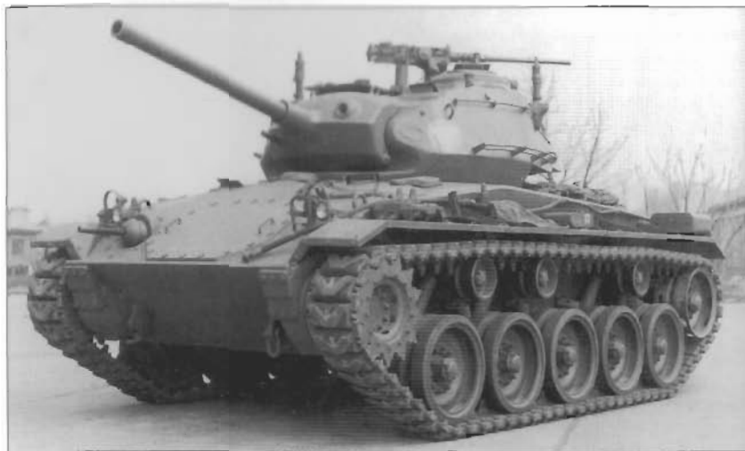
Austria was one of a number of non-NATO countries to receive the M24 through MDAP grants. This is a good example of the vehicles after their postwar refit showing the added radio aerial over the smoke mortar port, the added front machine gun pintle, as well as the medical box and jerrycan rack on the fenders. It is a late production type fitted with the attachments for the pontoons on the lower bow plate, but by this time they have been plugged up with bolts. Most postwar M24s were fitted with the T87 rubber block track as seen here, instead of the steel T86 track seen during the war years. (Osterreich Heeresbild)
