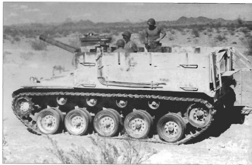
This M37 105mm GMC is seen on trials in the Mojave desert by the Desert Warfare Board in 1945. It has become so caked in dust that it appears almost white. The "L"-shaped brackets on the hull side are hoops used to mount a foul-weather tarp over the fighting compartment. (Patton Museum)
