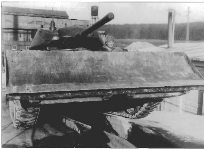
The M4 dozer blade was finally developed for the M24 tank, which differed from the experimental type in that it did not require the extensions along the hull side. This dozer was seldom seen fitted to the M24 in serving units, and this example is seen at the Butzbach depot in Germany serving with the 9th Reconnaissance Squadron in January 1946. Notice that the 60mm smoke mortar port on the turret roof has been modified to permit a second radio aerial to be fitted. (NARA)
