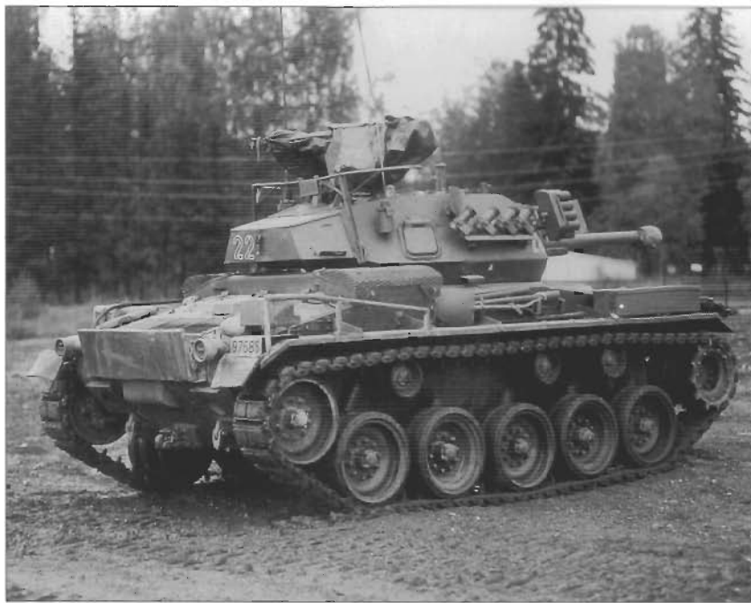
The Norwegian Army rebuilt some of their M24 light tanks in the mid-1970s as the NM-116. This added a new French 90mm gun, advanced fire controls, new track, and a new diesel engine. These remained in service for nearly two decades, finally being retired in 1992-93. (Norwegian Army)
