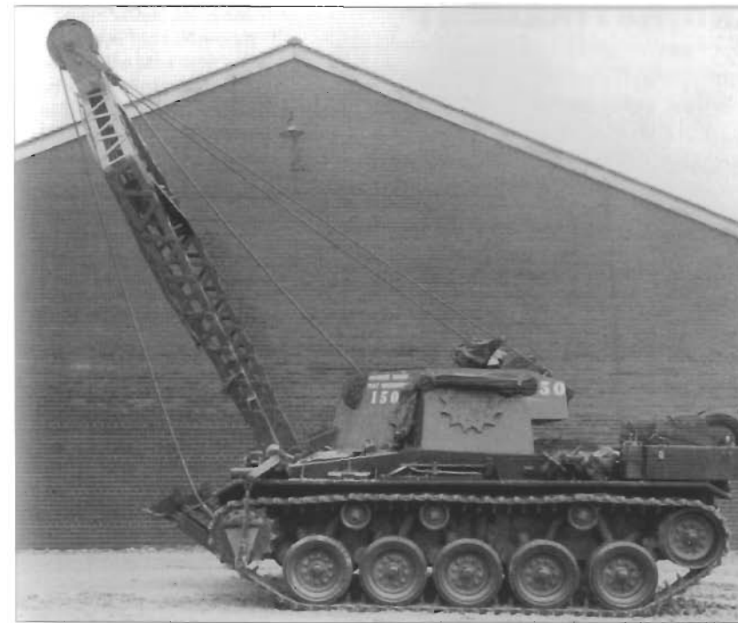
There was some interest in light tank units for a specialized light recovery vehicle, leading to the development of the T6E1 recovery vehicle. A pilot was completed in September 1944 and put through trials with the Armored Board at Fort Knox as seen here. Although it proved to be an effective design, production never started as development was not complete when the war ended in August 1945. (Patton Museum)
