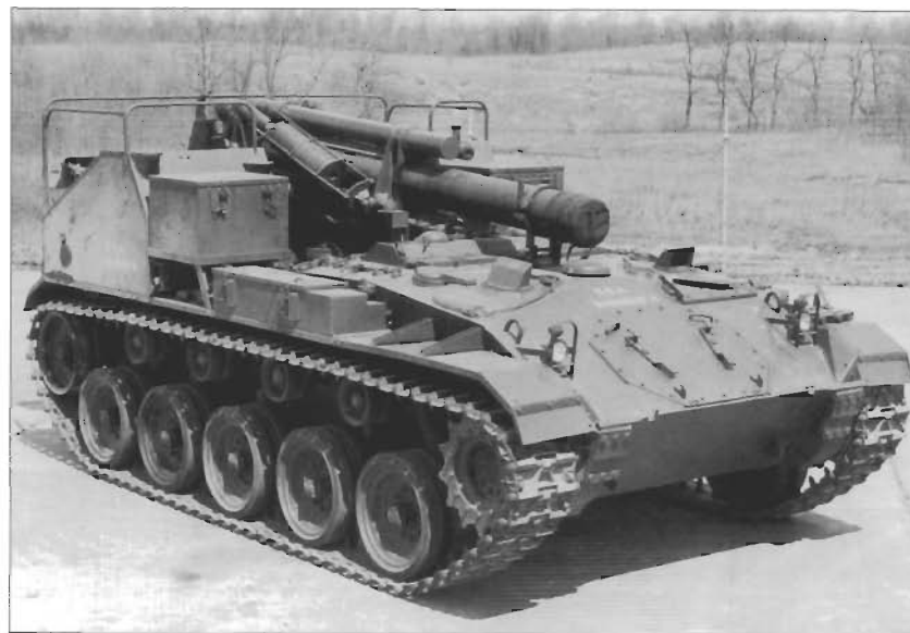
This is an early production example of the M41 155mm HMC manufactured in the summer of 1945. The M41 arrived too late for combat use in World War II, but did see action in the Korean War with a number of artillery battalions. (Patton Museum)
