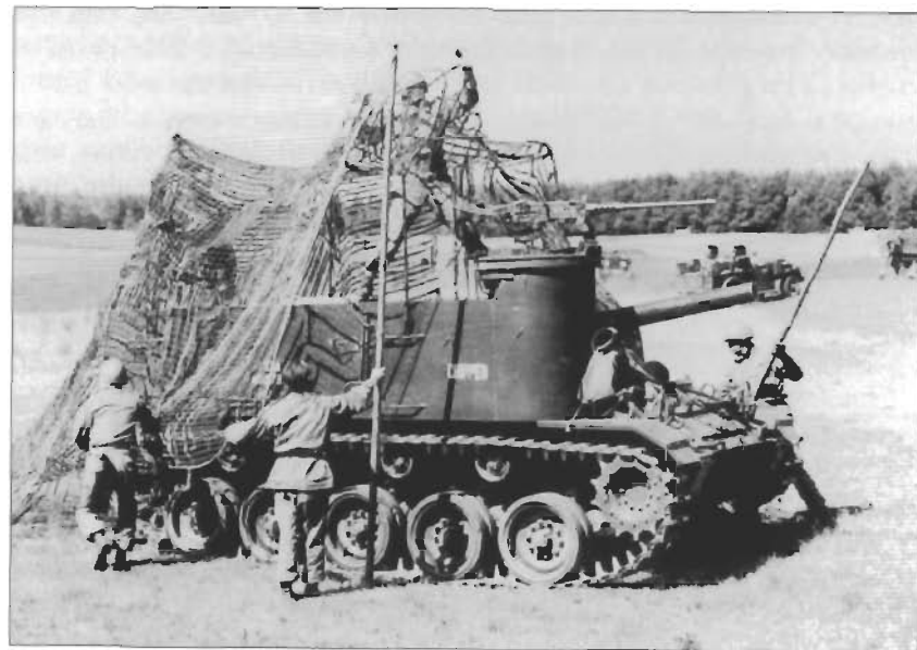
The M37 105mm HMC became the backbone of US Army armored field artillery battalions in the early 1950s. It was deployed in Germany until the mid-1950s when it was gradually replaced by the M52 105mm HMC, a fully turreted design based on the newer M41 light tank chassis. (US Army)
