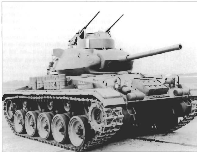
The M24 also served as the test-bed for a variety of weapons options including the T122 machine gun mount seen here in 1947 at the Aberdeen Proving Ground. This remote-control mount was armed with a pair of .50-cal. machine guns, but there was little demand for such a weapons mount and it did not pass beyond the test stage. (NARA)
