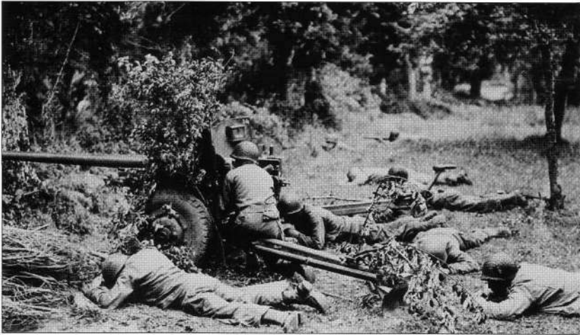
Normandy, 1 August 1944: a US crew man a 57mm M1 anti-tank gun (a licensed version of the British 6pdr) behind a hedgerow only 200 yards from the enemy. This remained the standard US infantry AT gun until the end of the war. Although its maximum range was over 10,000 yards, it needed to be far closer to do its job: it could penetrate just under 3in (76mm) of armour at 1,000 yards – not enough to pierce the hull or turret frontal plates of a Tiger, Panther, or even a late-model PzKw IV. (US National Archives)
