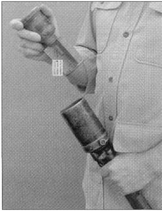
The No.68 anti-tank grenade, thrown from a rifle cup discharger. The tin label reminded the user to remove the safety pin before inserting the finned tail into the discharger.
