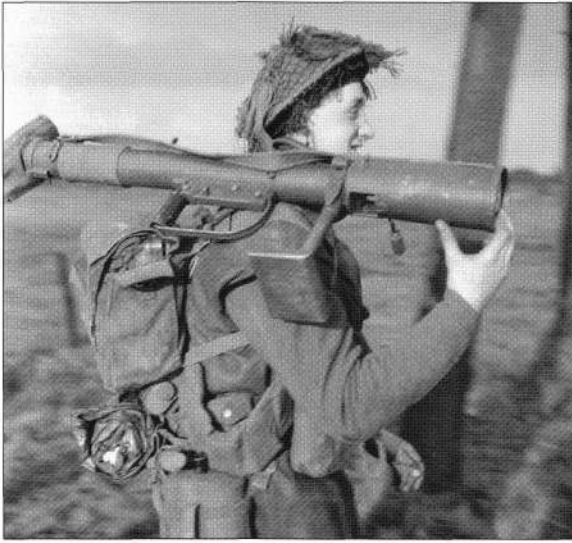
A heavily loaded British PIAT gunner - including uniform and webbing, the total weight being carried here is about 80 pounds. Despite the sling the weapon is more comfortable on the shoulder. The hanging cork was used to plug the spigot hole when the weapon was cocked but unloaded, to keep rain out of the mechanism. Interestingly, just visible between his small pack and rolled anti-gas cape is the unmistakable 'talcum powder tin' shape of a No.75 'Hawkins' anti-tank grenade. A versatile and fairly safe device which proved highly effective for blowing the tracks off Panzers, this was also adopted by the US Army. (IWM)
