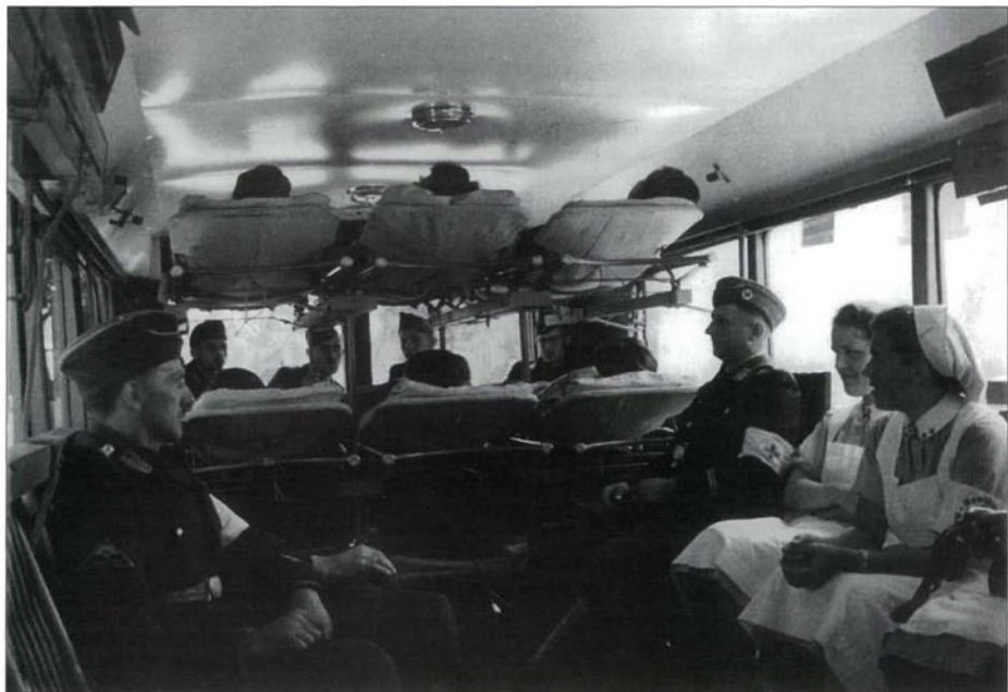
Interior view of a German Red Cross rapid response vehicle, looking from the front towards the rear doors. In addition to the crew this large bus, with convertible seats and removable stretchers, was capable of carrying 18 stretcher cases or 30 seated patients.
