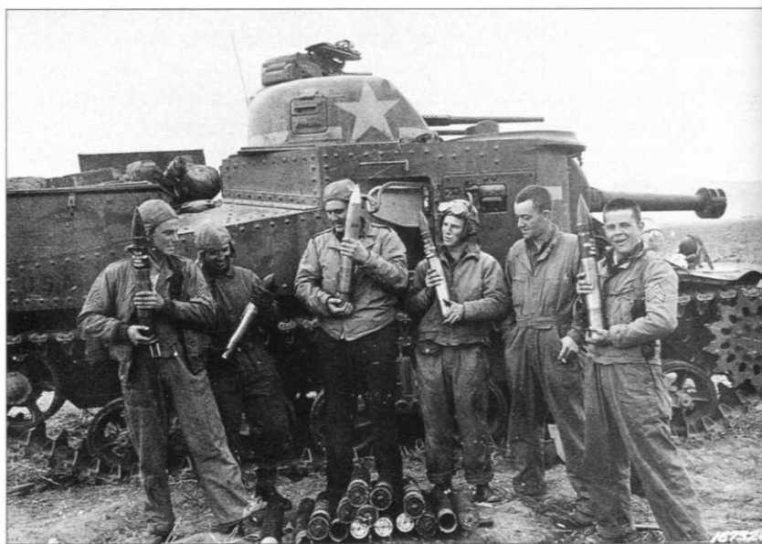
North Africa, January 1943: the crew of a 1st Armored Division M3 Medium tank (Grant) unpack 75mm shells from their black cardboard shipping tubes. Most wear HBT overalls with a mixture of 'M1941' Parsons field jackets and cold weather 'tanker' jackets. The three men at the left wear the light khaki padded fabric 'winter combat helmet' which was designed to fit under the hardened leather 'armored forces helmet', worn here by the third man from the right. By the end of the Tunisian campaign M4 Shermans had replaced most M3s in US Army tank units.
