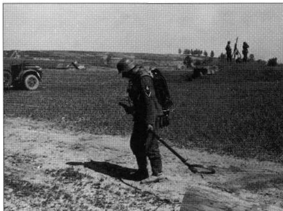
Minesweeping was a constant task for the field engineers in the German Army, as the Russians always mined roads if they had time. The equipment is a Frankfurt 40 detector. At the rear is a light anti-aircraft position.
