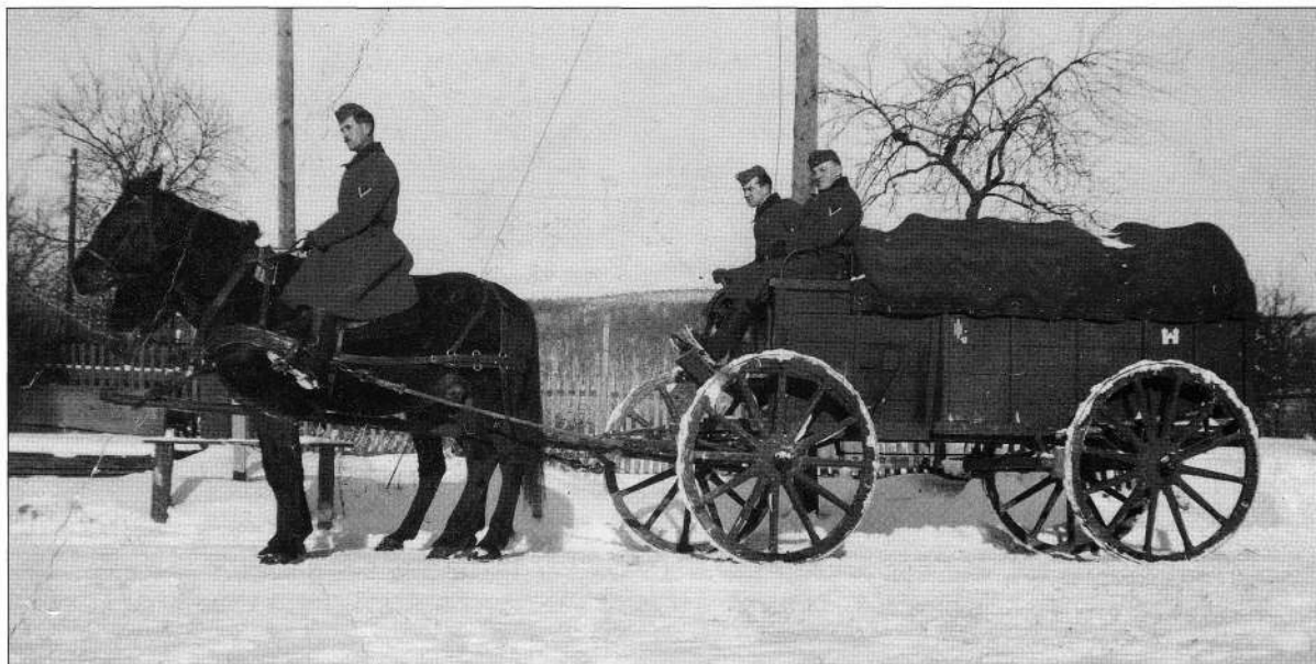
The infantry wagon with two horses, driver and two seated men. The Gefreiter is in charge of the wagon and its horses. This is the Hf.2 version; the later Hf.177 metal wagon was so heavy it earned the nickname 'horse murderer'.
