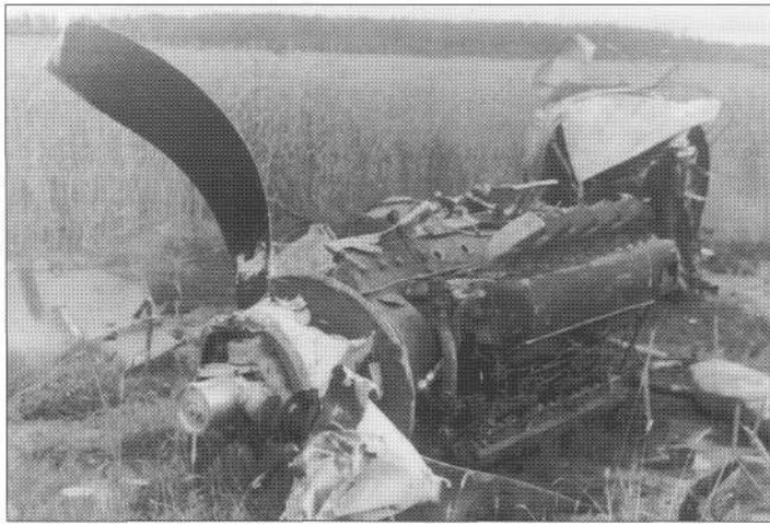
The engine of a Russian Yak-2 aircraft which has been shot down by flak. The aircraft was one of the most successful ground-attack aircraft used by the Russians and was fitted with two 23mm cannon and three machine guns and could carry 600kg (1,322lb) of bombs.
