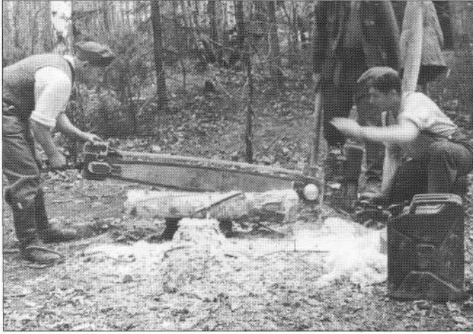
Two men using a light electric chain saw. The equipment weighed 50kg (111lb), had a cut of 1m (3ft 3in), and could cut at a rate of 6.4m (21ft) per minute.
