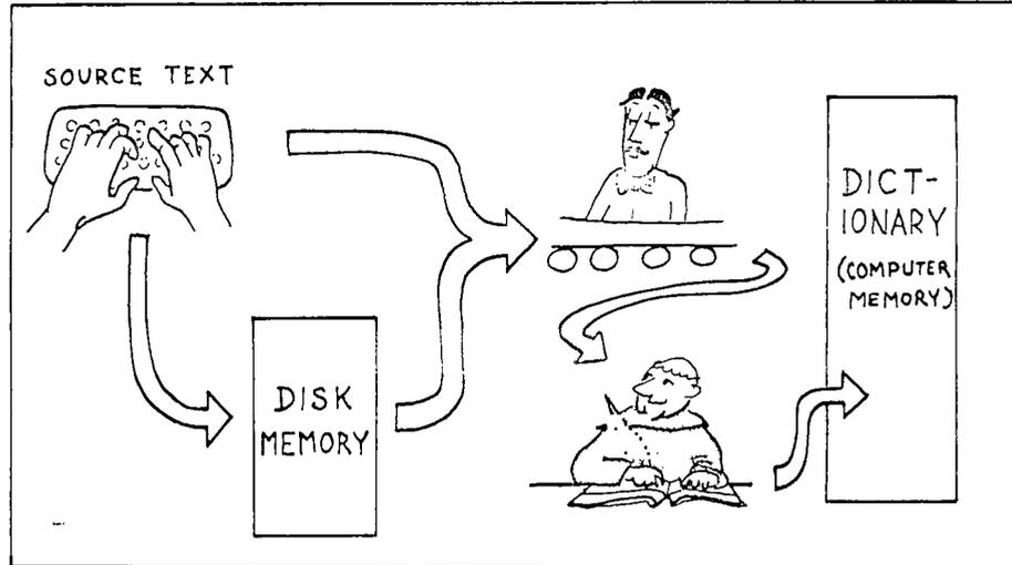
Disk memory is divided into units called "blocks." Many professional FORTH development systems have 500 blocks available (250 from each disk drive). Each block holds 1,024 characters of source text. The 1,024 characters are divided for display into 16 lines of 64 characters each, to fit conveniently on your terminal screen.
