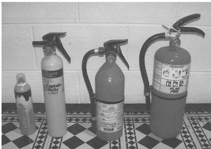
Typical fire extinguishers, like those above, are available at most home supply stores. In terms of fire extinguishers, bigger is better. Inspect your extinguishers regularly. The larger ones on the right can be refilled and repressurized.
