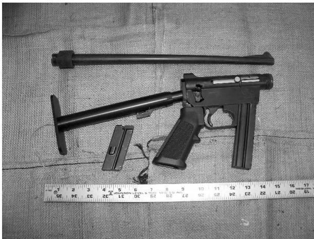
AR-7 with barrel removed and stock collapsed is only fifteen inches long and takes up very little room in the pack. The barrel can be attached in a few seconds.
