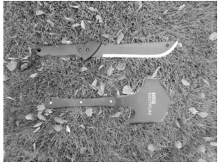
Top: a medium-length machete with a sawblade on the back; Bottom: a “Recon-Tool combination axe, shovel, and saw. Both are good tools for extended survival situations.
