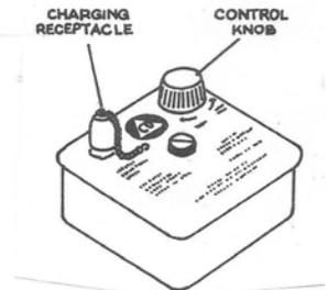
Surplus civil defense survey meters such as the CV-700, 751, or 720 can be purchased at reasonable costs. Some are calibrated and others are not, but calibration services are also available. These CD V-742 pocket dosimeters and CD-V750 chargers are also still available. These are used to register personal exposure rather than area radiation.
