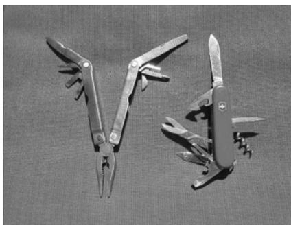
Multi-tool device and Swiss Army knife. Both have a variety of devices and blades. Newer versions of the multi-tool have blades that open and lock from the outside like a regular pocket knife making them much more effective.
