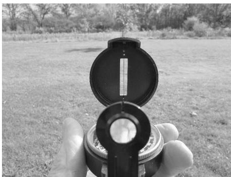
This compass is sighted on a tree at about 80 degrees (slightly north of straight East).
