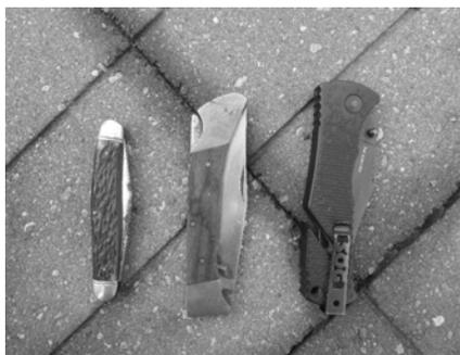
Left to right: A small low-cost, two-bladed pocket knife. Basic lock-blade pocket knife and high-end knife with seat-belt cutting notch, safety-lock, and belt clip.
