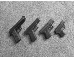
Automatic pistols come in all sizes. Left to right: full-size 9mm, medium-frame 40-caliber, compact 9mm, and subcompact 380 caliber. The full-size weapon has a seventeen-round magazine down to twelve rounds, eight rounds, and just six rounds for the subcompact.
