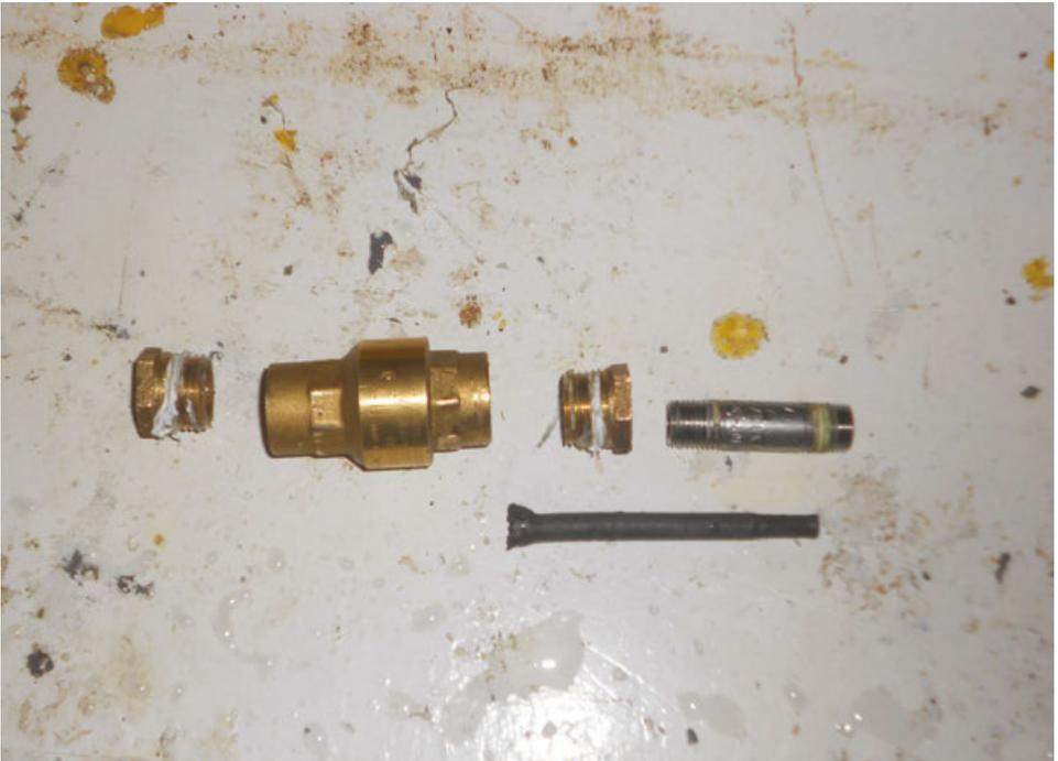
The idea is to create a single acting steam engine (meaning the steam only acts on one side of the piston) by using a pushrod inserted through the spark plug hole to push open the check valve when the piston is at Top Dead Center
