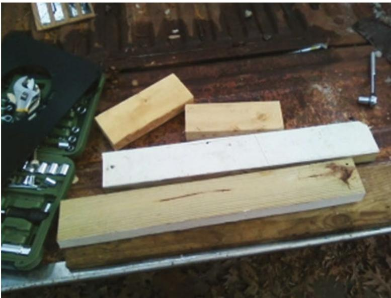
By clamping the open ends of the boards together, it holds the bag, which makes it *much* easier to iron. By facing the mitered edges of the board together, the “sharp” point also makes a crisp seal.
