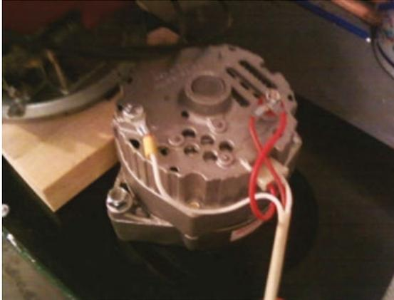
I used their adapter, some 14-gauge red and white wire, a 50 amp switch, some connectors, and heat shrink to rig up a wiring harness that snaps into the alternator. I probably should have used full battery cables to hook the alternator to the battery, but the run is short, the amps are low, and I will be next to the generator while it is running so I can monitor it if it gets hot.
