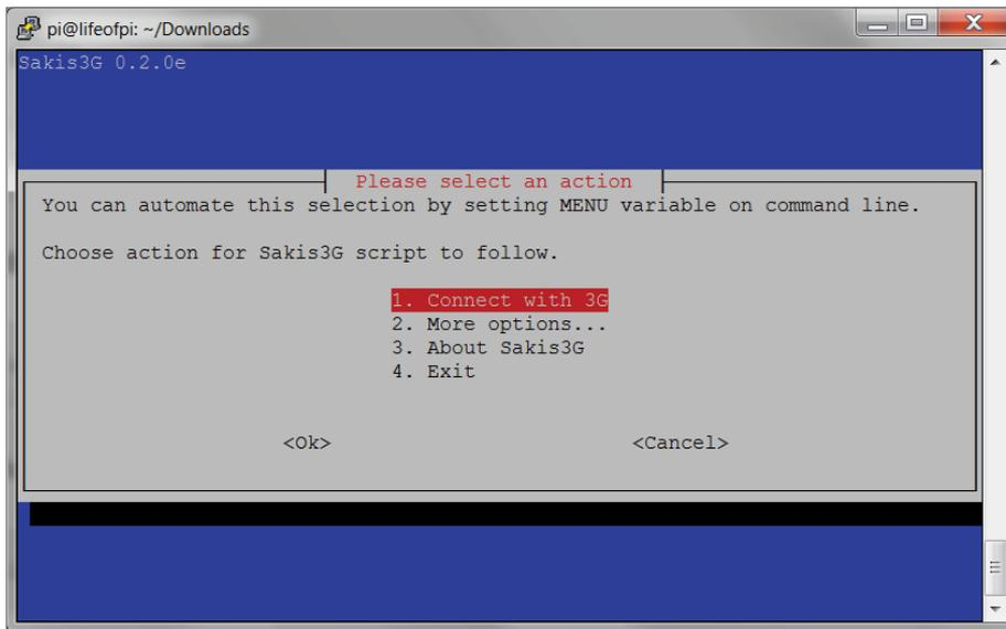
**Figure 6-10:** Step one: connect with 3G.
