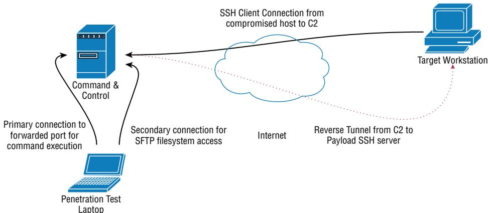
**Figure 1-11:** Initial basic Command and Control infrastructure.
