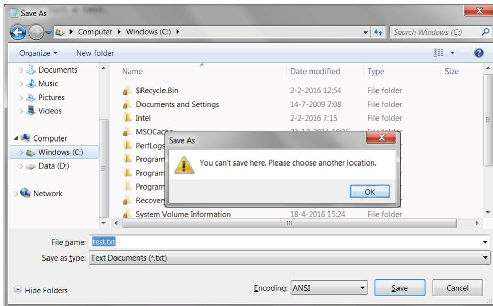
**Figure 4-10:** Notepad cannot write to the C drive. It's a fair bet most desktop software programs have the same restrictions.
