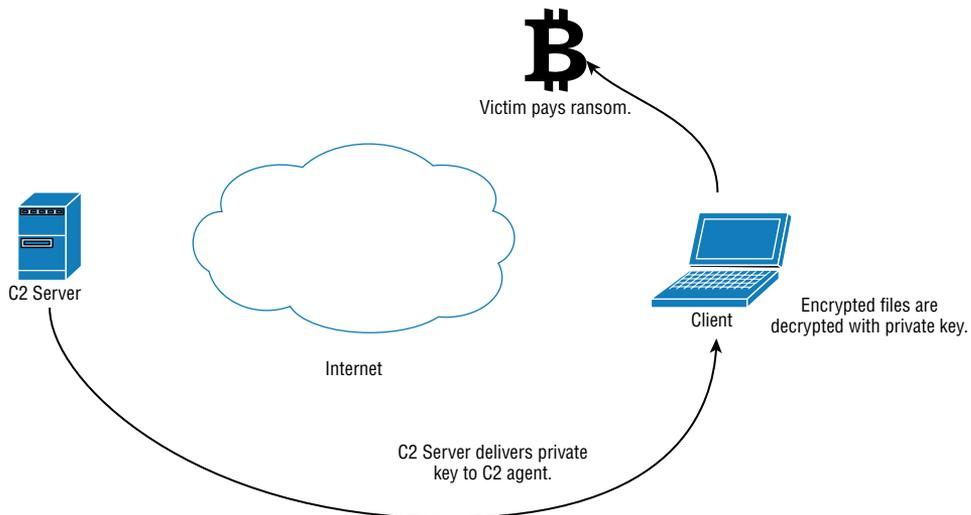
**Figure 5-4:** Decryption process flow.
