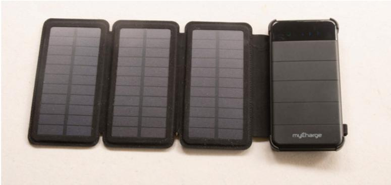
*This battery can be charged with a solar panel and then can charge other electric devices.*
