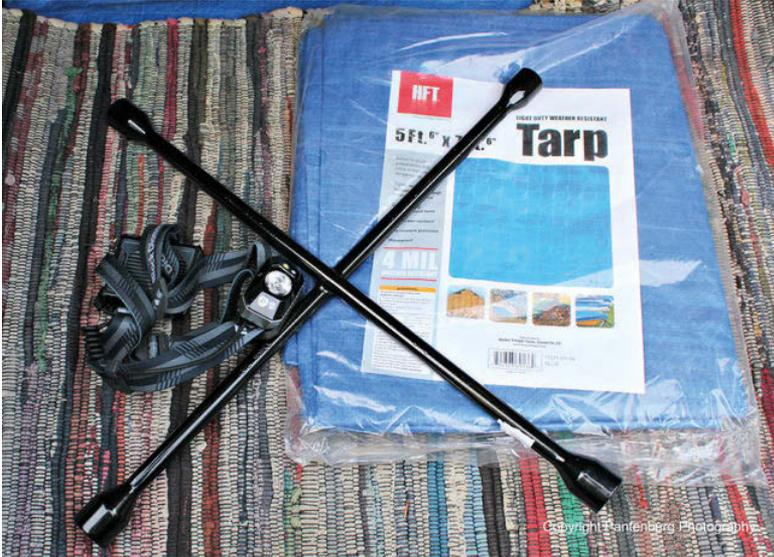
*Always carry in your trunk a rug and tarp for changing the tire, a good tire iron (not the poorly designed irons that come with the car), and headlamp for keeping your hands free.*
