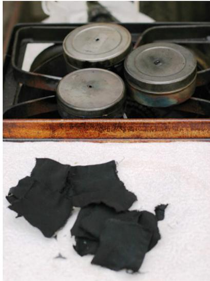
*Charcloth is a material that catches sparks. The organic material is “cooked” at a high temperature in an airless container with an exhaust hole, whereby the cloth is changed through a process called pyrolysis. The charred cloth becomes a source of fuel with a very low ignition temperature.*
