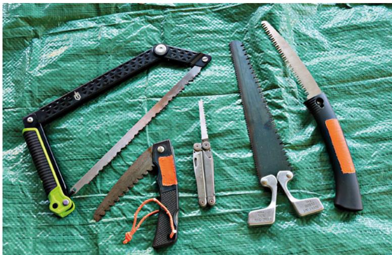
*These represent several different styles of saws. (From left) A take-down bow saw, folding limbing saw, Leatherman saw, Pac-Saw, and wood saw with push blade.*
