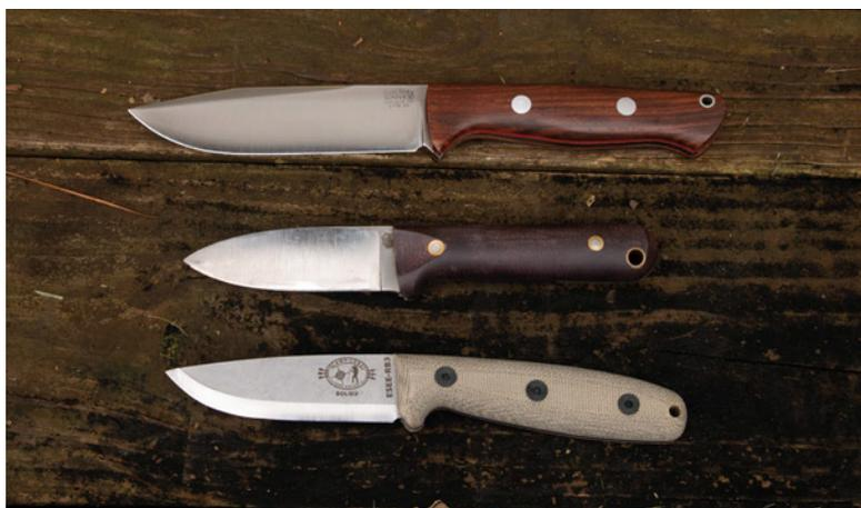
*These three different knife points have different uses and configurations. (From top) They are clip, spear, and drop points.*
