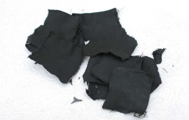
*The finished charcloth should be completely black and slightly flexible. When done correctly, the finished charcloth should easily catch a spark and grow into an ember.*
