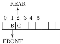
**Step 3:** Similarly, node B is deleted from the queue and FRONT is incremented by 1. Now, insert all the nodes adjacent to B, which is node C, by incrementing REAR. But C has already been inserted in the queue. So now in this case, node C is also deleted by incrementing FRONT by 1, and the node adjacent to C, that is, D, is inserted into the queue. Therefore, nodes A, B, and C are traversed.
