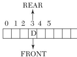
**Step 4:** Now we will again delete the front element from the queue, which is D. We will insert the adjacent node of D, that is, B. But it is already traversed. Finally, as we delete the front element D, we notice that  $\text{FRONT} > \text{REAR}$ , which is not possible. Hence, we have traversed all the nodes in the graph.
