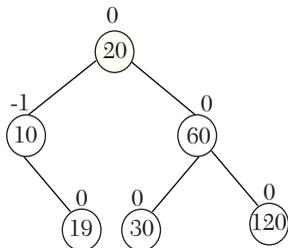
**Step 8:** Insert 100. No rebalancing is required.
