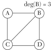
Figure 12.4. Graph showing degree of node B.
