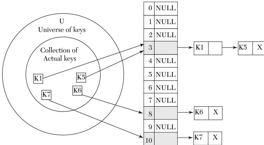
Figure 10.5. Keys being hashed by chaining method.
