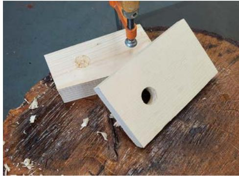
*I drilled this hole from both sides, but I also clamped a piece of scrap underneath during drilling. The scrap supports the fibers to minimize damage if you break through by accident.*
