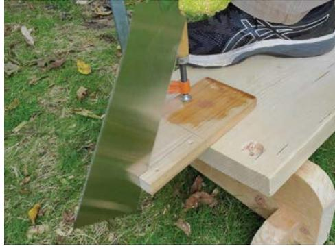
*Drill your clearance holes before you saw the cleat free. Large pieces are always easier to hold.*
