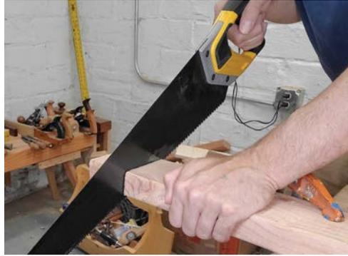
*Pulling back several times with the saw will make a little groove that will guide the cut. As you saw through the board, concentrate on pushing gently forward and keeping your saw straight up and down.*
