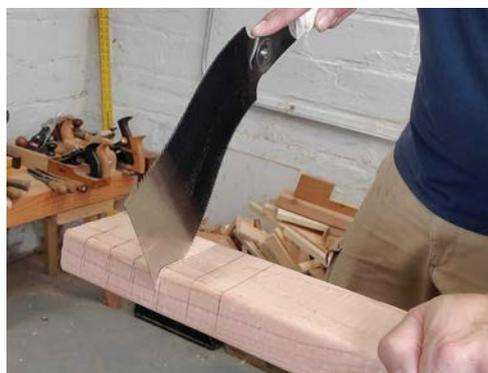
*If your blade bends on the push stroke, you're probably sawing too hard or twisting the handle. Try to relax and keep the blade straight up and down.*
