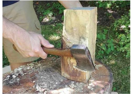
*To trim off the ugly surface of my log, I'm gently chopping down half of one side and then flipping the log over and chopping off the rest. Note that my other hand is holding the log by the top of the far side and my fingers are never close to the cut.*
