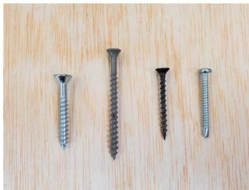
*Left to right: wood screw, deck screw, drywall screw, sheet metal screw. Note the "bugle head" on the drywall screw and the round head on the sheet metal screw.*
