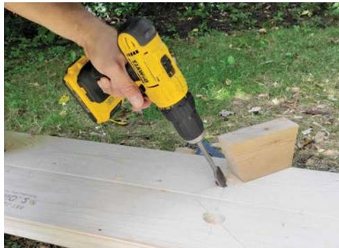
*Whether you drill with the brace or an electric drill, line your bit up with our 45° lines and then bring in the angle-block.*
