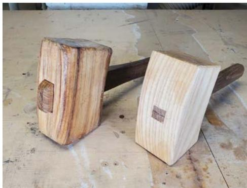
*Both of these traditional mallets have handles that extend all the way through the head. While this construction is very sturdy, it's also difficult to make.*
