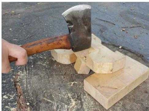
*One hard strike with the back of the hatchet should knock out your waste with no trouble, although you may need to use the knife to square up the bottom of the notch.*
