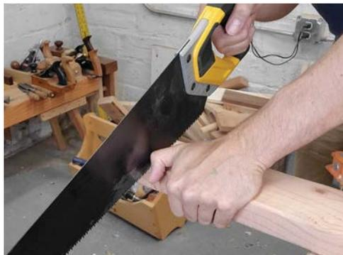
*Left: Grip your saw with your index finger pointed. This hand position will help you cut a straight line. Right: Press the knuckle of your left hand against the blade of the saw to keep you on track as you begin your cut.*
