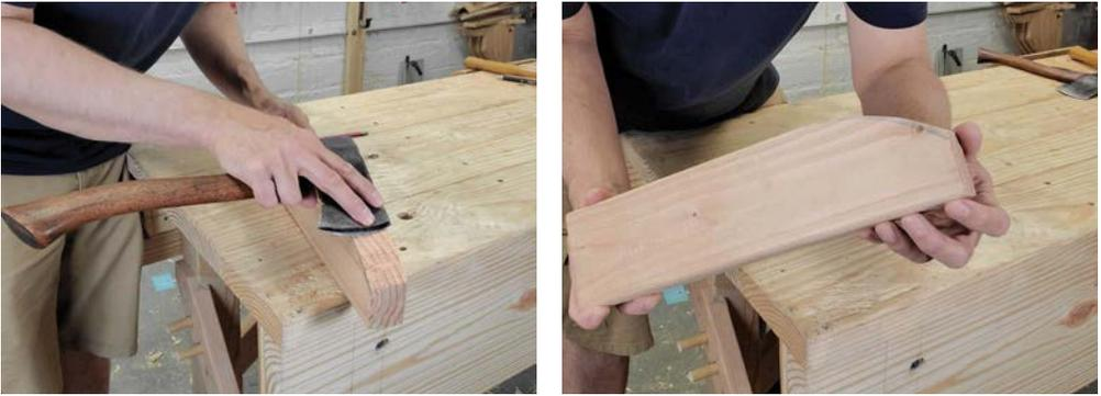
*Grip the head of the hatchet and use it to trim the rough surface left by chopping. Then refine the surface further with a sanding stick. Practice this technique; we'll be using it in our first projects.*
