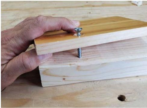
*Drop your screw into the clearance hole and then use the point to find the pilot hole. When you use the screw to line up your holes, you save a lot of fumbling around.*
