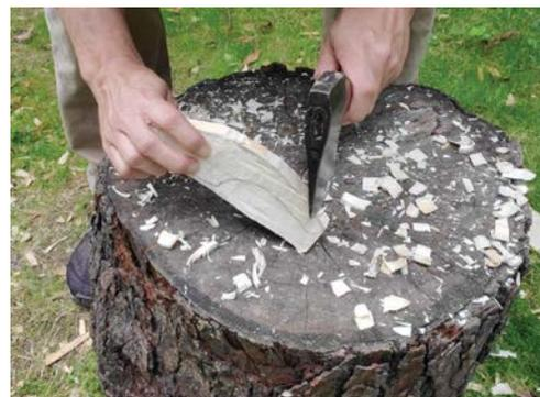
*To cut the outside curves, work from the middle to the tip. As you round each curve, keep the hatchet chops straight up and down and slowly rotate the work.*
