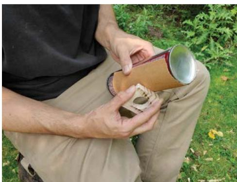
*Sandpaper wrapped around a spray can will add a scallop detail to the edge of this piece.*
