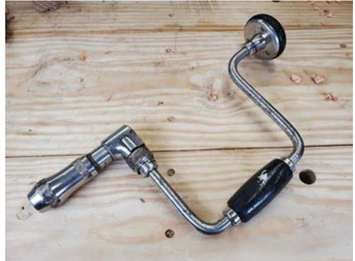
*This bit-brace might look like a silly old tool, but a good brace is a cheap way to drill most holes.*
