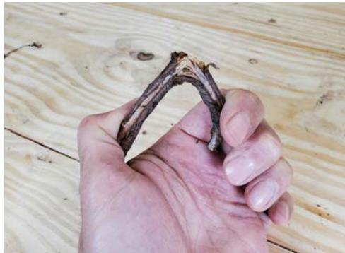
*This dead twig splinters instead of bending. Where it breaks, you can see the fibers that make up the wood.*
