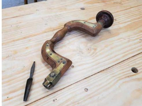
*This wooden "brace" and its hand-forged "bit" used to be standard equipment for drilling holes. For the drilling in this book, we'll use some updated tools.*
