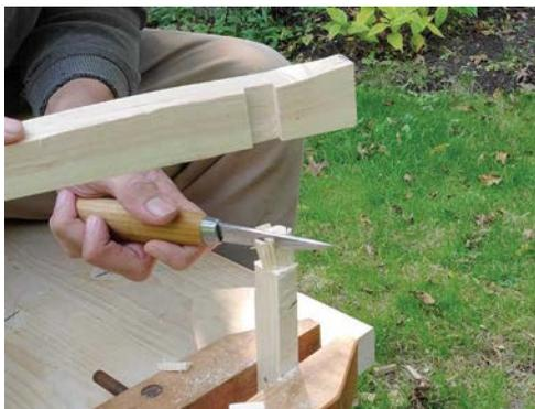
**Batoning:** Just like your hatchet, your knife can be used for controlled splits. Of course, your knife is much more delicate than a hatchet and can only be used to split small pieces. If I'm carving a small tenon (a little joint) on a delicate piece of stock, I'll saw my shoulders and then baton off the waste with my knife and a scrap of wood as the mallet. Remember to take small cuts and strike the spine of your knife gently.
