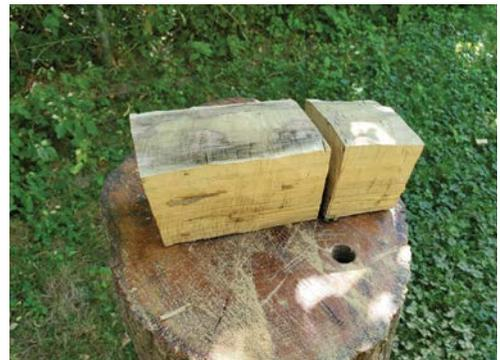
*I can use my chopping block with the clamp to hold my log while I saw it to length. In the finished piece, you can see the slight angle on the end. Both the striking faces should be angled this way.*
