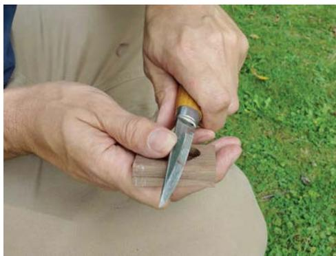
*I can easily bevel this edge with a push-cut.*
