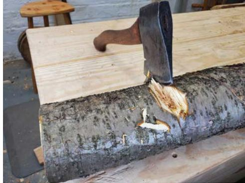
*I chopped into this log for over a minute and I've barely dented it. Axes are bad at cutting across the grain.*
