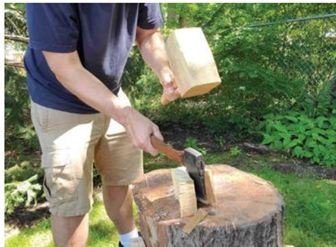
*A hatchet plus a mallet gives you both power and control for splitting. Instead of swinging the hatchet, you can place it anywhere on the work and then tap it with the mallet.*
