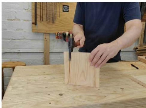
*Another safe and accurate way to split wood is to put the edge of your hatchet where you want the split and then keep it in contact with the wood as you lift them both and strike them against your work surface. Don't expect to make the split in a single hit. Make the split with several, controlled strikes.*
