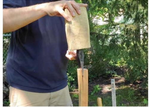
*My chopping block is a good surface for small cuts like sawing away extra length. My handle is also too thick, so I split it to width using my mallet head to drive the hatchet. Even without a handle, my mallet is already useful.*
