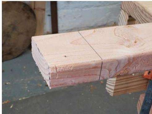
*A clear cutting line goes over the face and down the edge of your board. 2×4 stock is sold with the corners rounded off, so your line might not meet in the corner.*
