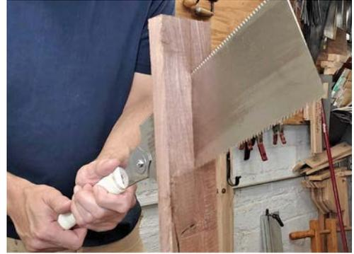
*I'd like to split this piece of wood in half, but the grain is not cooperating, and my split is crooked. If I rip the same piece of wood with the saw, my cuts stay straight no matter what the grain does.*
