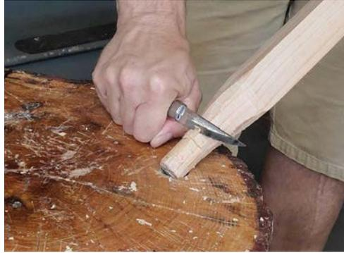
The hatchet and the knife will quickly turn your shoulder into a taper. A little sandpaper helps smooth the transition between the taper and the tenon.
