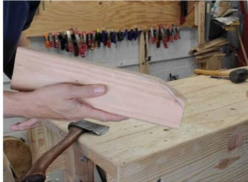
*Once you've chopped into the waste, strike down with your hatchet to shear off a layer of wood. Repeat this chopping and shearing until you've removed most of the waste.*
