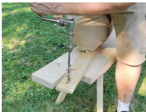
*Drilling on this bench is a lot like sawing. Hold the work with your body weight and bear down on the drill.*
