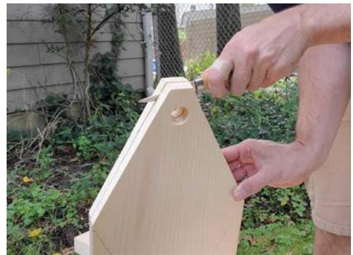
*With your two ends stuck together, it’s easy to cut the details onto both pieces at once. When you’re done, use the knife and the hatchet to slowly force the pieces apart.*
