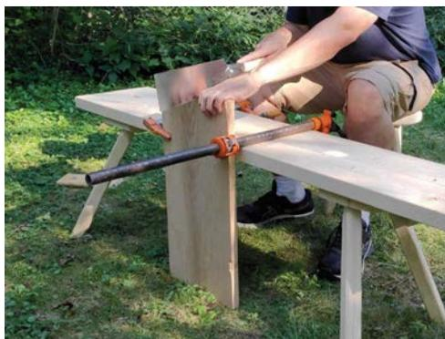
*You can hold wide boards against the edge of your bench by adding one more long clamp. In the picture, I've clamped my work to the far side of the bench so that my pull-saw can work effectively.*
