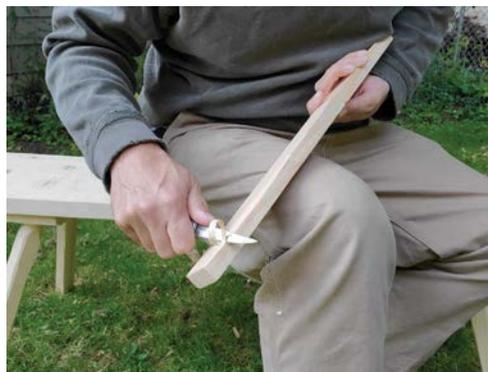
against the spine and skew the blade so the tip points toward you a little. Push forward with a slow, controlled cut, moving the work along the edge toward the point as you cut. Try to take one long, very thin cut all the way along the board edge. If you'd like a wider bevel on your stock, take several light passes, rather than one heavy cut.
