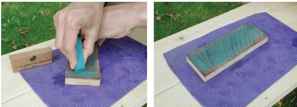
*To make my strop, I glued a piece of old leather to a piece of MDF (a cheap particleboard) that's very flat. Then I colored it in with green buffing compound.*
