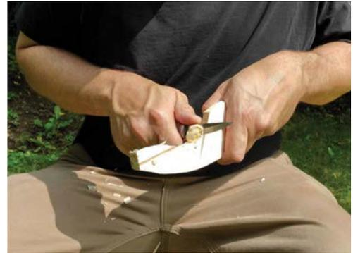
*To finish the tight curve, I work into the stop-cut from both directions with a controlled push-cut. Notice that I'm peeling away thin slices and always keeping my left hand behind the knife.*
