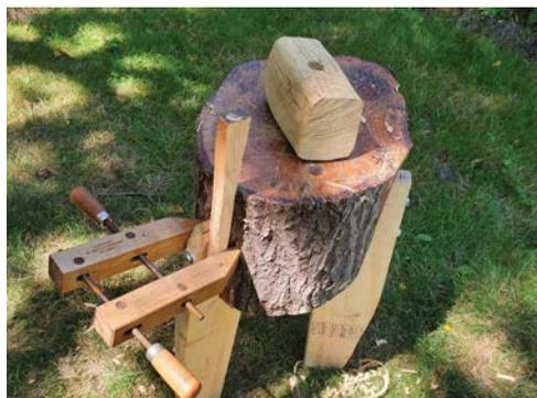
*After I drill a hole in the bottom of my mallet, I can clamp the handle-stock to the chopping block and carve the tenon on the end.*
