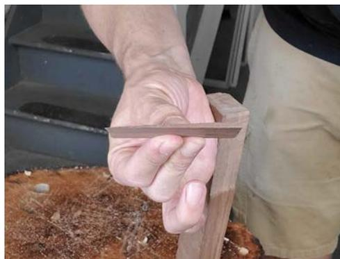
*I sawed this wedge from a scrap of walnut. It tapers to a featheredge and is much longer than I need. I'll be able to drive this wedge deeply into the joint.*
