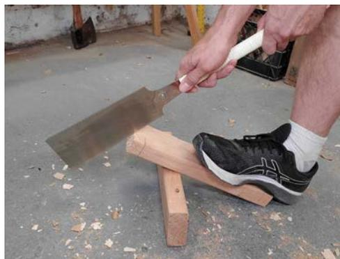
*Using a scrap of wood as a sawhorse lets me stand on the wood and still see it clearly. I start my cut with the fine crosscut teeth, and then switch to the big rip teeth and a powerful, two-handed grip. With this stance, ripping is easier.*
