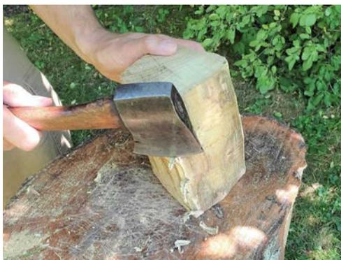
*I'm not going to leave any sharp edges on my mallet head. I'll use the hatchet to trim the edges and then a sanding stick around the faces. The final tool needs to be comfortable and resist splintering.*
