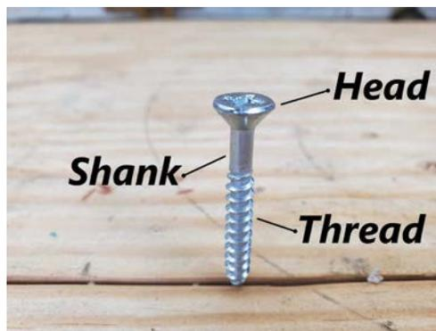
*Anatomy of a wood screw. Each part of a screw plays a role in connecting pieces of wood.*
