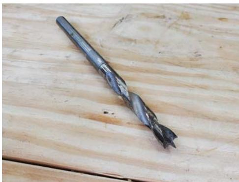
*Brad point bits are designed for wood. Like an auger, they have a sharp point and nickers that slice the wood.*
