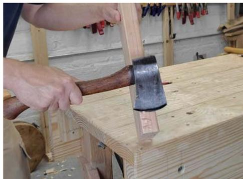
*Trace a curve across the corner of a piece of wood and then remove everything outside the curve. Start with a series of light chops to weaken the fibers.*
