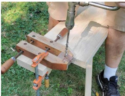
*Your two clamps can work together to hold small pieces for drilling and carving.*
