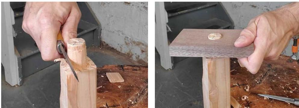
*Trim carefully with your knife, taking very thin shavings. At this stage, little changes make a big difference. After several rounds of trimming and fitting, your test-board should slide all the way to the shoulder.*
