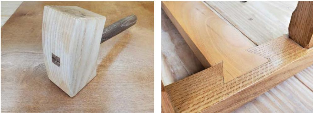
*Two joints. On the left mallet with the head and handle joined in **mortise-and-tenon** with a wedge for added holding power. On the right is a simple **dovetail**. The angled sides of this joint help hold it in place, but it still needs a bit of glue.*
