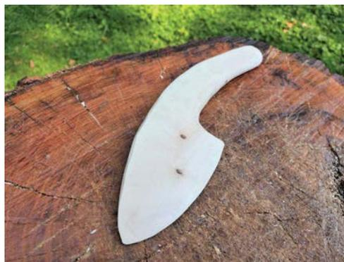
*You need to let the wet wood dry before you can get the final finish. After a little sanding, the butter knife is ready for an oil finish.*
