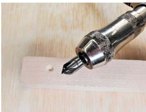
*The countersink is a simple tool that works in a drill or a brace. Cut your countersink before you drill your holes and you're guaranteed to get a smoother result.*
