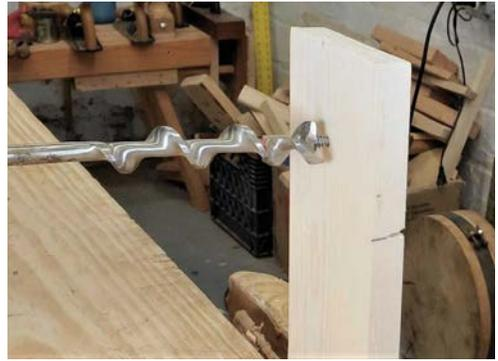
*To prevent blowing out the far side of your hole, drill until the point of your bit pokes through, then flip the board around, put the bit into the hole, and finish drilling. The finished hole will be clean on both sides.*
