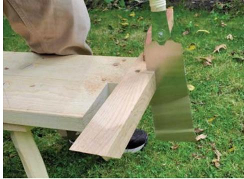
*To saw out my notch, I remember the “triangles” rule from Chapter 7. I saw the lines I can see, flip the piece, and saw the lines on the other side. I finish up by bringing the saw perpendicular and sawing the final triangle hidden inside.*
