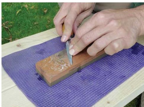
*After you've sharpened the first section of blade, move the knife over and sharpen the next section. I can usually sharpen this knife in three sections. As you get near the curved tip, you probably want to skew the blade to put more of the bevel in contact with the stone.*
