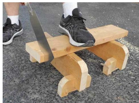
*For crosscuts, you can kneel on the work and have both hands to start the saw right on the line. Once your cut is established, stand with one foot on the work and use two hands on the saw.*
