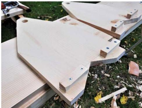
*The cleats installed on the ends. Note that I've struck a pencil line at the point of the lower triangle and used it to align my cleats. This placement will also keep my cleats from being visible on the finished tote.*
