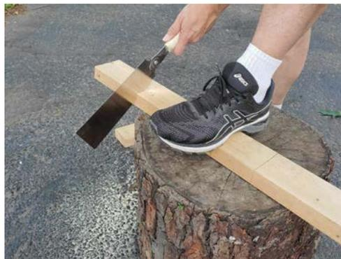
*Once I've started my cut, I hold the wood with one foot and grip the saw with two hands for long, powerful strokes. Notice how I'm sawing both the face and edge of the board at once. With my saw following both lines, I'm much more likely to get a square edge.*
