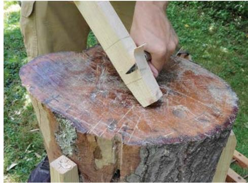
*Ripping at a slight angle will start your taper. Follow up with the knife and you can “plane” off the saw marks and get a smooth surface.*
