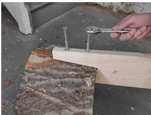
*Run your screws in with an adjustable wrench (or a socket wrench if you have one). Get them good and tight. If you try to tighten them later, the screws are likely to snap.*
