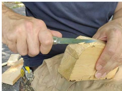
*The corners can be quickly shaped with the hatchet and knife. When I use the hatchet, the hand holding the work is far away from the cut. When I refine the curve with the knife, I work off the side of my lap where a slip of the blade can't cut me.*
