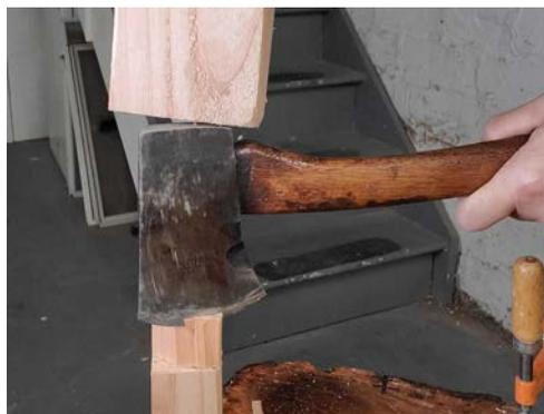
*You can use your hatchet to split most of the waste off your tenon. A piece of 2×4 makes a good mallet. Notice how the stop-cuts keep the splits from traveling too far down the leg.*
