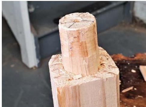
*Drill a hole in a scrap of hardwood and use it to test your tenon. At first, the tenon won't fit at all. Trim a little with your knife and try again. Once your test board slides on a little bit, you'll be able to see crushed, shiny fibers and a little ridge where the test-board stopped. These signs will tell you where to trim.*
