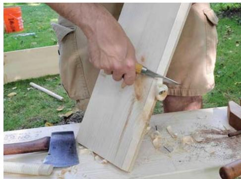
*You can lay out your bevel by letting the nail and knuckle of your middle finger ride against the edge while you hold your pencil at the distance you want. This simple technique is surprisingly accurate. After most of your waste is chopped away, finish up with a planing cut from the carving knife.*
