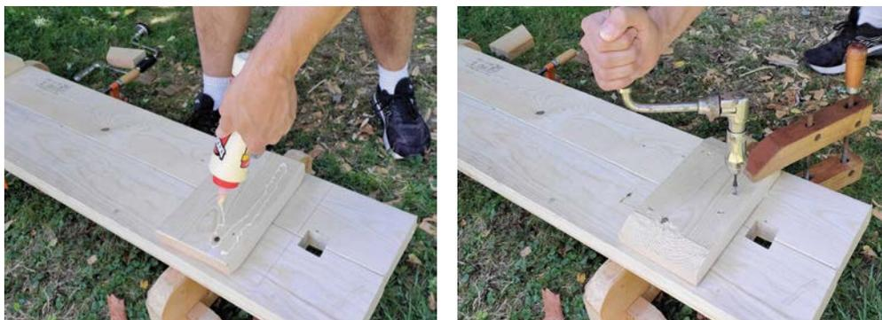
*Install your battens with screws and your brace. A little wood glue can't hurt. In the picture, I just put 4 screws in each batten. That way, I know my drill won't hit a screw on the way through. After the leg-holes are drilled, you can add the other screws.*
