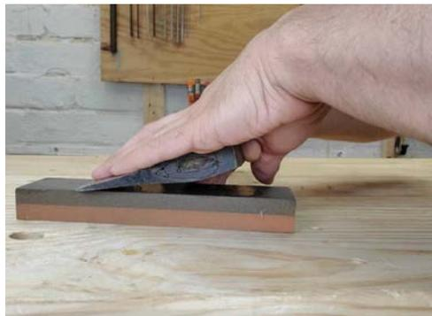
*Your basic sharpening stroke starts with the tool up on its edge at about a 25° angle. As you push forward along the stone, slowly rock the tool back so that you transition from the edge to the bevel. At the end of your stroke, the edge is off the stone and you are only working the bevel.*
