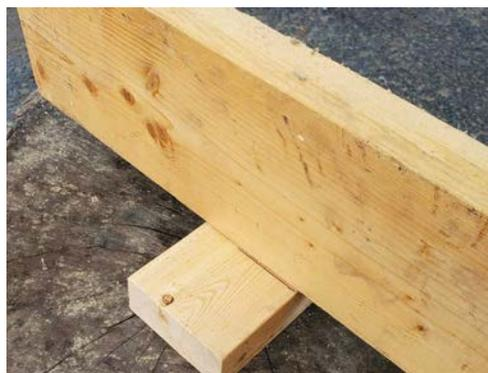
*To get my center notch dead on, I mark one side and then lay a piece of 2×6 along my line and trace the other side. By marking the exact width of my stock, I'm guaranteed a tight fit when I attach the feet to the beam.*
