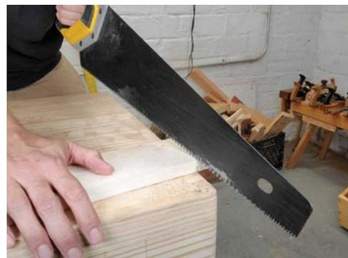
*Flip your square so that the lip rests against the face of the board and you can use the edge to strike a line that meets your first line. These two lines meet at a perfect right angle and are very useful for guiding your saw through a cut.*
