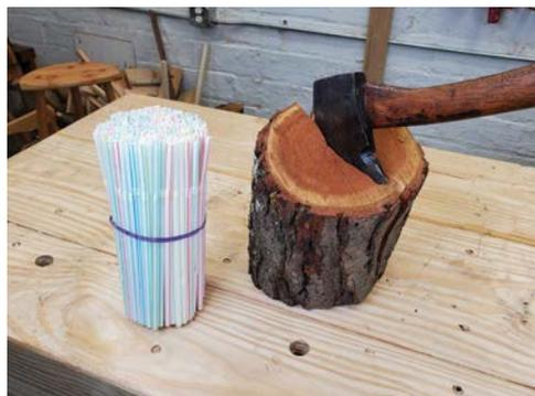
*The bond between wood fibers is pretty weak. By chopping down into the end grain, the hatchet slid between the fibers and easily split this log in half.*
