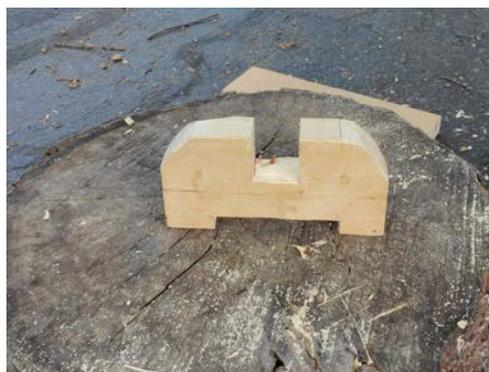
*My foot is roughed out, but the top notch has a splintery bottom and the walls need to be widened to fit the beam. The knife and sanding stick can handle these tasks.*
