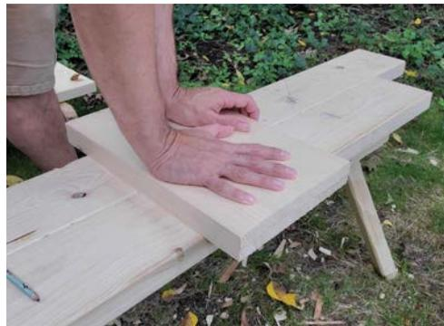
*Put pieces of tape on both your ends and add a line of superglue on the tape. When you press the ends together, the glue will stick the boards together, but because it's only on the tape, you'll be able to separate the parts later.*
