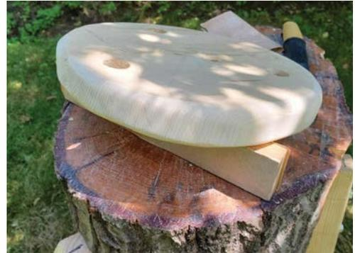
*My knife quickly slices a bevel around the edge of my seat. Notice that I've sketched a line about  $\frac{1}{2}$ " (13 mm) inside the rim. I did this line by eye, but it will keep my bevel consistent. After I carve away the waste, I can round the bevel over with the sanding stick and some sandpaper held in my hand.*
