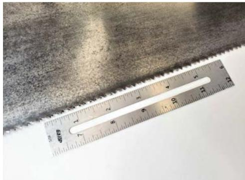
*Saw teeth close up. At six teeth per inch, this saw is a fast, coarse tool.*
