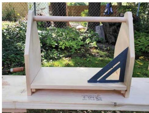
*With the dowel in its holes and the bottom resting on the cleats, I can use my speed square to make sure the ends are square to the bottom.*
