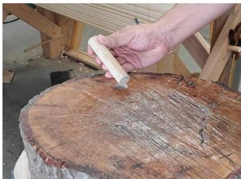
*After adjusting your hole, your clamp should slide in and stay in place with friction. Once it's done, drill a hole (or two) in the top of your log to accept a peg. The clamp will hold work down and the peg will keep it from rotating.*
