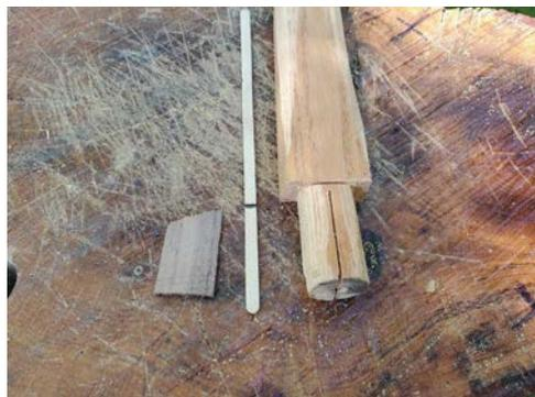
*Any stick of wood will make a depth gauge for finding the length of your tenon and your wedge. Both of these must be **less** than the depth of your mortise.*
