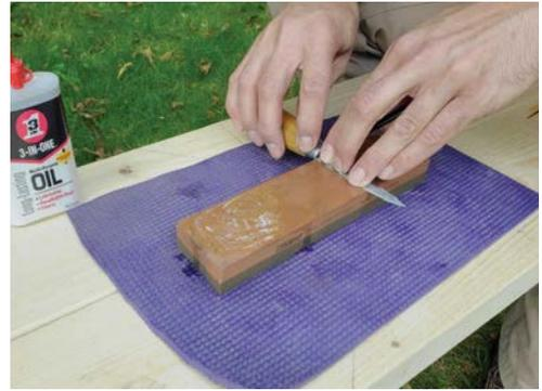
*Coat your stone evenly with oil and begin sharpening at the base of the blade. Remember to lay that bevel flat on the stone and keep it there.*
