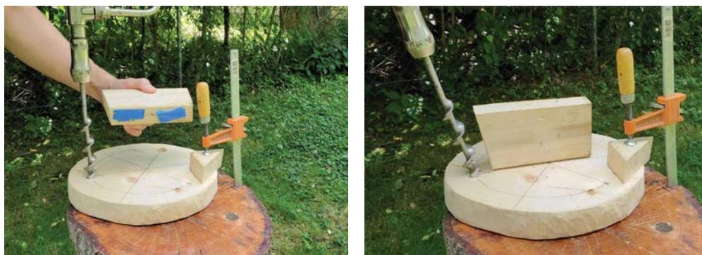
*Begin drilling along your sight line with your drill held straight up and down. When the hole is started, add your guide block to give you the correct angle.*
