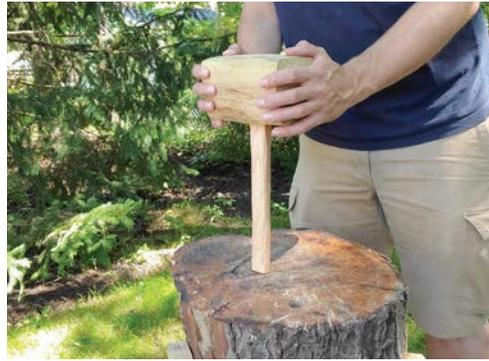
*Before I assemble the mallet, I coat all the surfaces with glue and insert my wedge. Then I put the handle in the head, make sure it's turned the right way, and start tapping it against my block. As I drive the handle in, it tightens.*
