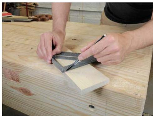
*Hold the lip of your square against the side of a board and strike a line across the edge. Your line will be perfectly square to the edge of the board. Saw along the line, and your cut will be square.*
