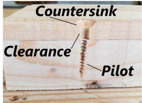
I installed this screw and then cut the wood in half to show what happens inside. Note how the three holes each work differently. The threads bite deeply into the **pilot hole**. The **clearance hole** doesn't even touch the screw shank. The **countersink** cradles the screwhead and allows it to pull against the threads.
