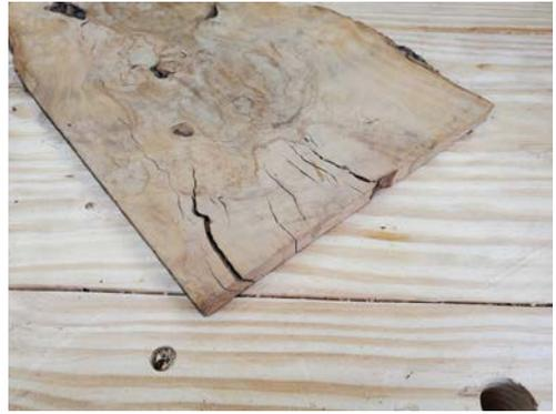
*The deep cracks at the edge of this board show that it was dried too quickly, and the wood fibers split apart from the stress. Wood that's dried carefully won't split.*
