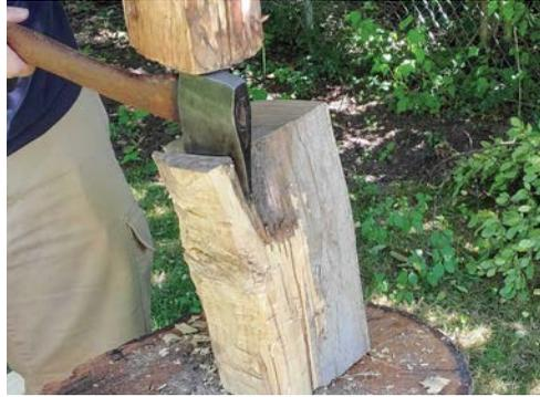
*To trim the stock for the head, I'm putting the edge of my hatchet where I want a split and hitting the back with another piece of firewood. This approach gives me both control and power, and the log is quickly trimmed.*
