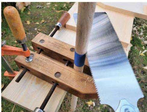
*A piece of tape wrapped around a dowel makes it easy to get a square cut. Just follow the edge of the tape.*
