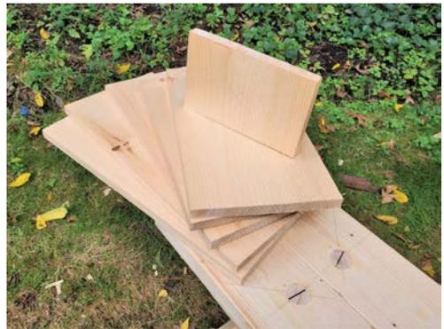
*Crosscut all your components from the plans. The little piece sitting on top of the stack will be cut up to make some details later in the project.*
