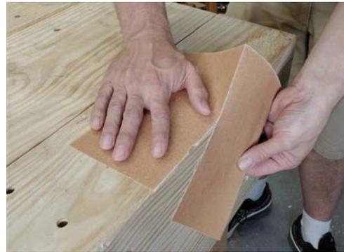
*Sandpaper is difficult to cut but it's easy to tear. Fold it over and use a pencil to make a sharp crease, then use the edge of a table to support the fold while you tear. You'll quickly learn how to get a clean and straight line.*
