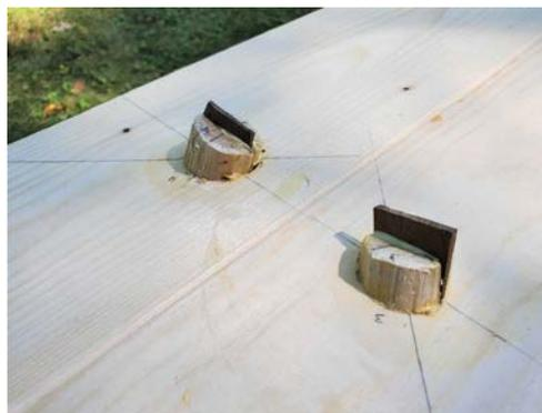
*Well-made wedges can be driven firmly and will stop moving before the wedge is buried in the tenon. If your wedges are disappearing into the leg, try cutting thicker wedges with a steeper taper.*
