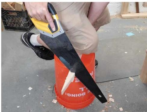
*A plastic bucket can make a good platform for sawing. Use the weight of your body to keep the wood steady as you saw it free.*
