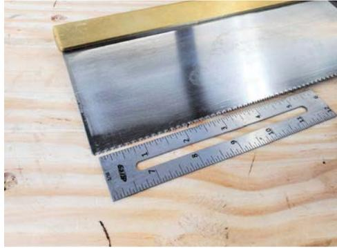
*A small, fine saw cuts a narrow kerf and leaves a smooth surface. This saw has 13 teeth per inch. It's great for detail work, but it's too slow to use for cutting up big boards.*
