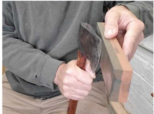
*You can also sharpen with the hatchet on your knee. Hold the tool steady and move the stone in circles up and down the bevel.*
