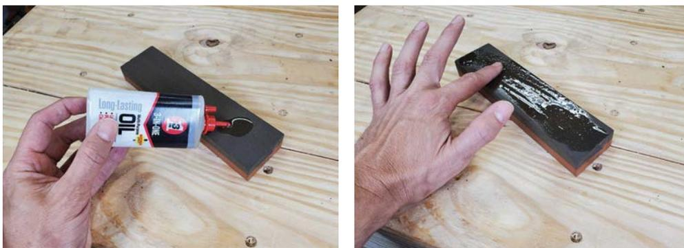
*Your sharpening stone should be evenly coated with oil. As you use the stone, little particles of metal will come off your tool. The oil will keep these particles out of the stone. Be sure to wipe off the used oil every time you use it.*
