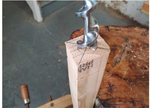
*You can screw-clamp the leg to your chopping block and have free access to the end. Once you've found the center of your stock, drill down to score a circle in the end.*
