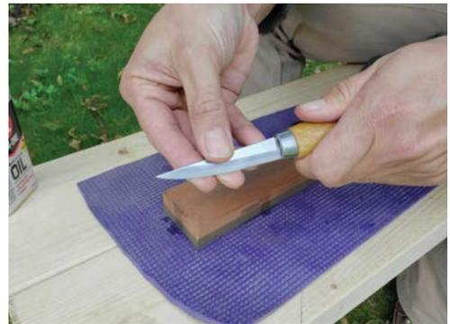
*On the left, you can see that the first 1/3 of the blade is covered in fine scratches all the way to the edge. On the right, I'm pushing my fingertips across the edge from the underside. As my skin moves over the edge, I should feel the burr.*
