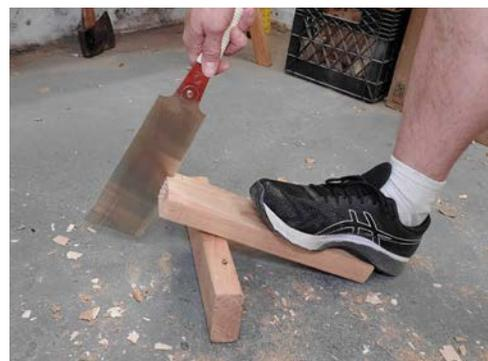
*I only sawed the lines I could see, so now I need to flip this board over and finish the rip from the other side. Once I rip down the other side, there will still be a little "triangle" of wood at the base of the cut. I lift my arms so the saw is perpendicular to the wood and finish the cut square.*
