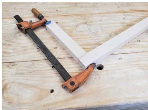
*These two pieces can be connected with a “butt joint.” A little glue and clamping pressure will make them stick together.*
