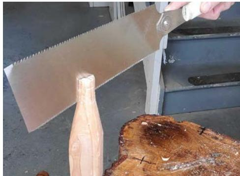
Mark your tenon perpendicular to the grain of your seat-board and then saw down that line.
