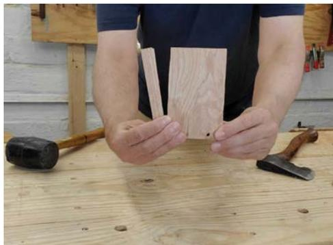
*By placing the edge of my hatchet exactly where I want to split the wood and then striking it with a rubber mallet, I get to choose exactly where the wood splits. This technique is safe to use, even on small pieces of wood.*
