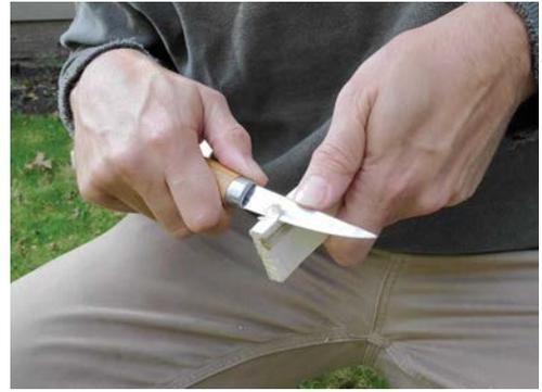
**Thumb Push Cut:** This is a detail cut for removing small amounts of wood. Hold the work in your left hand with your thumb extended. Place the knife against the wood and use your left thumb to push the blade forward. Alternately, you can lock your thumb in place and lever the back of the knife around the tip of your thumb. Both of these cuts offer excellent control and added leverage if you need to cut deeply. I often use this cut when working into a tight curve.
