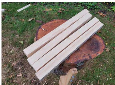
*To lay out your legs, use the edge of a board. I ripped piece C into six legs and then picked out the best four. The two legs I'm not using can be cut up to make three small battens.*
