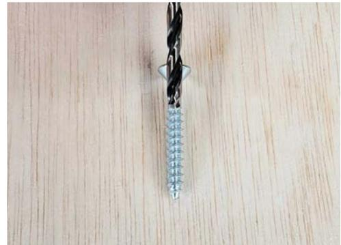
Finding your drill bits is easy. The pilot-hole bit should let the screw threads show on both sides. The clearance-hole bit should be slightly larger than the screw-shank.
