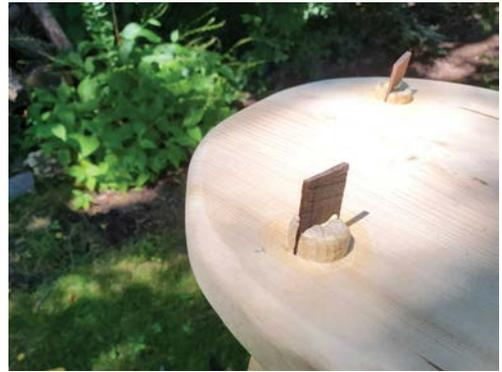
*A well-seated wedge looks like this. Notice that there's a lot of wedge sticking out of the tenon. Cut your wedges long and give them a very gradual taper. You want to stop hitting the wedge when it stops moving, not when you run out of wedge to hit.*
