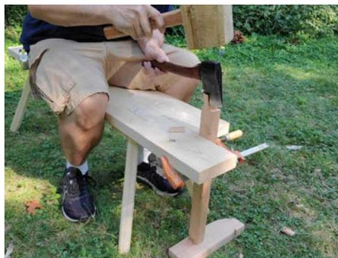
*The little corner on the end of your bench makes a great place to clamp narrow stock. In this picture, I put a scrap under my stock to keep it from sinking into the ground as I hit it.*
