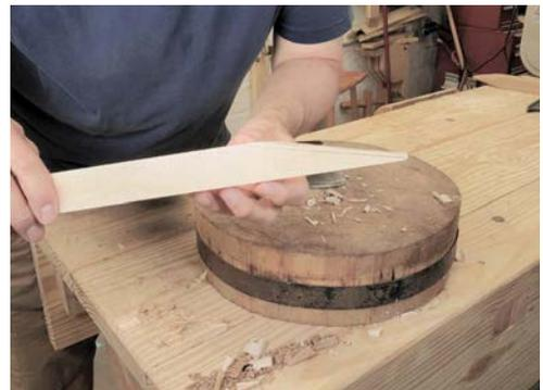
*As I shape my wedge, I'll peel off layers of wood until I'm close to my line, then I can flatten my surface with the hatchet or with a sanding stick.*
