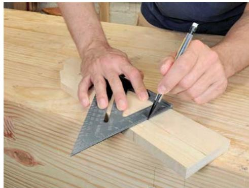
*By holding my pencil against the ruler and dragging the square, I can draw a parallel line any distance from the board's edge.*
