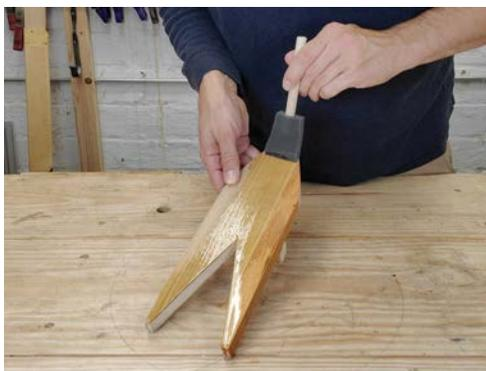
*The bootjack will see hard use, so I'm finishing it with oil-based poly. I've thinned the finish with mineral spirits so I can use a foam brush.*
