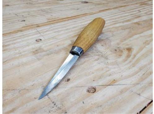
The **Mora Sloyd Knife** has a very wide bevel to give you lots of control. The handle is comfortable, and the knife comes with a sheath. You don't have to buy this model. Any small, slightly curved knife with a wide bevel will work. (Many tool makers refer to this bevel style as a "Scandi grind" so that's what to look for.)
