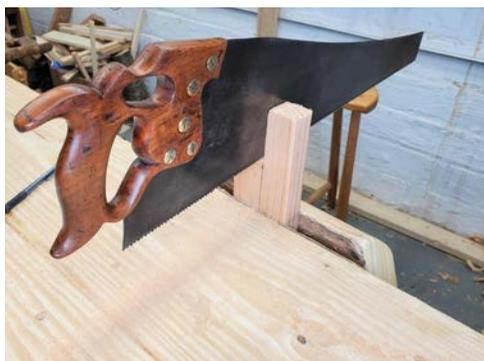
*On the left, I’m crosscutting a board to make it shorter. On the right, I’m ripping a board to make it narrower. I’m using a different saw for each cut and these saws are each designed for one kind of cutting.*
