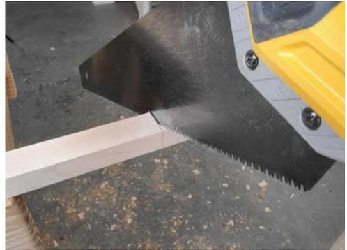
*When you saw a piece of wood, you turn some of it into sawdust. I saved this board in half, but the left-hand piece is a little bit longer because of the kerf.*
