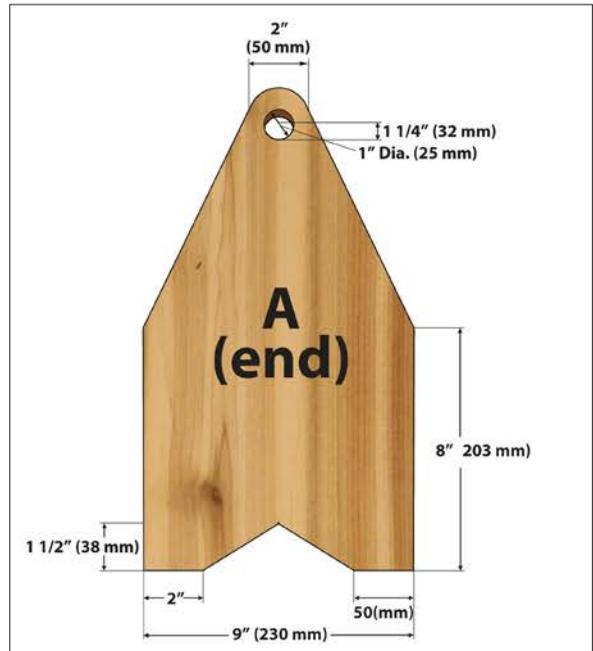
Most of this project is cutting and shaping the ends (A), since they have most of the details. To end up with two identical pieces, it's helpful to fix them together and work on both at the same time. Stick a few pieces of masking tape or blue painter's tape to your ends, dab on a little superglue and press the ends together for 30 seconds. The glue will fix your pieces tightly together, but the tape will make it easy to get them apart without damaging the wood.
