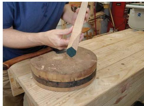
*Use the techniques from the last chapter to chop and peel one corner off the stick. Try to leave a flat and even surface. Take off all four corners and you'll be left with a hexagon.*
