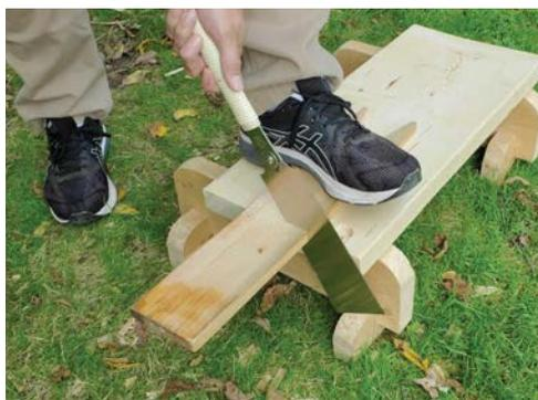
*Use the rip teeth on your Ryoba to cut out the V-notch. Stand on your work to hold it steady. This is where using a long piece of stock comes in handy. After the notch is done, crosscut to final length.*
