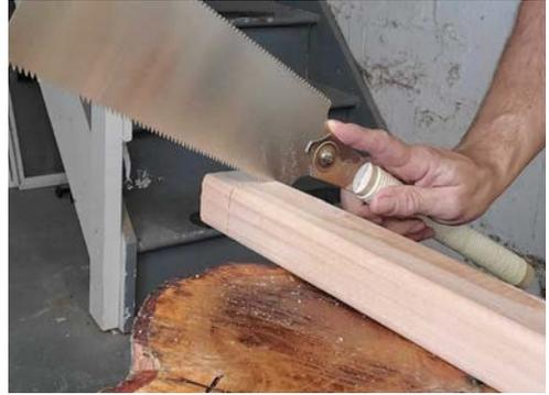
*I've drawn a **shoulder line** on the end of my leg and now I'm sawing that line all around the leg. This creates a stop-cut like we used in Chapter 5.*
