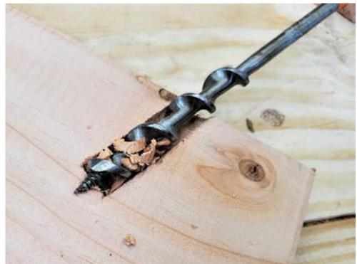
*If we look inside the wood, we can see the auger bit working. The snail pierces the wood and guides the bit. The lips break up the wood. The flutes carry the chips out of the hole.*
