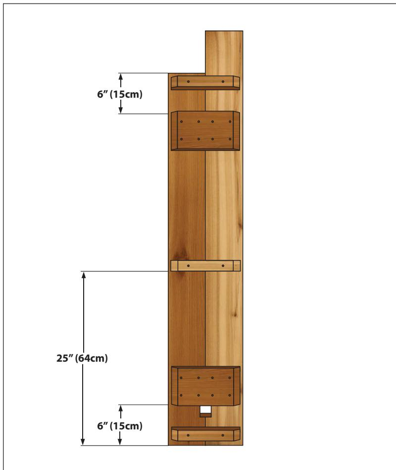
*My large battens are screwed to the bench 6" (15 cm) from either end. After the legs are installed, you can add the smaller battens in the middle of the bench and close to the bench ends.*
