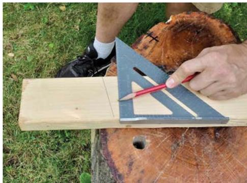
*You can use your speed square to easily lay out an angled line. Cut along this line and you have a 15° angle guide.*
