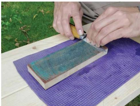
*Place your blade with the bevel flat on the strop and pull it toward you with firm downward pressure. Repeat. In the picture, you can see the middle of my strop getting dark as it rubs steel off the knife.*
