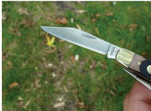
*The carving knife on the left has a single, wide bevel that's great for woodworking. The pocketknife on the right has a narrow secondary bevel. It cuts, but it's hard to control.*
