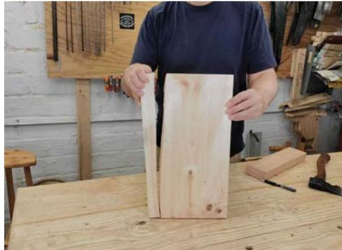
*Instead of sawing the edge off this board, I can split it off with a hatchet. Notice that my hand is far away from the split and my fingers are well out of danger. I only use this technique with a wide board so that I can hold it safely.*
