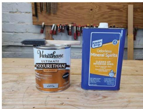
*Oil-based polyurethane can be used straight from the can, but I thin it with mineral spirits.*
