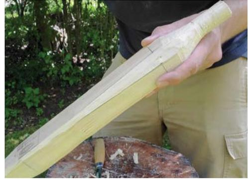
*To make tapering the upper leg easier, I've drawn some lines along each corner. Notice that my lines are wider at the top of the leg. I can easily remove the waste with my knife and follow up with a sanding stick.*
