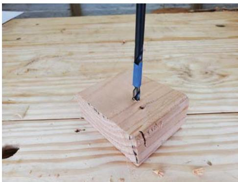
*The tape on this bit tells me exactly when to stop drilling.*
