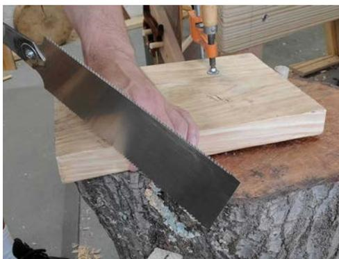
*With a clamp and a peg you can hold wood still for sawing or chopping.*
