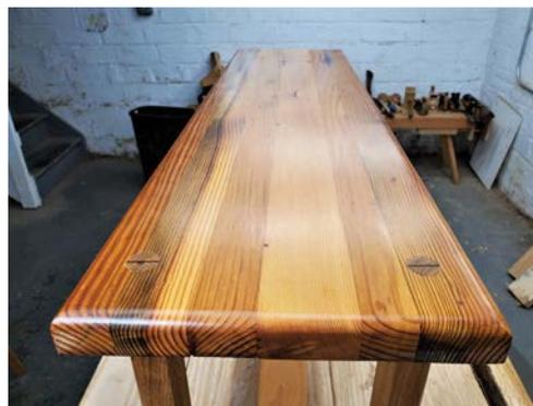
*This benchtop is made with many thin boards laminated together. The wide glue surfaces and long-grain connections make these joints strong and durable.*
