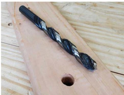
*Twist bits are simple, cheap and effective, but they're not designed for wood. Larger bits might tear the fibers a little. Notice the ragged edges on this hole.*
