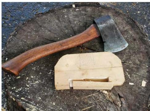
*To split out the waste, I start with the upper corner of my hatchet and strike firmly with a scrap of wood. This construction lumber is soft, so the edge should plunge right in. After I've worked along both sides of my line, the waste comes right out.*
