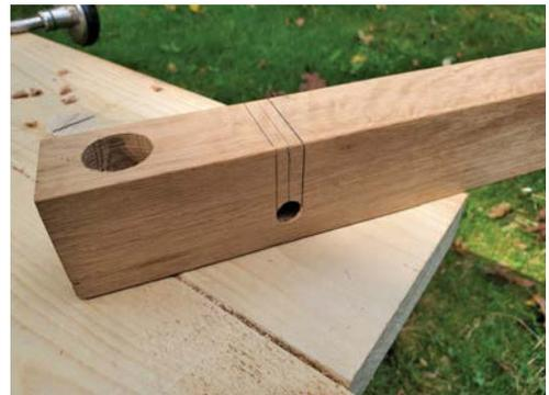
*To make a slot, start by drilling a hole. Then use your square to strike lines from the edges of the hole and carry them around the side and onto the opposite face.*
