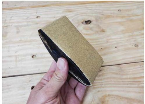
*This commercial rubber sanding block grips the paper securely and makes it easy to sand large surfaces with the paper held flat.*
