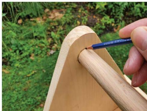
*When you have the sides square to the bottom, trace around the handle where it enters the sides. The lines on the handle will let you get it back in position fast during glue-up.*
