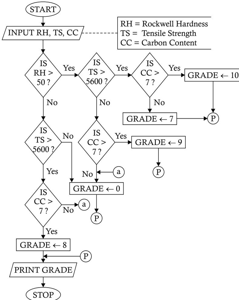
**Task Analysis.** We must determine the grade of the steel on the basis of the values of three characteristics, namely, the Rockwell hardness, carbon content, and tensile strength. The values of these three features are the input.
