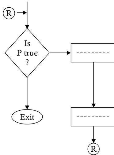
For a post-test iteration, the predicate is tested after performing a set of operations once to decide whether to repeat the set of operations or to terminate the repetition. If the condition happens to be true, then the set of operations is repeated; otherwise, it is not repeated. The diagrammatic structure of this logic is as follows.
