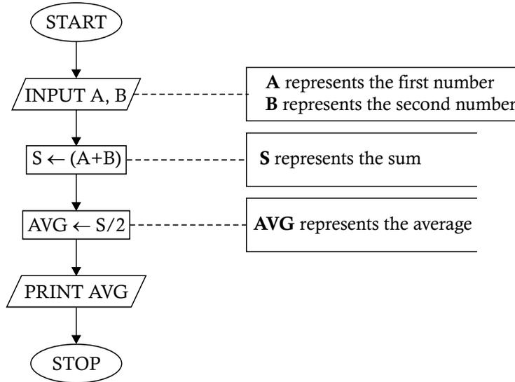
**Task Analysis.** From the concept of determining the average of two given numbers, we know that the given numbers must be added together to obtain the sum first; the sum is then divided by 2 to obtain the average. The flowchart for Problem 1.2 illustrates this idea.
