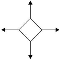
*Decision:* used to show any point in the process where a decision must be made to determine further action
