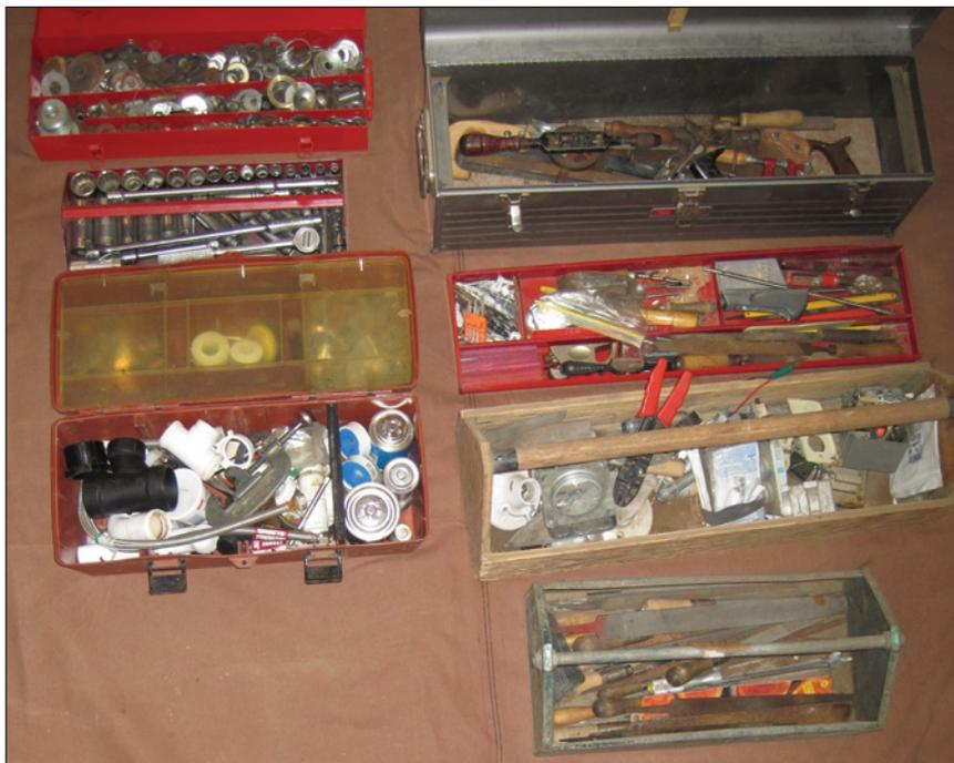
*Left: Red metal box contains assortment of washers; red tray holds socket set; plastic box contains plumbing tools, adhesive and supplies. Right: Grey metal toolbox and red tray contain carpentry hand tools; wooden tray holds electrical parts and tools; metal tray is full of files.*
