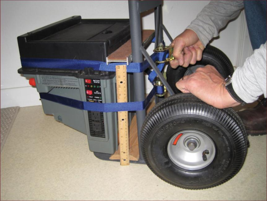
*Tightening blue nylon ratchet straps securing generator case to hand truck frame. Note padded aluminum base for photovoltaic panel. Ruler shows scale.*
