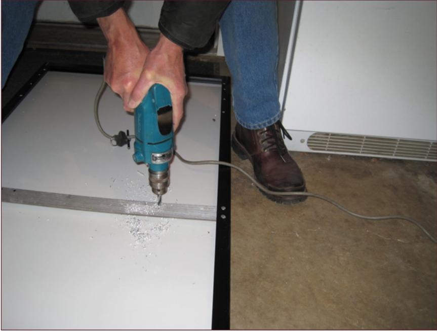
***Drilling holes in horizontal support to receive U-bolts that fasten photovoltaic panel to hand truck frame.***
