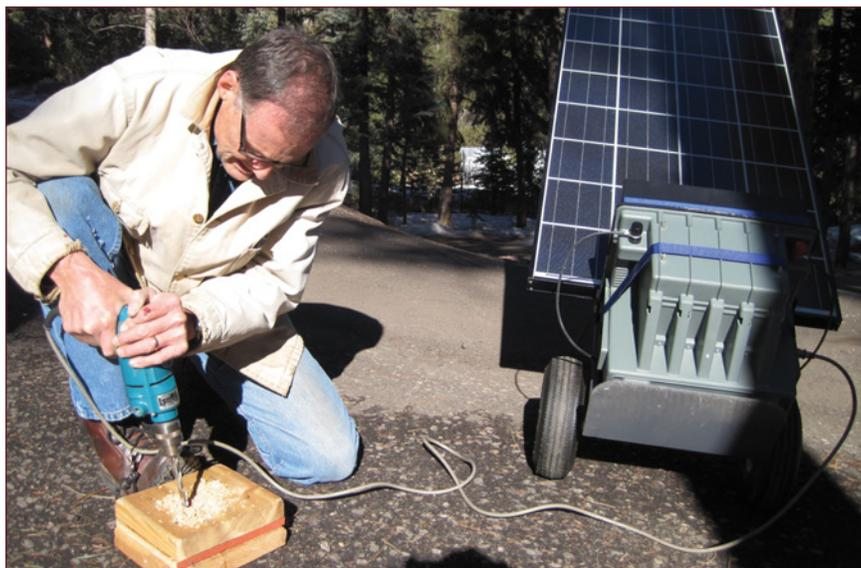
*Using a heavy-duty drill in the field. System is leaning on stand to maximize sunlight on PV panel.*
