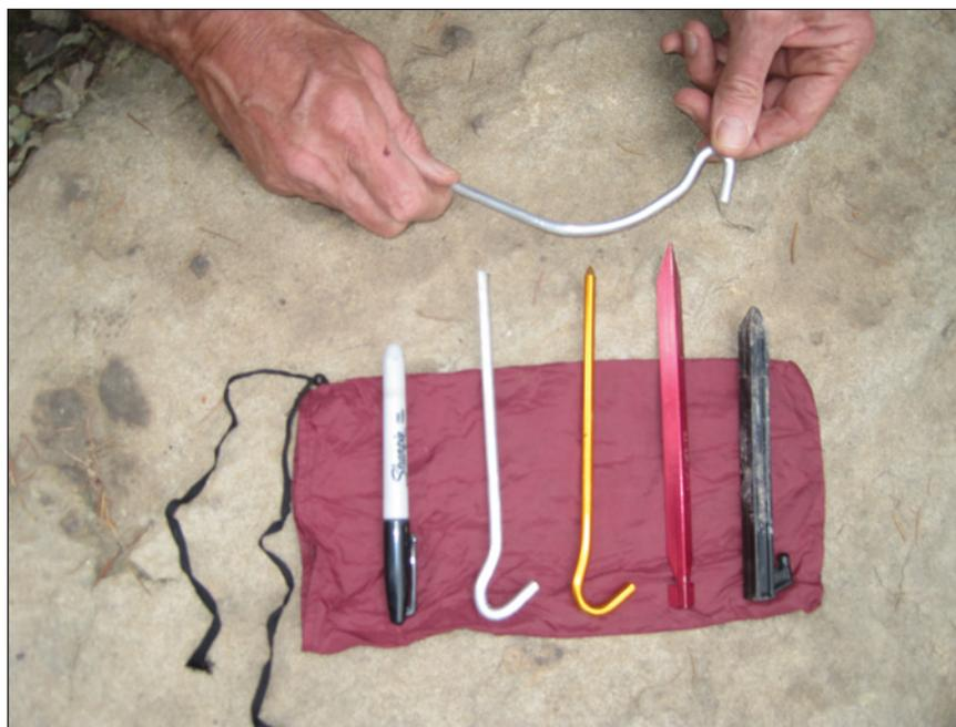
***Tent pegs come in a variety of shapes and materials. The bent peg was made from inexpensive aluminum. Marker shows scale.***
