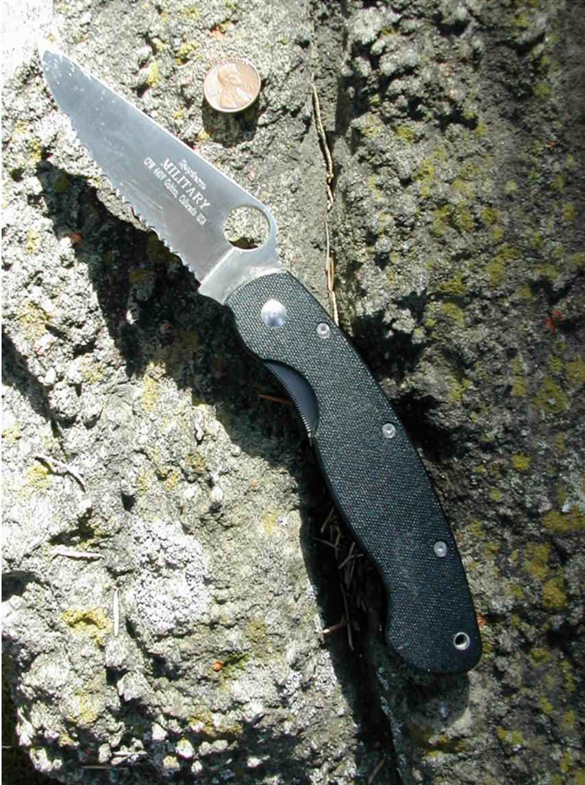
*Spyderco military model features blade of CPM (crucible particle metallurgy) 440V, a tough stainless steel. The black scales are G-10.*
