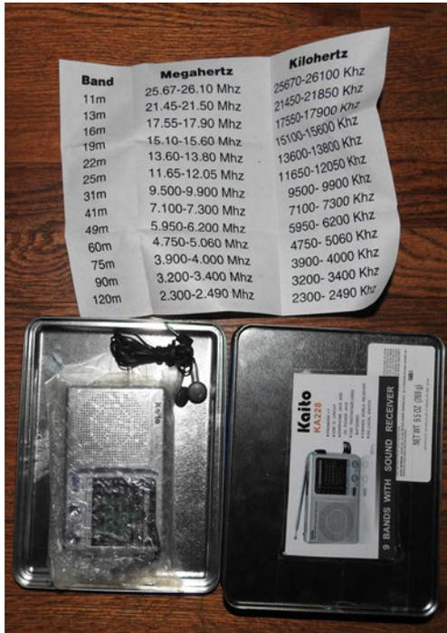
***This \$10 shortwave receiver, shown here in an EMP-proof Faraday Shield made from a Christmas candy tin, runs for days on two rechargeable AA batteries, and is beyond value in a far-reaching catastrophe.***
