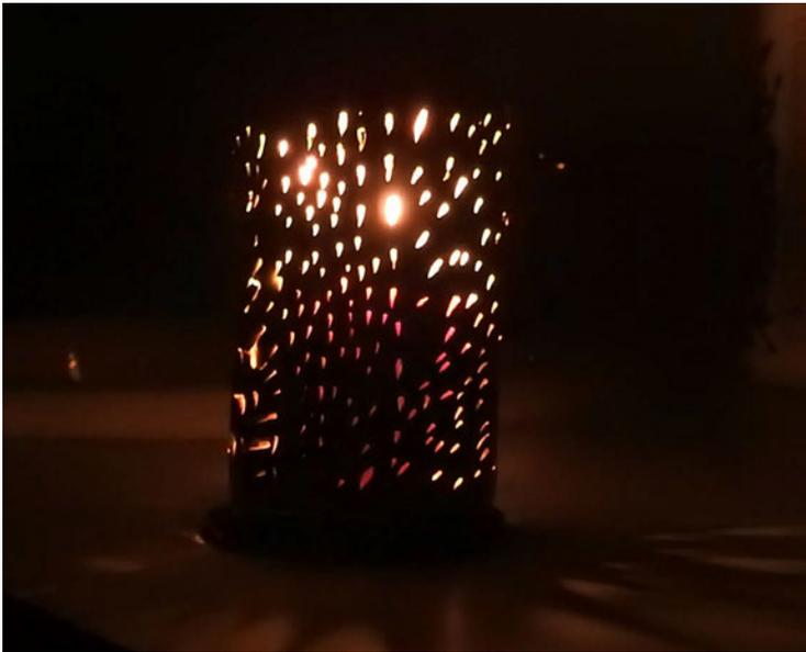
*Made from a soda-pop can, this punched-tin lantern approximates those dating back hundreds of years, turning a candle into a wind- and rain-resistant all-weather lantern—just be careful not to burn yourself on the hot can.*
