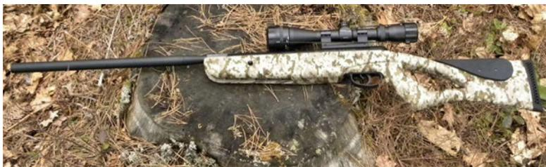
***This .177-caliber Remington air rifle fires a pellet faster than the speed of sound, holds a steady pressure in its cylinder for long periods of time, and possesses the accuracy to drive nails at 25 yards.***
