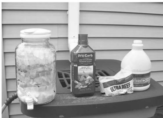
Homemade filter using alternating layers of sand and activated charcoal separated by coffee filters. After filtration, use bleach for biological decontamination of rainwater from the roof.
