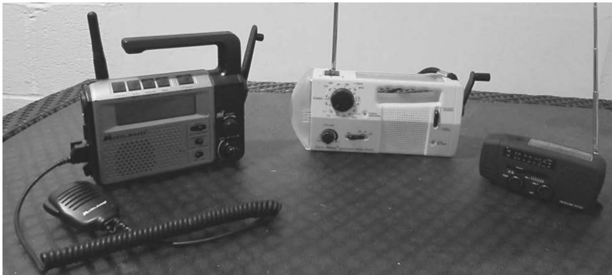
Emergency radios come in many forms. The one on the left is crank and battery powered, and has the capacity to transmit on the GMRS/FRS wavelengths. The center one has a light and a siren, and is crank and solar powered. The small radio on the right has a crank and solar power system, and can even be used to recharge your cell phone.
