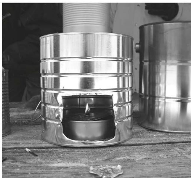
While the homemade hobo stove shown here uses alcohol, it can use twigs or candles as well.
