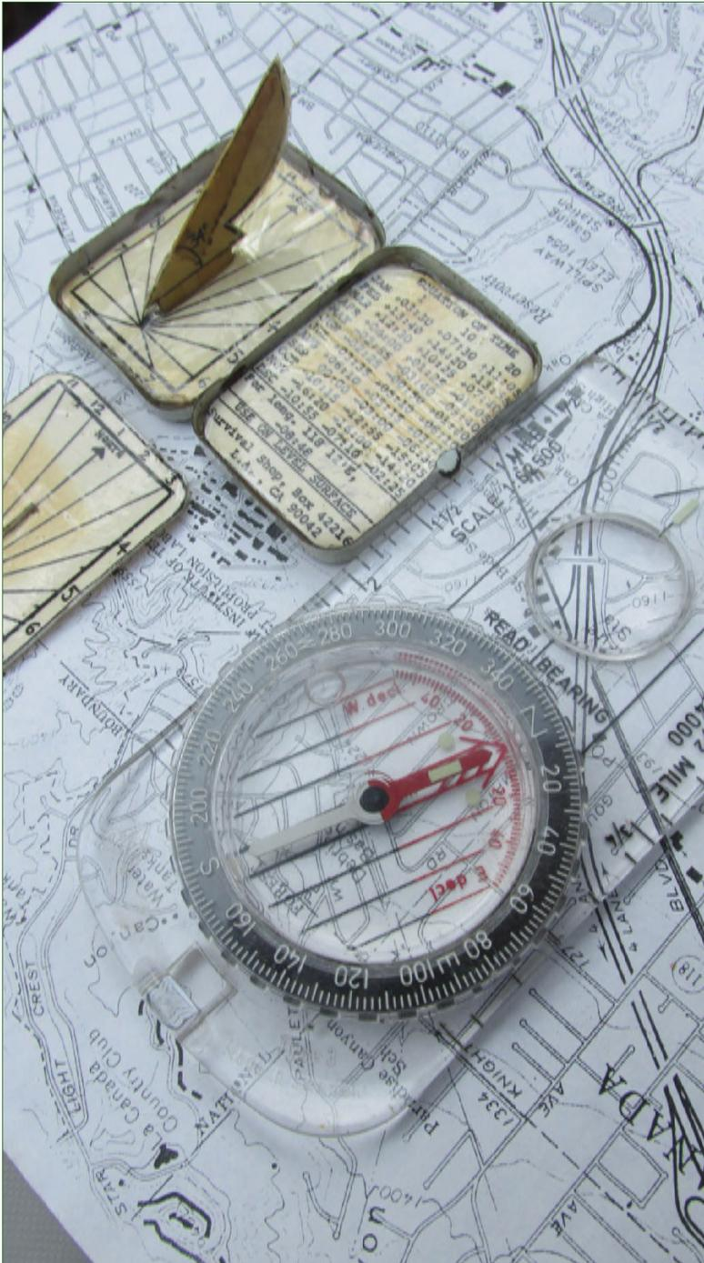
***A simple localized sundial that fits into an aspirin tin is actually accurate when made well and adjusted for location.***
