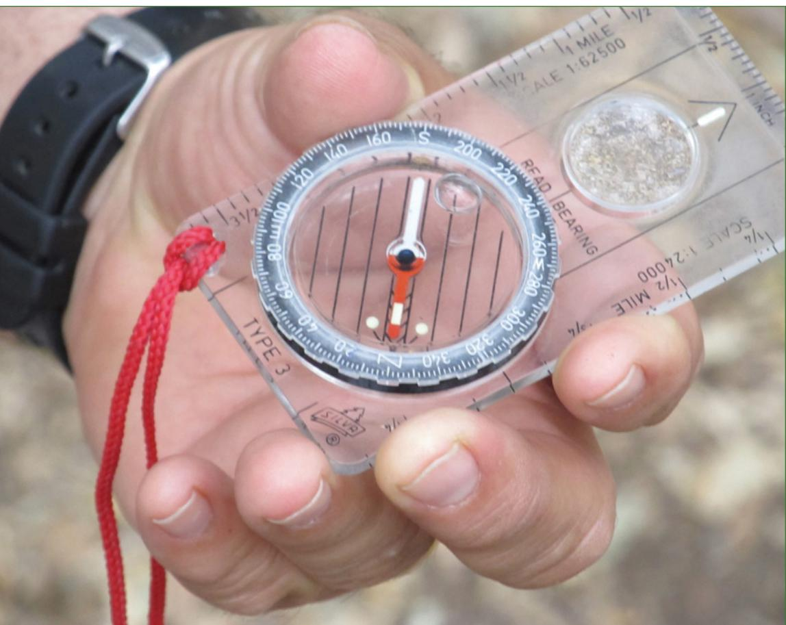
*The dog is in the doghouse. The magnetic needle's north end is within the boundaries of the printed arrow on the movable dial of the compass.*
