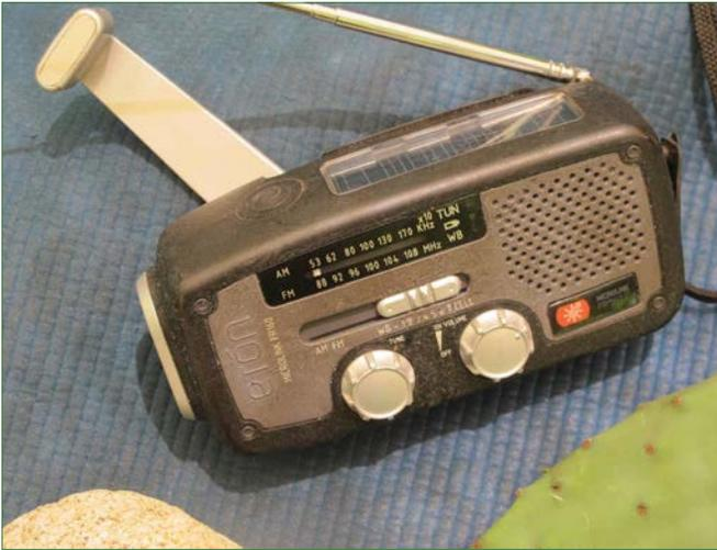
*One example of the hand-crank radios available. This one also has a solar panel.*
