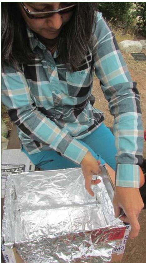
***Line the inside of the smaller box with aluminum foil.***
