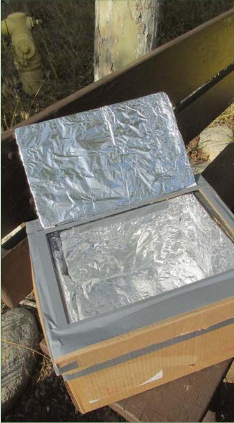
***The finished solar box cooker. The flap covered in aluminum foil can be adjusted to shine more sunlight into the box. When not in use, the flap protects the glass.***
