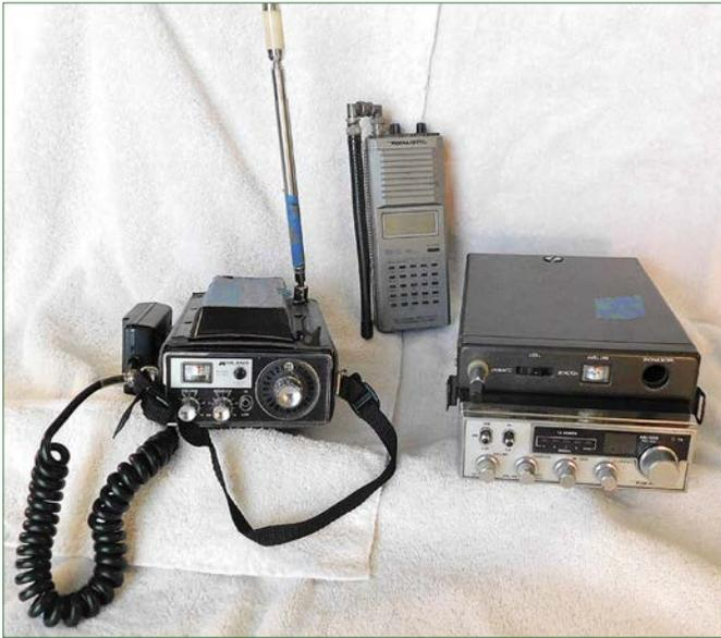
***These old radios are still operational after several decades. Left, is a Midland CB from the '70s. The built-in antenna and battery pack have allowed five mike contacts. Center: a 30-year-old scanner. Right, a Mobil CB with SSB, allowing greater range. Normally mounted in a truck, this one's attached to an old Radio Shack Portable Power Pack. This allowed use on the move or at remote locations.***
