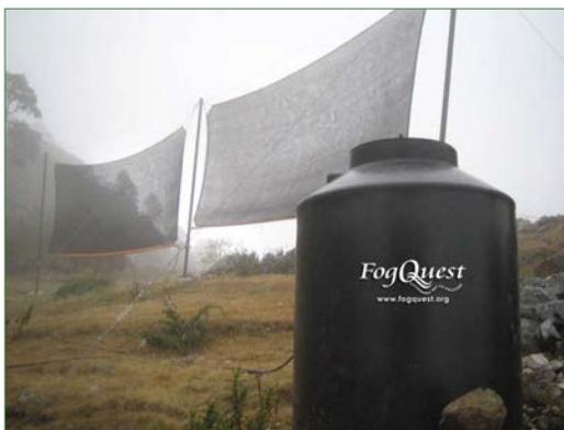
*Dew collects on the unique fabric, and the water drips down a tube and into a collection tank. PHOTO COURTESY OF FOGQUEST.*
