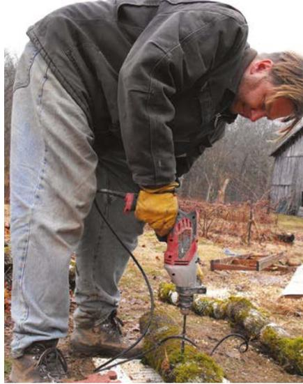
A battery-powered drill allows you to drill your holes out in the woods rather than hauling the logs back to your house to be inoculated. But a corded drill has more power and doesn't need its batteries refreshed at intervals.
