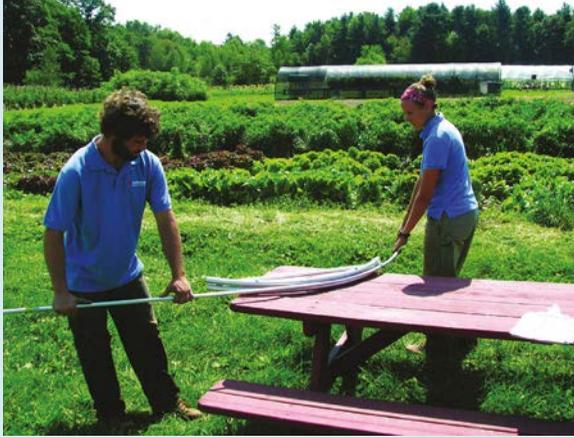
The Quick Hoops™ Bender streamlines the production of metal hoops.
