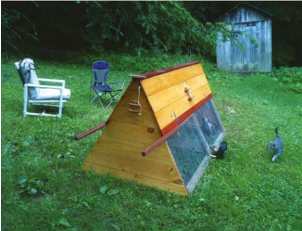
Duncan Sickler's chicken tractor would fit into any neighborhood, no matter how nice. He built his tractor using the Catawba coop plans available online. The tractor is an A-frame structure with an open-bottomed "downstairs" and a wood-floored upstairs. Chickens hang out on the ground but head up a ramp to lay eggs or roost for the night.
