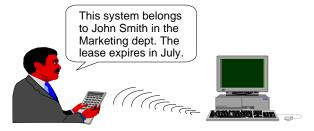
As soon as the systems are unpacked and plugged in, the rest of your job can be completed from a management console using IBM's LANClient Control Manager™ (LCCM) software and Wake on LAN® technology. You can easily program a routine that turns each system on, reads the Asset ID-programmed software requirements, downloads the appropriate operating system image, and then powers the system off.³
