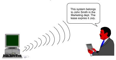
The next time you need to do a physical inventory, you can simply walk around the premises with your handheld reader. This device can read the complete, up-to-date system information through the Asset ID interface. Critical system data such as user ID, lease expiration date and configuration information can be read in seconds. Because the embedded Asset ID tag contains
