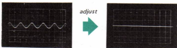
Fig. 3-8. Fm discriminator alignment output response
