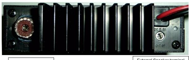
Antenna socket for PL-259 (UHF) External Speaker terminal (3.5 mm mono, 4-8 Ohms)
