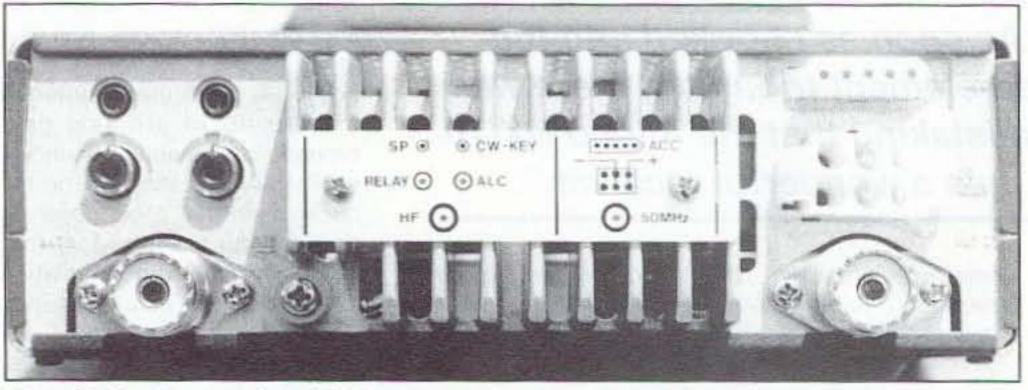
Photo D. On the rear of the DX-70 are two antenna jacks to the left for 3–30 MHz, and to the right for 50–54 MHz. It has the same power plug as all other brands of HF ham sets.
