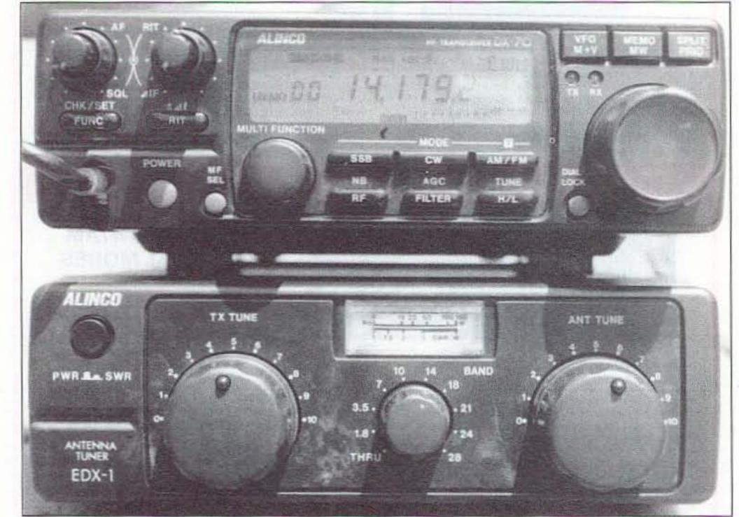
Photo A. The Alinco DX-70 and the matching Alinco Antenna Tuner combine to form a compact "field" radio.
