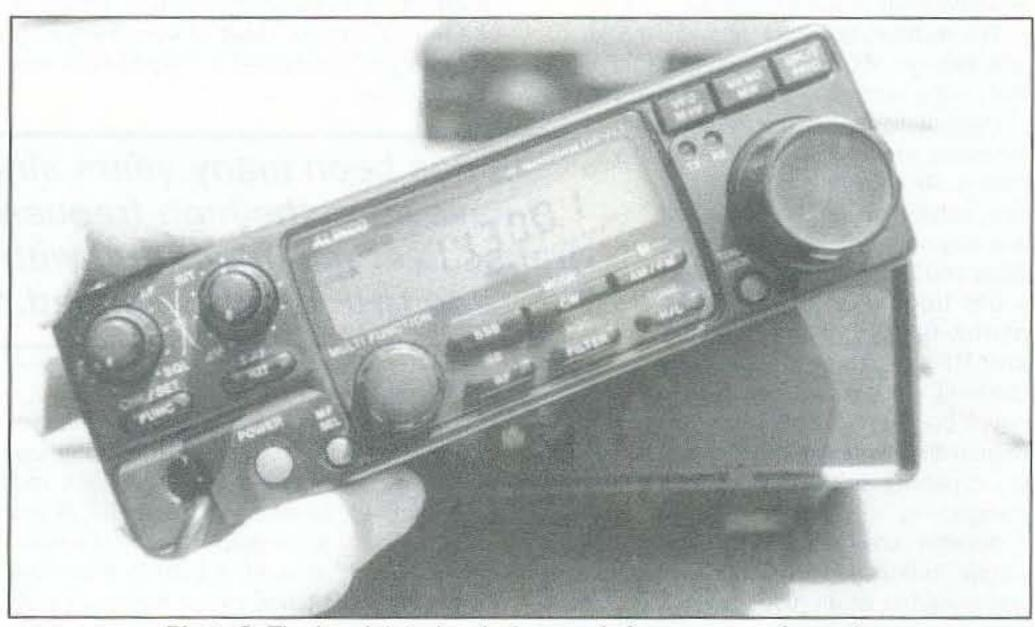
Photo C. The head detaches in 3 seconds for purposes of security.
