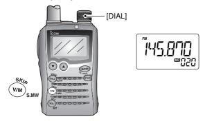
② Push and hold [V/M] (skip-s.mw) for 1 sec. to enter select memory write mode.
