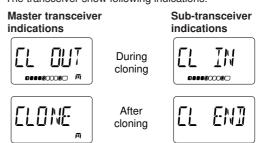
When cloning is finished, turn power OFF, then ON to exit cloning mode.
