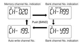
→ After selecting channel number indication as described at left, push [BAND] (τs•Locκ) to select the desired bank. Or while pushing and holding [BAND] (τs•Locκ), rotate [DIAL] to select the desired bank.
