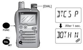
⑤ While pushing and holding **[FUNC]**, rotate **[DIAL]** to select the polarity from "BOTH N" (normal), "TN-RR" (TX: normal, RX: reverse), "TR-RN" (TX: reverse, RX: normal) and "BOTH R" (reverse).
