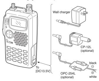
\*To charge the battery pack 13 to 16 V DC is necessary.
