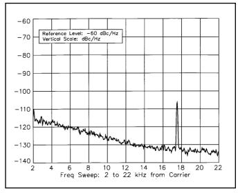
Figure 3—Worst-case tested spectral display of the TS-570D transmitter output during composite-noise testing. Power output is 100 W at 3.5 MHz. The carrier, off the left edge of the plot, is not shown. This plot shows composite transmitted noise 2 to 22 kHz from the carrier.
