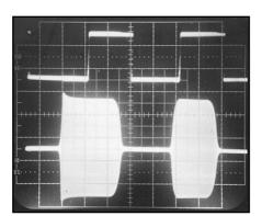
Figure 2—CW keying waveform for the TS-570D showing the first two dits in the full-break-in (QSK) mode. The equivalent keying speed is 60 wpm. The upper trace is the actual key closure; the lower trace is the RF envelope. Horizontal divisions are 10 ms. The transceiver was being operated at 100 W output at 14.2 MHz.
