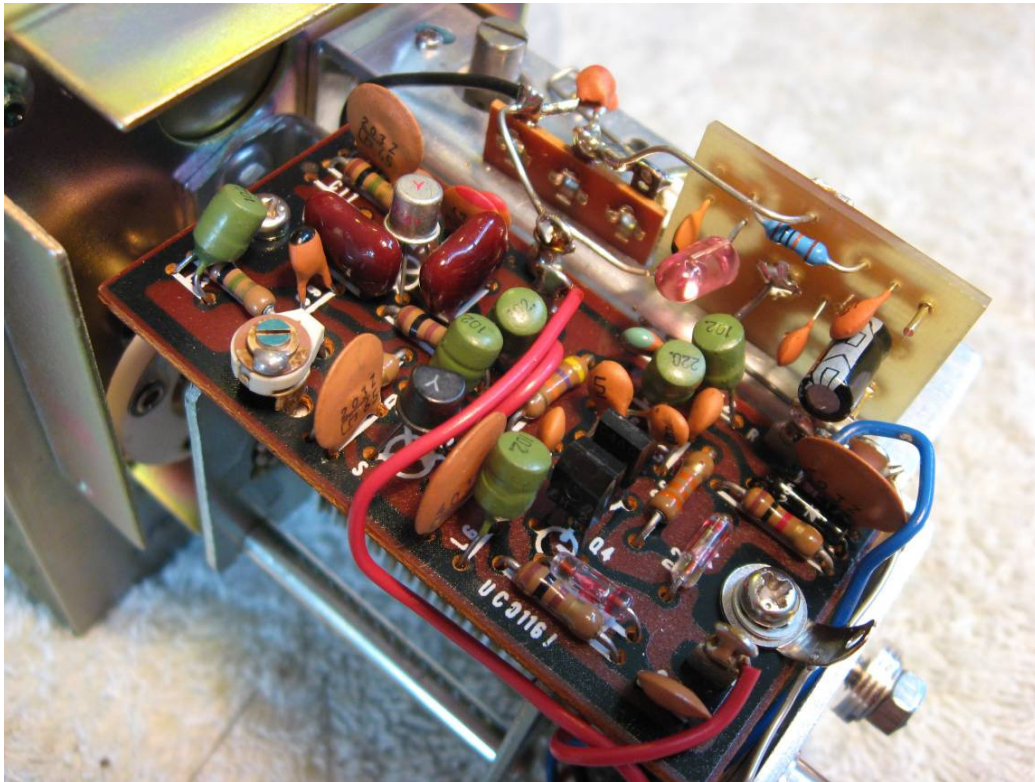
Photo 1 – The Varactor PCB mounted inside the VFO enclosure
