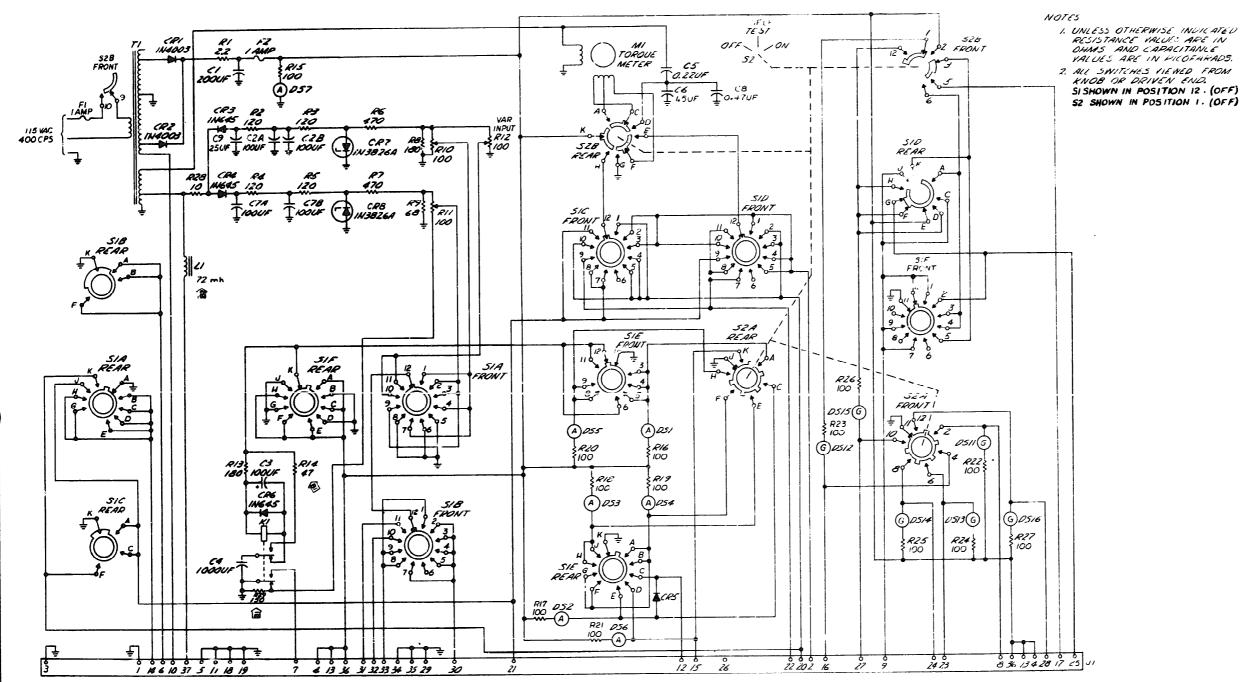
FO-3. 878L-16 Electronic Control Amplifier Tester, Schematic Diagram.
