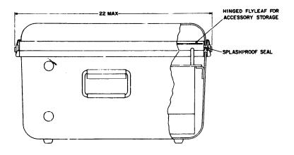
Figure 2-4. 980H-1, Test set, outline and mounting dimensions.
