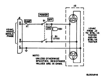
Figure 2-5. Test Set 980H-1 Power Panel, Schematic Diagram.
