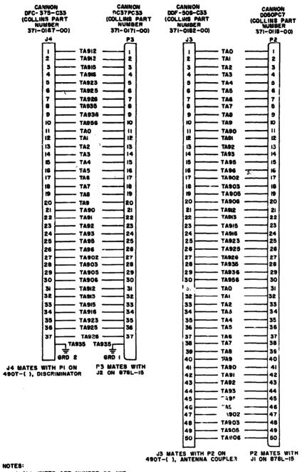
I. ALL WIRES ARE NUMBER 26 AWG. 2. CABLE LENGTH IS 36±1 INCH.
