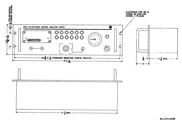
Figure 2-2. TS-2354/ARM-109 Test Set, Electronic Control Amplifier
