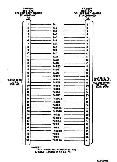
Figure 2-8. 878-16 Special Cable Assembly W3, Schematic Diagram
