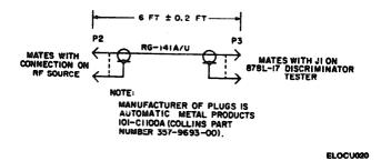
Figure 2-9. 878L-17 Special Cable Assembly W4, Schematic Diagram.
