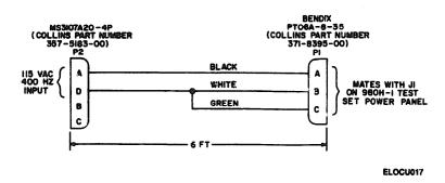
Figure 2-6. Power Panel Special Cable Assembly W1, Schematic Diagram.
