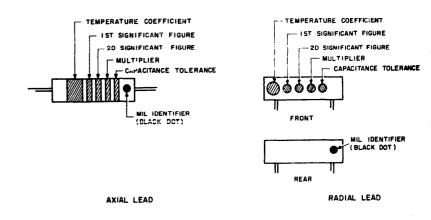
FO-1. Resistor, capacitor, and inductor codes.
