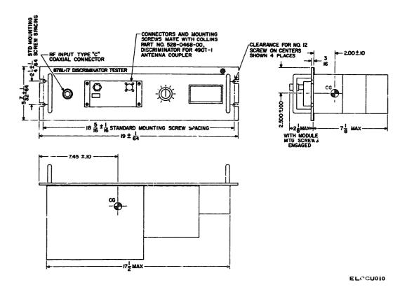
Figure 2-3. 878L-17 Discriminator Tester, outline and movnting dimensions
