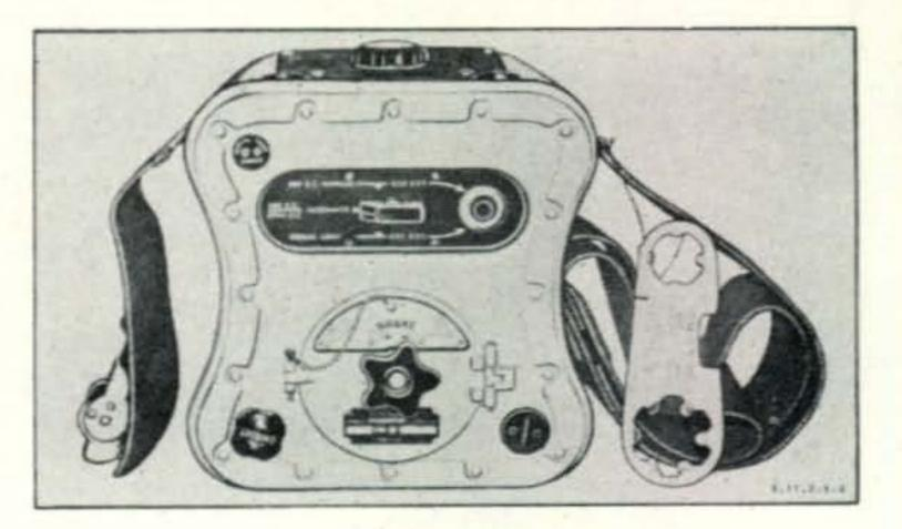
The AN/CRT-3 "Gibson Girl" emergency transmitter. Adapted from the German N.S. 2 "Notsender," in 1941, it gets its name from the curvaceous shape, designed to be easily held
