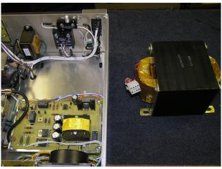
Position the HV transformer with the wires and connector as shown.
