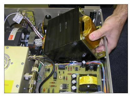
While supporting the raised side of the transformer, gently lower it in place until it, too, is resting on the chassis. The large opening in the side of the chassis allows access to do this.
