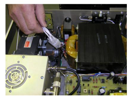
Plug the connector on the transformer into the one on the wiring harness. It is keyed so that it cannot be plugged in backwards. Make sure that the connector halves are pressed together until the lock tabs snap in place.
