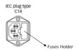
13.5 Power Supply Unit (PSU) protections
