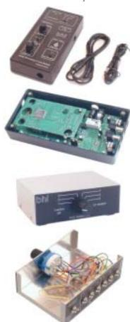
A useful 'extra' was a small, separate line output level control just above the main output level knob. Using this I easily matched it to the input line on my PC's sound card as well as via a *RigBlaster* multimode unit, thus giving me a dual benefit; DSP filtering on both 'listening' audio as well as line-output audio for data decoding. A headphone output socket is also fitted, this usefully disconnecting the output speaker audio but not the output line audio when headphones are connected.
