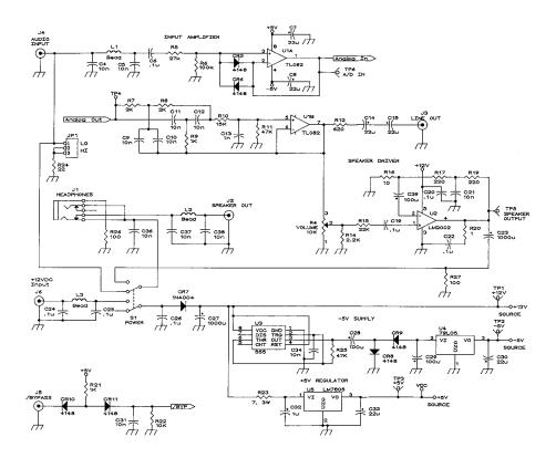
Figure 9 - Audio and Power Supply Section Schematic
