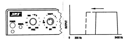
Figure 4 - Low Pass Filter Operation
