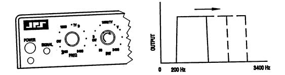
Figure 5 - High Pass Filter Operation
