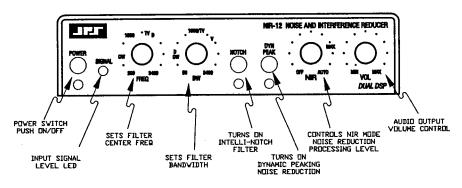
**Figure 1 - Front Panel View**
