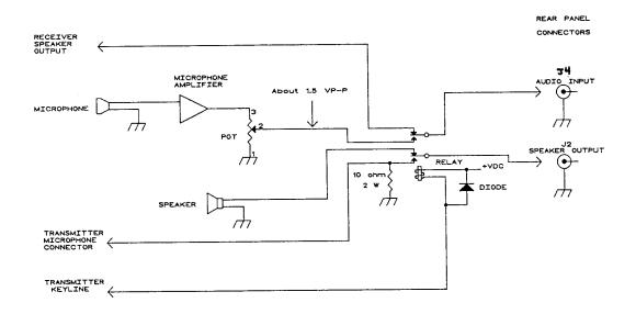
Figure 6 - Connections for Transmit Audio Processing
