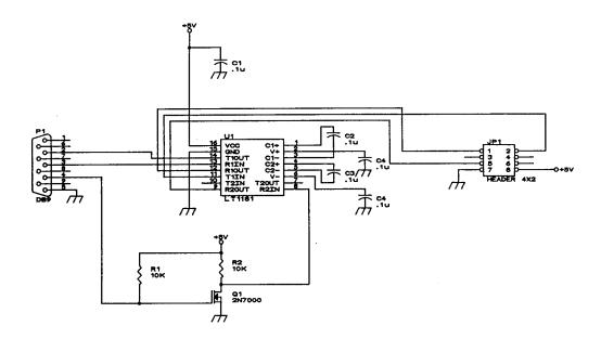
Figure 8 - Level Changer Schematic for RS-232
