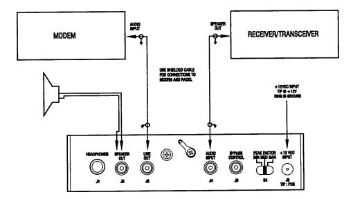
Figure 3 - Connection Diagram
