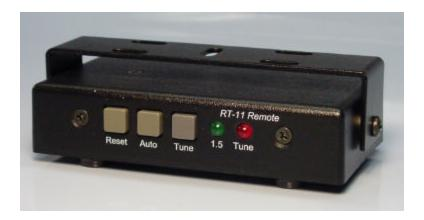
**User-provided control**: You can easily build a custom interface for your particular installation. You can use all, or as little as two control wires to the tuner. For two-wire control, only DC power and ground are required. The tuner will automatically execute a tuning cycle if RF is present at power-up. You can simply insert a momentary open switch at the control location on the +12 DC power line to control the tuner. Cycling power to the tuner with RF present will execute a tuning cycle.
