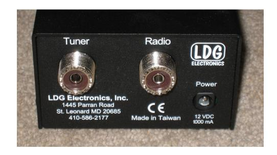
• **Tuner**: connects via coaxial cable to the Radio port on the RT-600.
