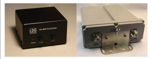
The RC-600 controller has two pushbuttons and one LED indicator light.
