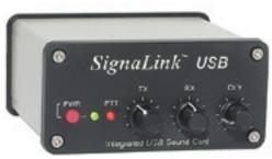
Connecting the SignaLink USB to your radio is relatively easy. You can connect the unit to the transceiver data/auxiliary ports, or to the mike and speaker jacks. (TigerTronics sells pre-made interconnecting cables for a variety of transceivers.) There is a 16-pin DIN socket on the SignaLink for receive audio, transmit audio, PTT and ground connections.
